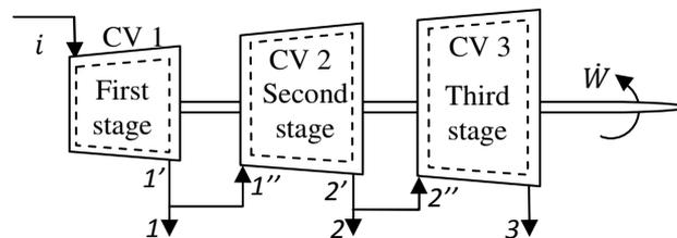
Figure 9. Expansion process in a turbine of multiple (three) stages.
