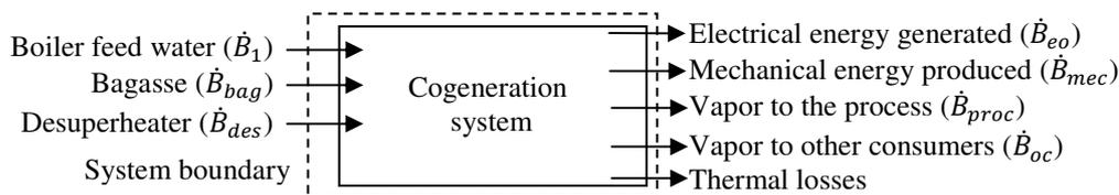
Figure 12. Flowchart of the cogeneration system for the analysis of the exergetic efficiency.
