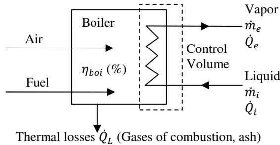
Figure 6. Mass rate balance and energy rate balance of the boiler.
