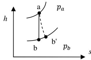
Figure 7. Expansion of the vapor in a single stage turbine (Sears, 1969).
