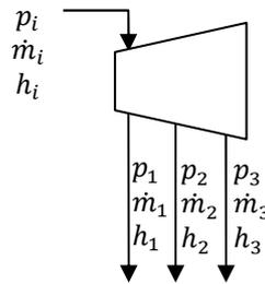
Figure 8. Model of a controlled extraction turbine.
