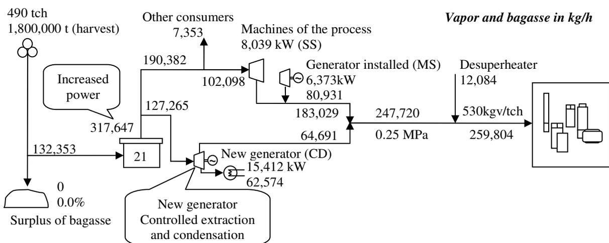
Figure 3. Flowchart of the plant in the Case 2 (Fórum de Co-Geração, 2002).
