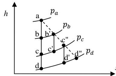
Figure 10. Expansion of the vapor in a multiple stage turbine (Sears, 1969).
