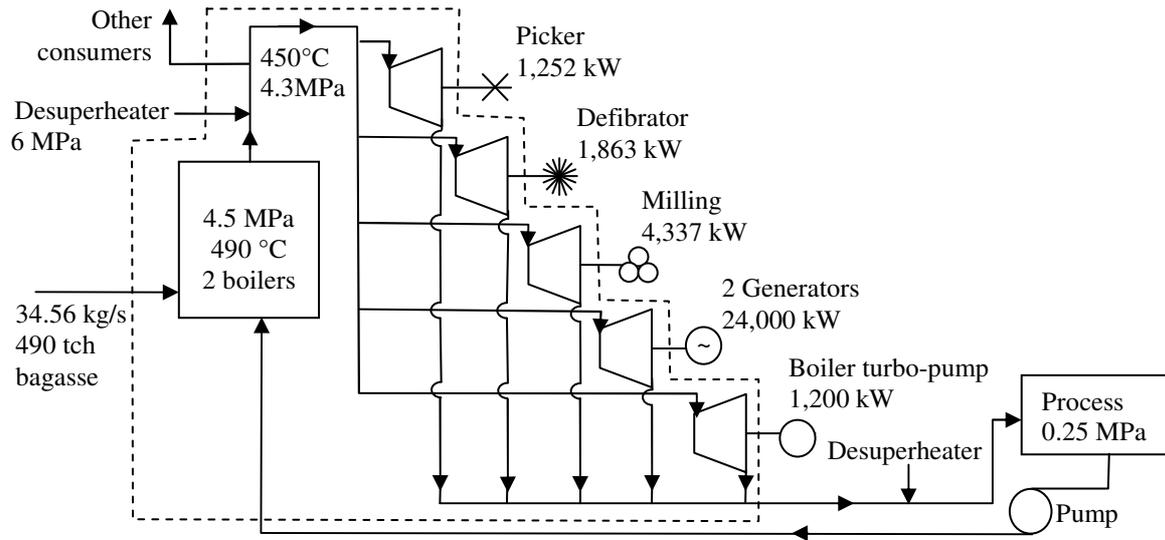
Figure 5. Schematic diagram of Coruripe plant in Campo Florido (courtesy of plant).
