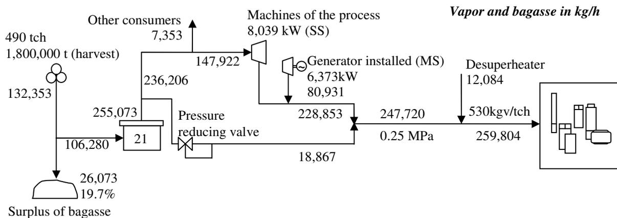
Figure 2. Flowchart of the plant in Case 1 (Fórum de Co-Geração, 2002).
