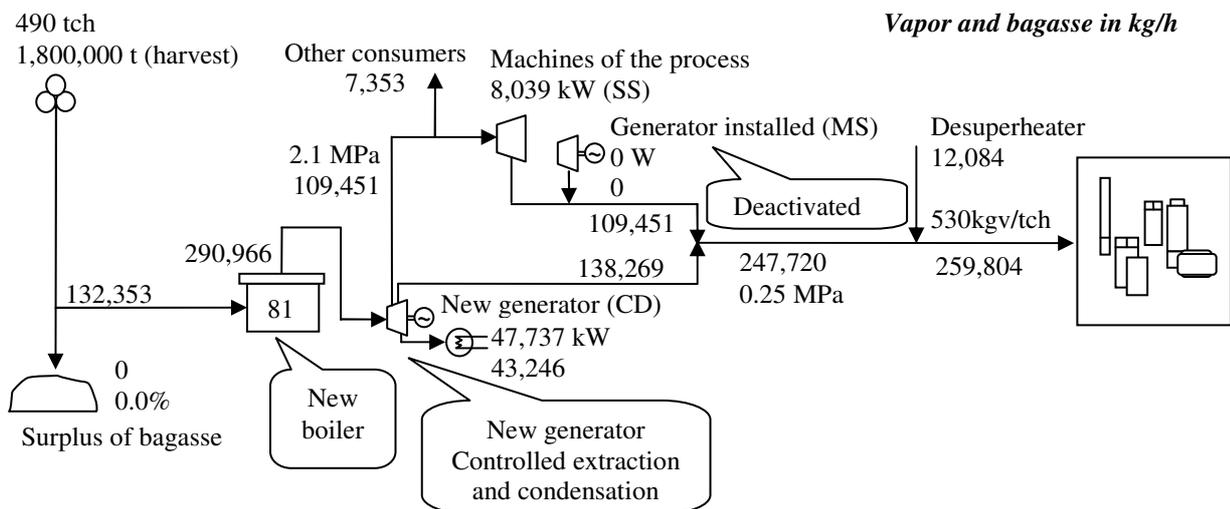
Figure 4. Flowchart of the plant in Case 3 (Fórum de Co-Geração, 2002).
