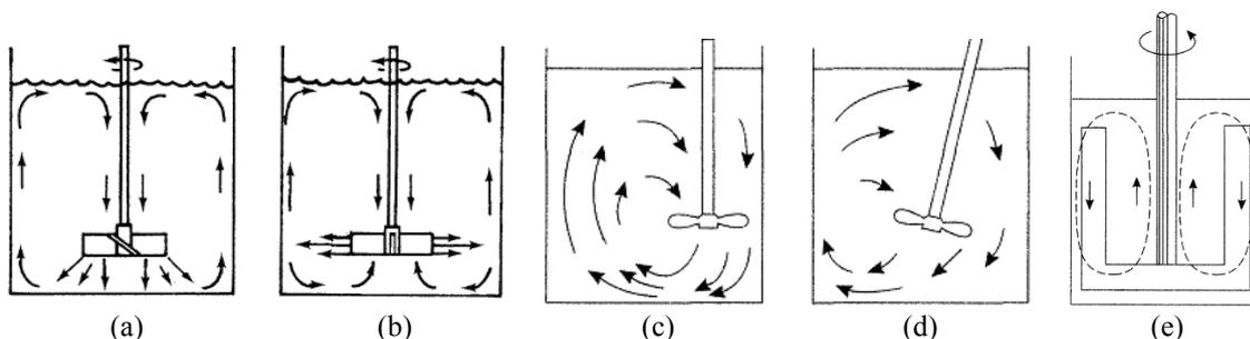
Figure 2 – Liquid flow patterns with a pinned-blade turbine (a) open straight-blade turbine (b) decentralized impeller (c) prone and decentralized impeller (d) and anchor impeller (e).
