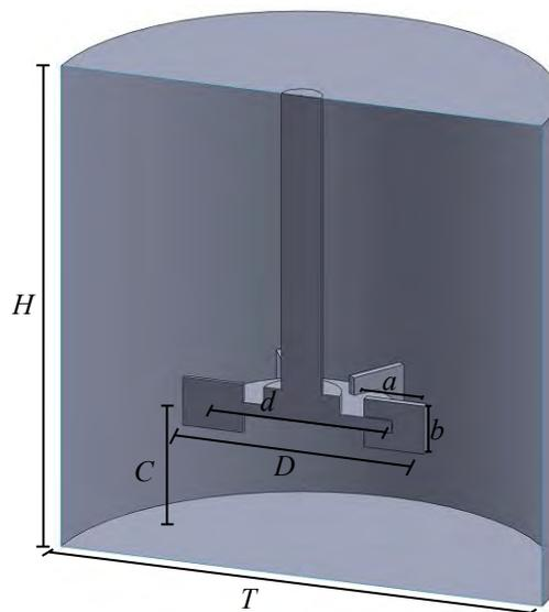
Figure 3. Stirred vessel cross-section view.
