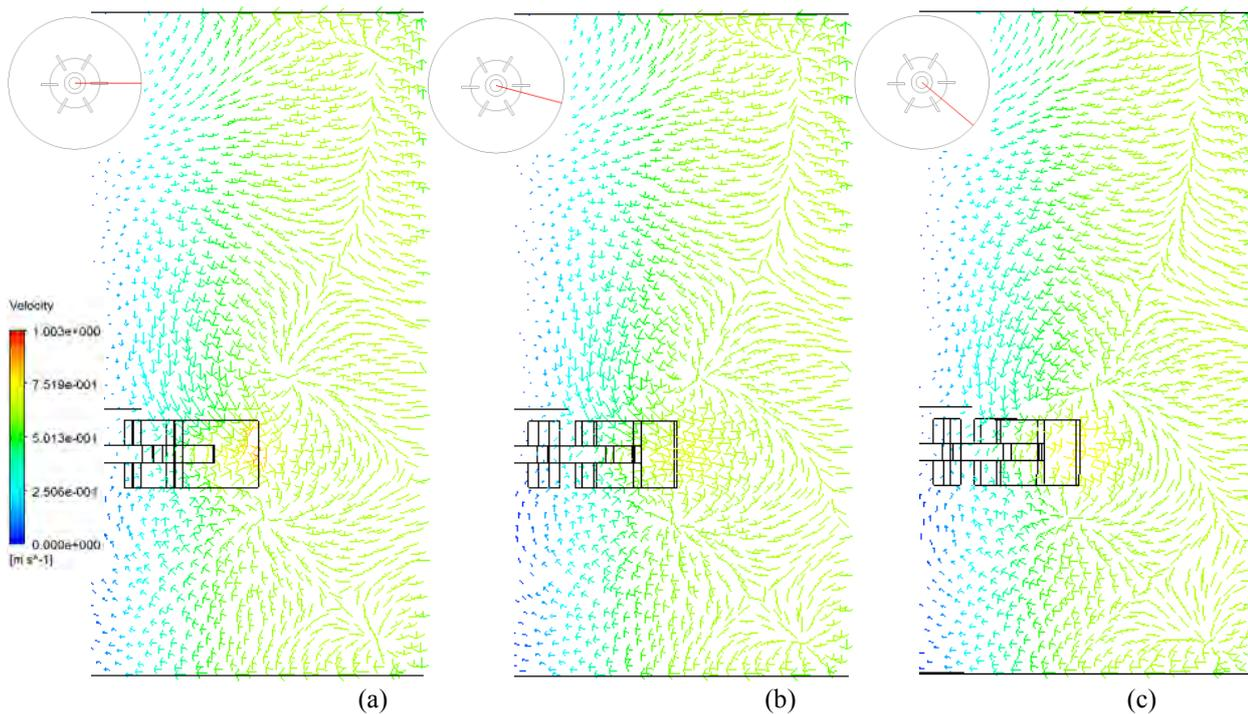
Figure 7. Instantaneous velocity vector plots at three azimuthal locations relative to a blade: (a) plane containing the blade (b)  $15^\circ$  behind the blade (c)  $40^\circ$  behind the blade;
