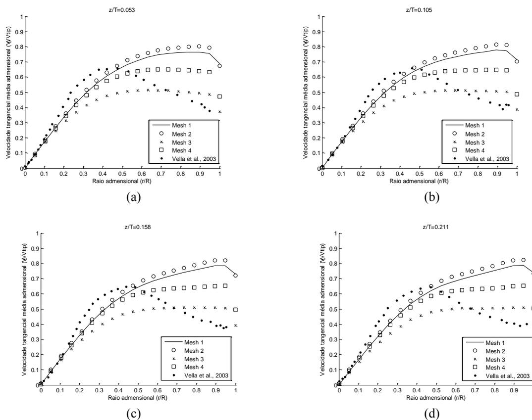
Figure 6. Radial profiles of tangential velocity at different elevations.
