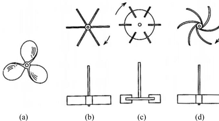
Figure 1 – Top and front view of the most common types of impellers, three-blade marine propeller (a), open straight-blade turbine (b), bladed disk turbine or Rushton Turbine (c), Vertical curved-blade turbine (d).
