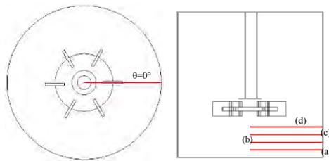
Figure 5. Positions of radial lines of tangential velocity,  $\theta = 0^\circ$  (a)  $z/T = 0.053$ ; (b)  $z/T = 0.105$ ; (c)  $z/T = 0.158$ ; (d)  $z/T = 0.211$
