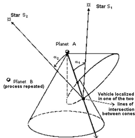
Figure 2 – Geometry of the conventional interplanetary optical navigation. Source: Scull (1966).
