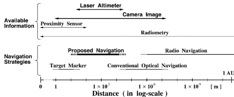
Figure 3 – Available information and navigation strategies. The proposal of Misu *et al.* (1995) for the optical navigation of the Hayabusa spacecraft in the proximity phase with asteroid Itokawa.
