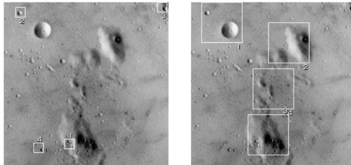
Figure 4 – Images used in the proximity autonomous navigation of the mission Hayabusa (Extraction of templates of different sizes. Left: Extracted areas (16x16). Right: Extracted areas (64x64). Source: Misu et al (1995).
