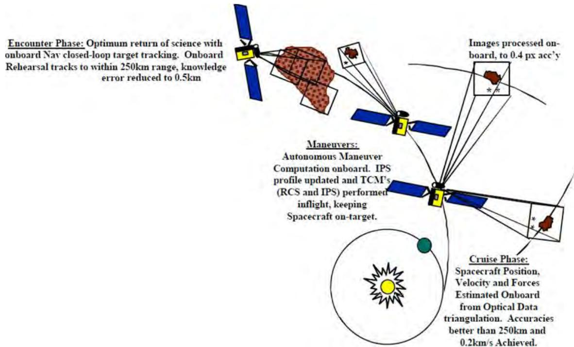
Figure 5 – Autonomous Optical Navigation (AutoNav) for DS-1 mission. Source: Desai et al. (2000), p. vii.
