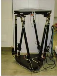
Figure 1. The Stewart platform of the Aerospace Control Laboratory.
