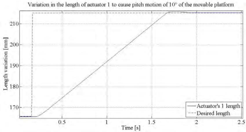
Figure 4. Variation in the length of the actuator 1 to cause pitch motion.
