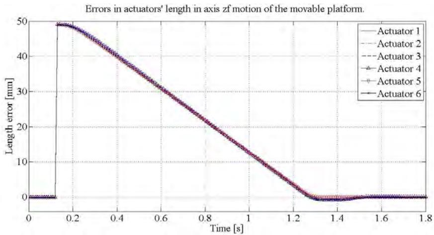
Figure 5. Errors of actuators' lengths during the movement in the axis zf of the movable platform.
