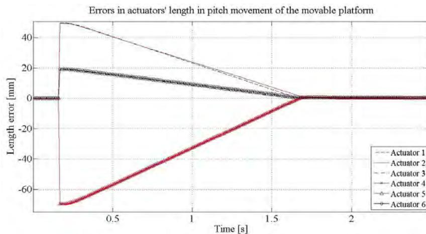
Figure 6. Errors of actuators' lengths during the pitch movement of the movable platform.
