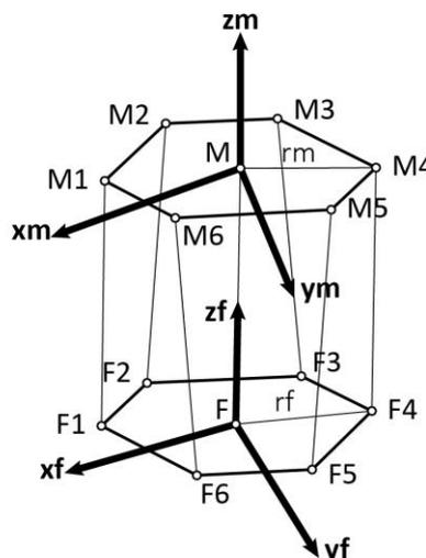
Figure 2. Base and movable platforms coordinate systems.
