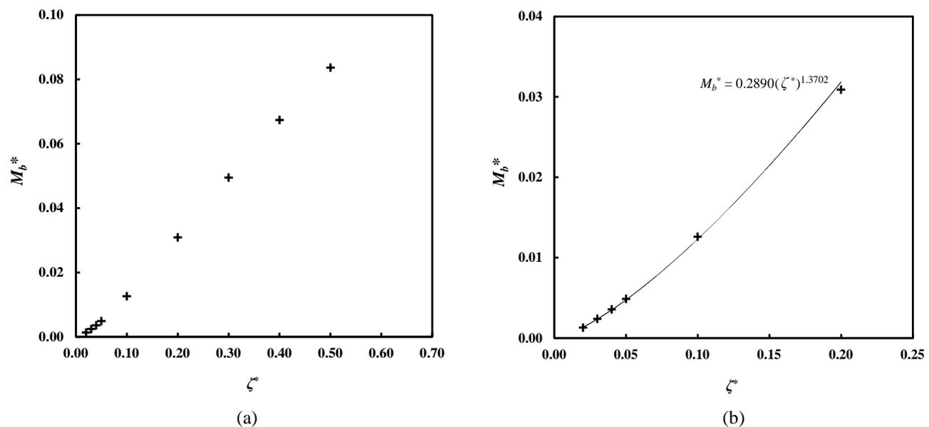
Figure 6. Dimensionless added mass for a prolate ellipsoid ( $b/a = 1/0.6 \cong 1.67$ ) as function of the dimensionless penetration depth,  $\zeta^*$ : (a) full penetration range; (b) small penetration range and power fitting.
