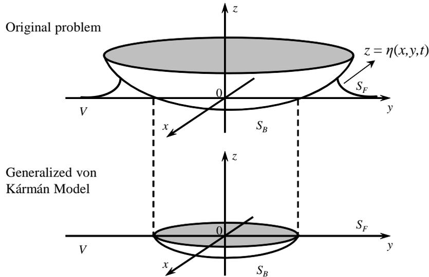
Figure 1. Sketch of the three-dimensional contact area in the Generalized von Kármán Model (GvKM).
