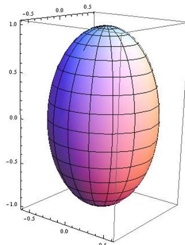
Figure 3. Prolate ellipsoid ( $b/a = 1/0.6 \cong 1.67$ ), being  $a$  the semi-diameter and  $b$  on the axis of revolution  $z$ .
