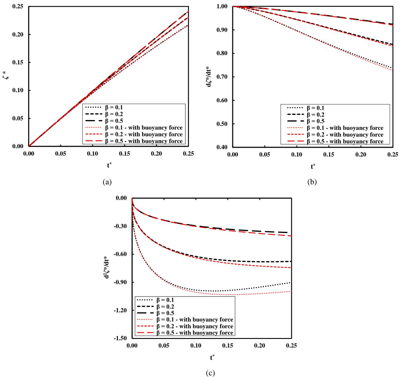
Figure 9. Dimensionless penetration, velocity and acceleration of an impacting prolate ellipsoid ( $b/a = 1/0.6 \cong 1.67$ ) vs. dimensionless time, for three values of specific mass. Equation of motion with and without buoyancy force; Eqs. (13) and (12), respectively.
