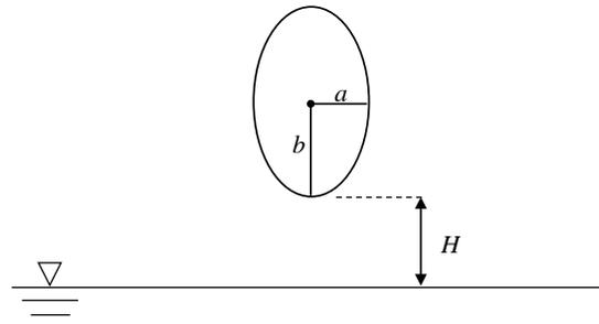
Figure 8. The prolate ellipsoid dropped from the rest.
