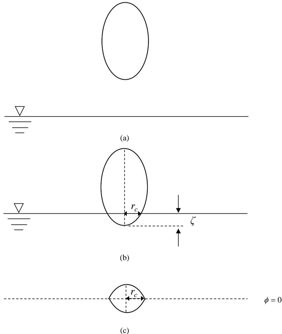
Figure 2. Sketch of the computational strategy: (a) before impact; (b) body impacting the water surface; (c) double body, which is symmetric to the plane  $z = 0$ .
