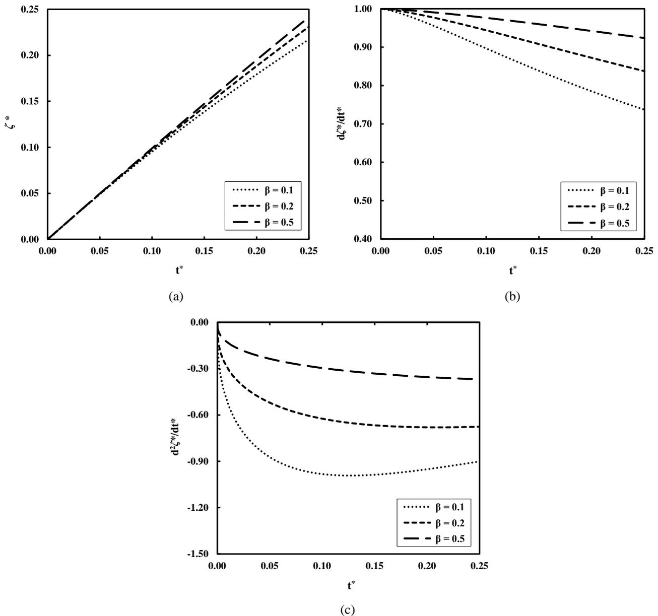
Figure 7. Dimensionless penetration, velocity and acceleration for an impacting prolate ellipsoid ( $b/a = 1/0.6 \cong 1.67$ ) vs. dimensionless time, for three values of specific mass. Equation of motion without buoyancy force, Eq. (12).
