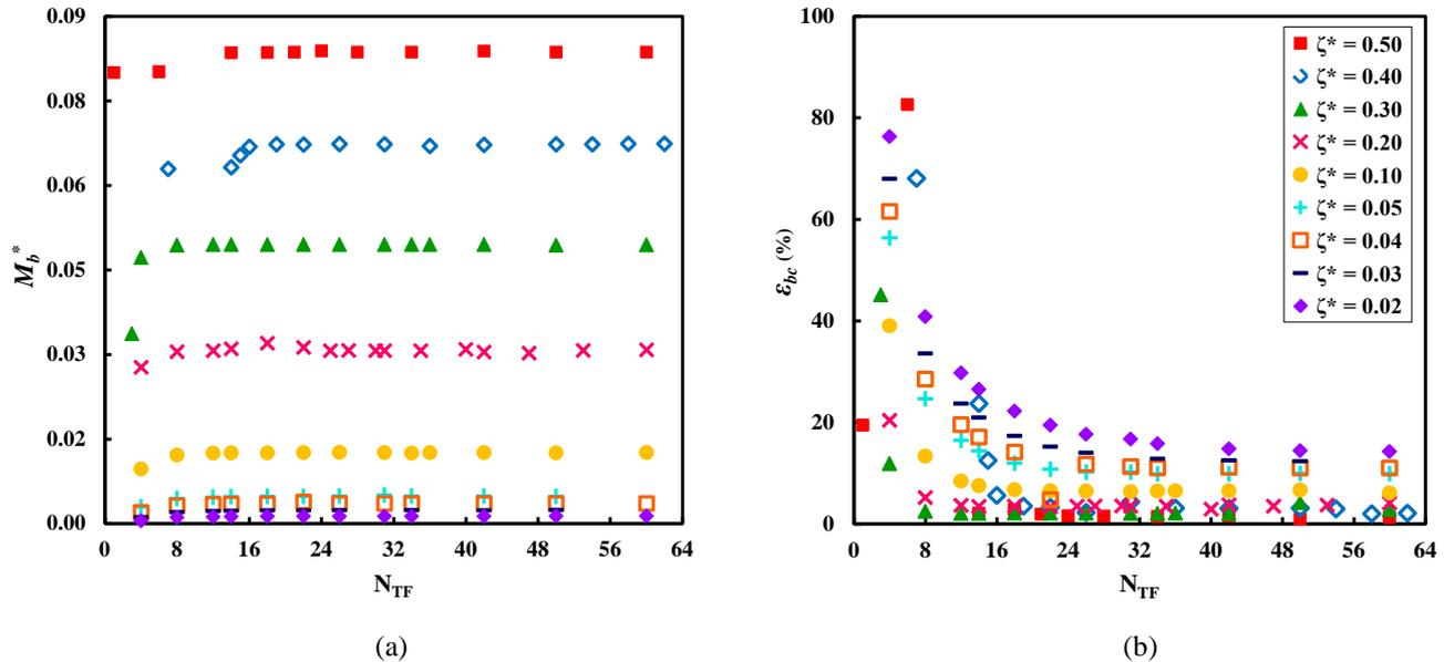
Figure 5. Numerical results and convergence study for a prolate ellipsoid ( $b/a = 1/0.6 \cong 1.67$ ), as function of  $N_{TF}$  (the number of trial functions) (a) dimensionless added mass; (b) weak solution boundary condition error. The legend in (b) is also used in figure (a).
