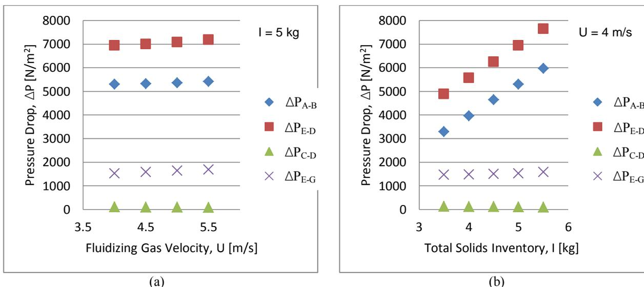
Figure 3 - Pressure drop in the fluidization loop. (a) Variation with the fluidizing gas velocity; (b) Variation with the total solids inventory.
