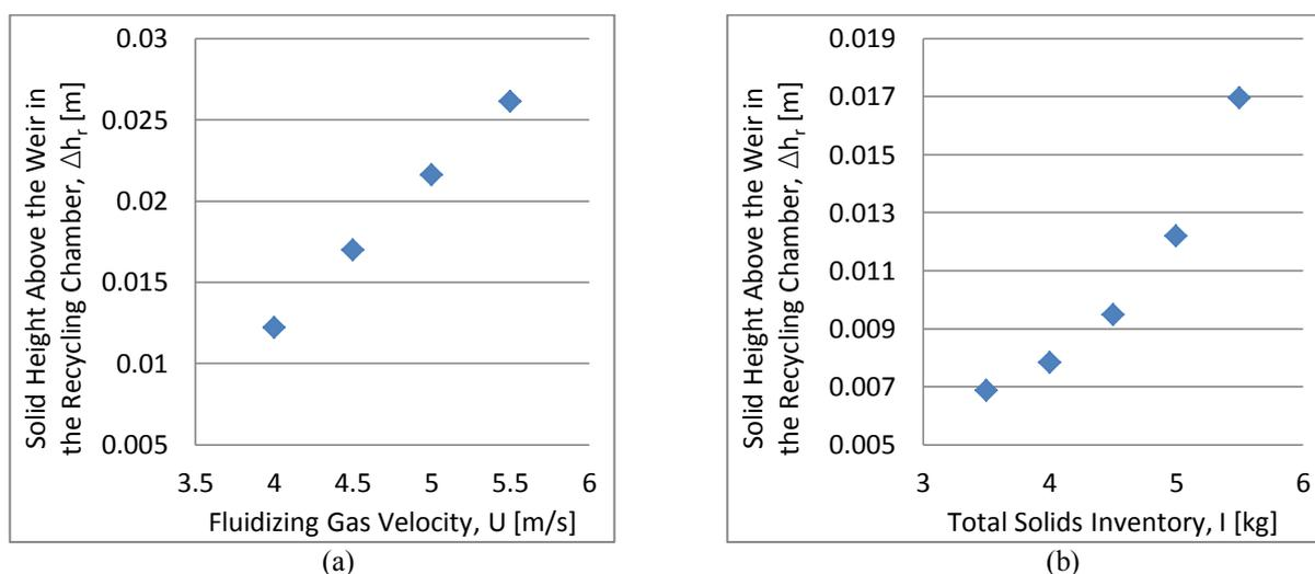
Figure 5 – Solid height above the weir in the recycle chamber,  $\Delta h_r$ :(a) with the varying the fluidizing velocity; (b) with the variation of the inventory of solids.
