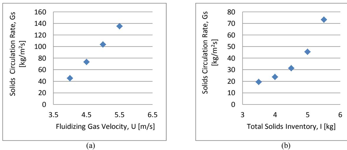
Figure 4 – Solids circulation rate behavior,  $G_s$ :(a) Variation of the fluidizing velocity; (b) Variation of the solids inventory.
