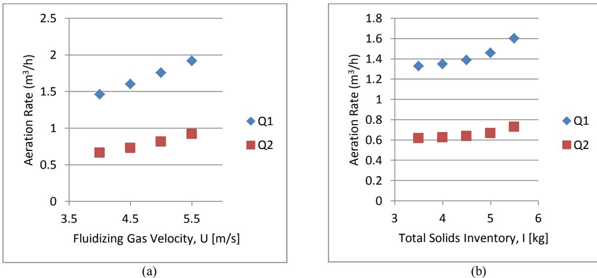
Figure 6 – Aeration rate in the supply chamber ( $Q_1$ ) and in the recycle chamber ( $Q_2$ ). (a) Variation of the fluidizing gas velocity; (b) Variation of the total solids inventory.
