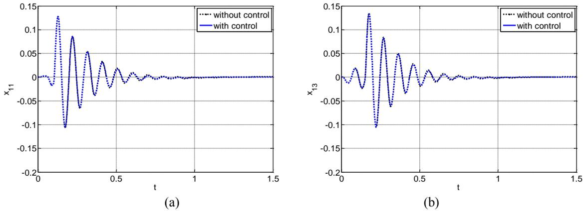
Figure 7. Displacement of the rear unsprung masses. (a) Left. (b) Right.
