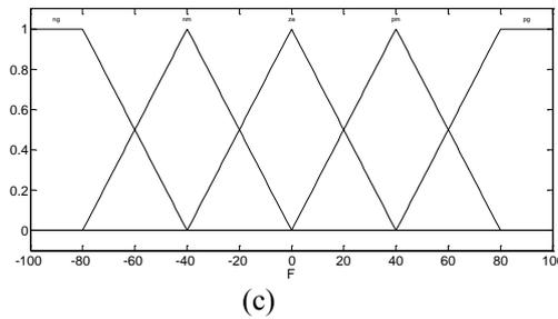
Figure 4. (a) Input membership function (Velocity). (b) Input membership function (Relative Velocity). (c) Output membership function (Force).
