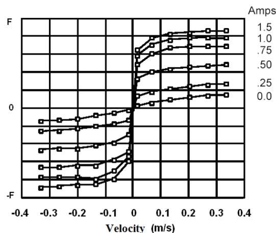
Figure 2. Force–velocity characteristics of a MR fluid damper as a function of the coil current.
