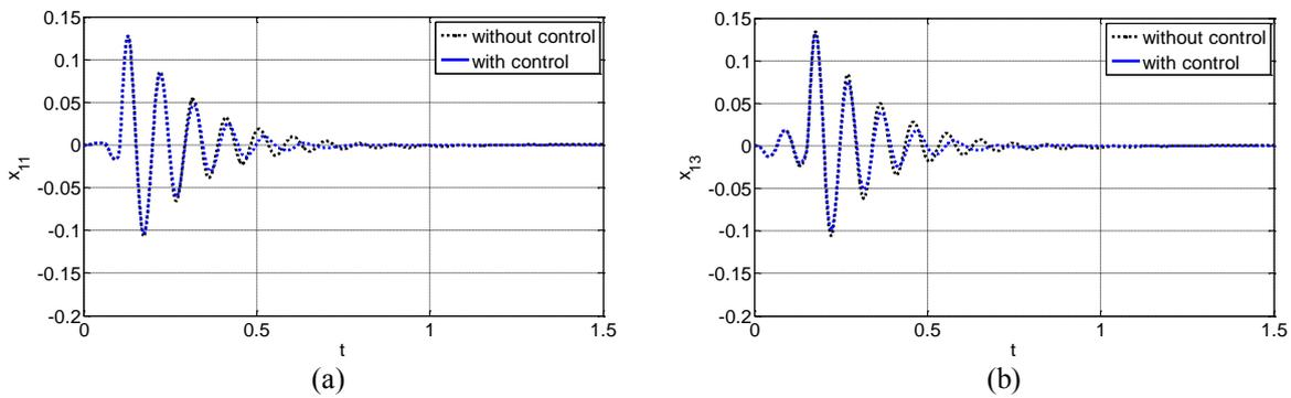
Figure 13. Displacement of the rear unsprung masses. (a) Left. (b) Right.
