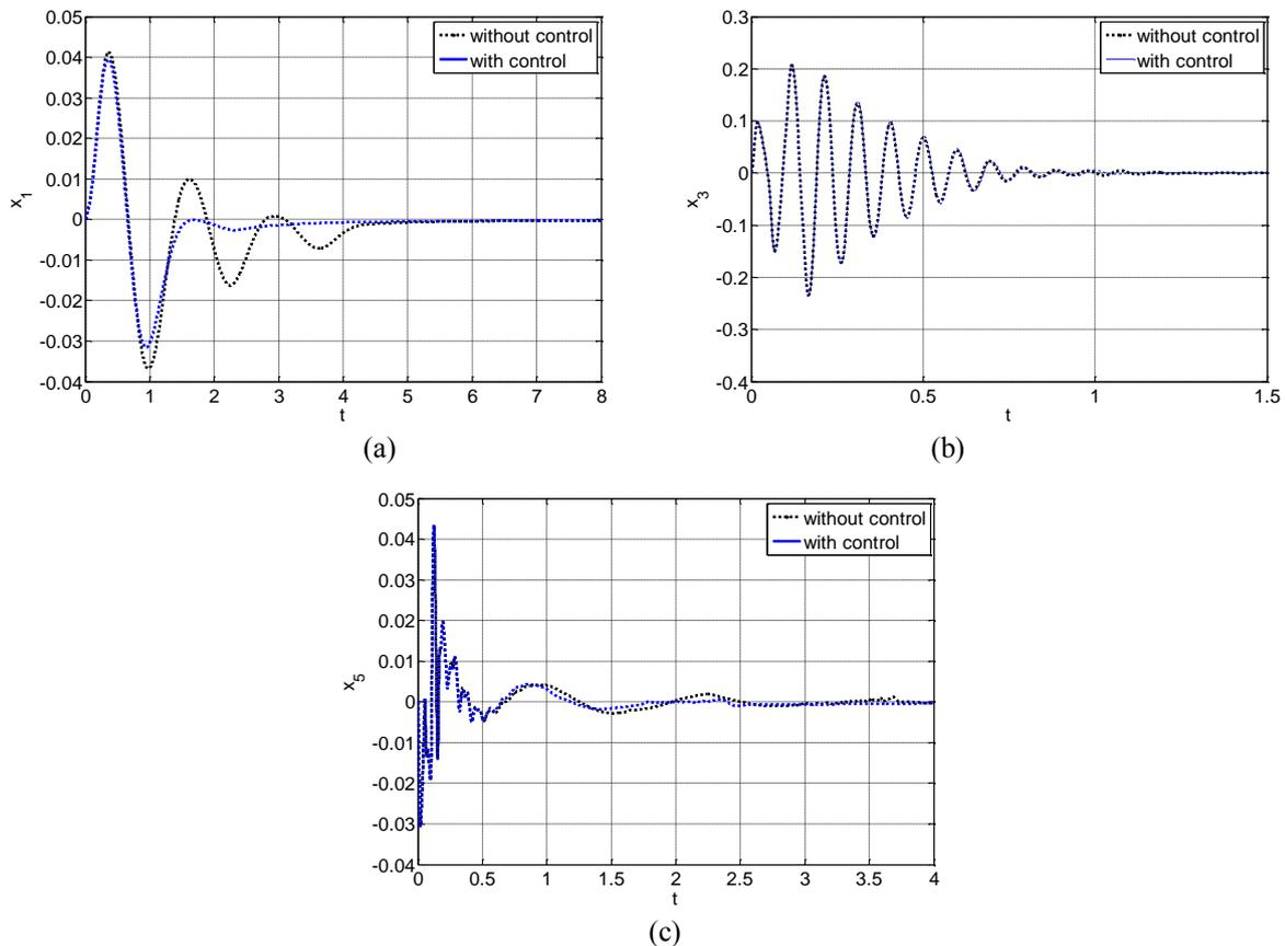
Figure 5. Sprung mass: (a) Vertical displacement. (b) Pitching movement. (c) Roll movement.
