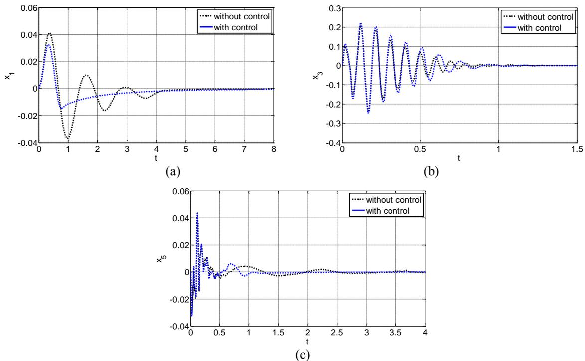
Figure 11. Sprung mass: (a) Vertical displacement. (b) Pitching movement. (c) Roll movement.
