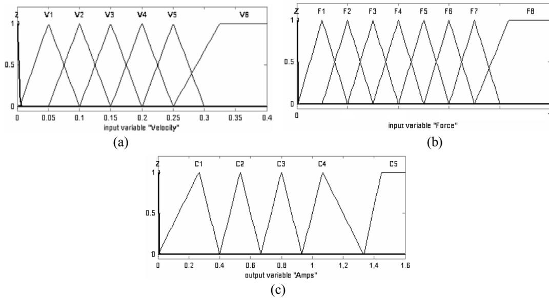
Figure 3. (a) Input membership function (Velocity). (b) Input membership function (Force). (c) Output membership function (Amps).
