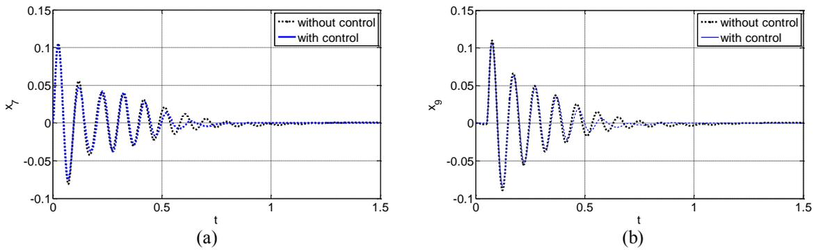
Figure 12. Displacement of the front unsprung masses. (a) Left. (b) Right.
