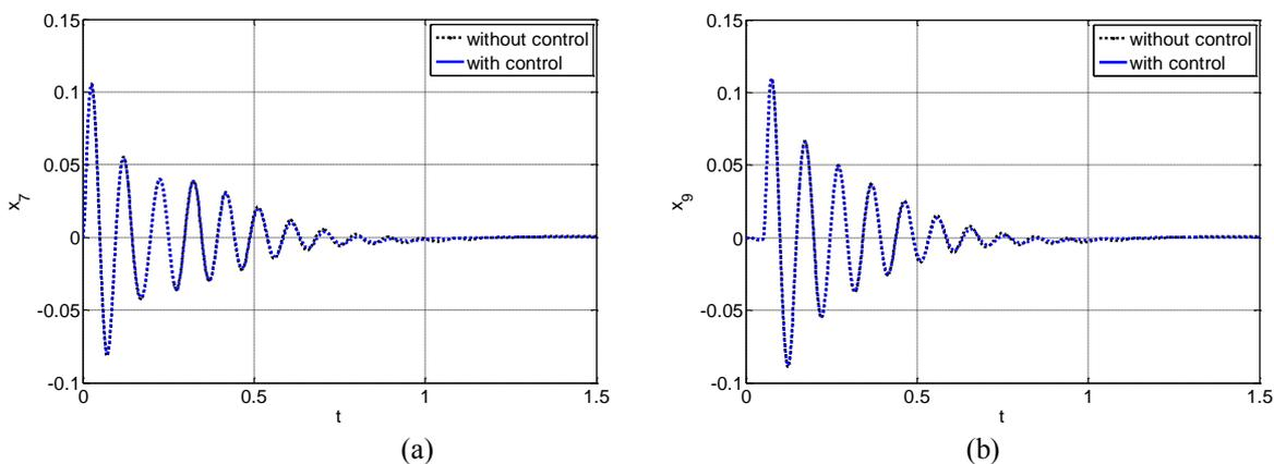
Figure 6. Displacement of the front unsprung masses. (a) Left. (b) Right.
