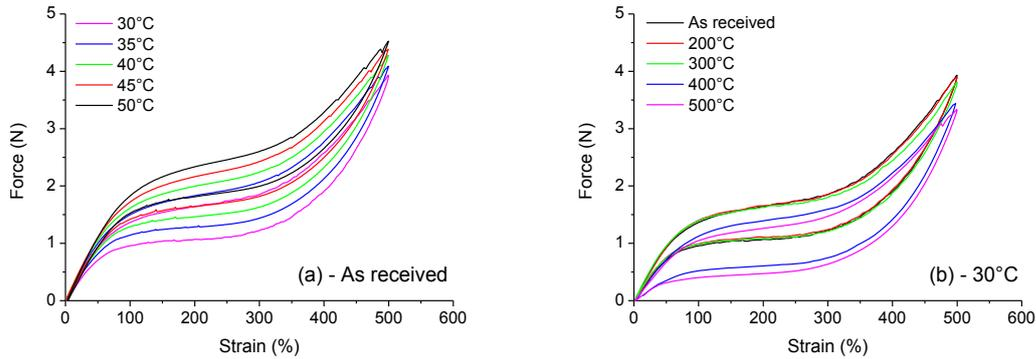
Figure 3. Superelastic behavior of the M7 mini spring sample in function of temperature and annealing temperature (continues).
