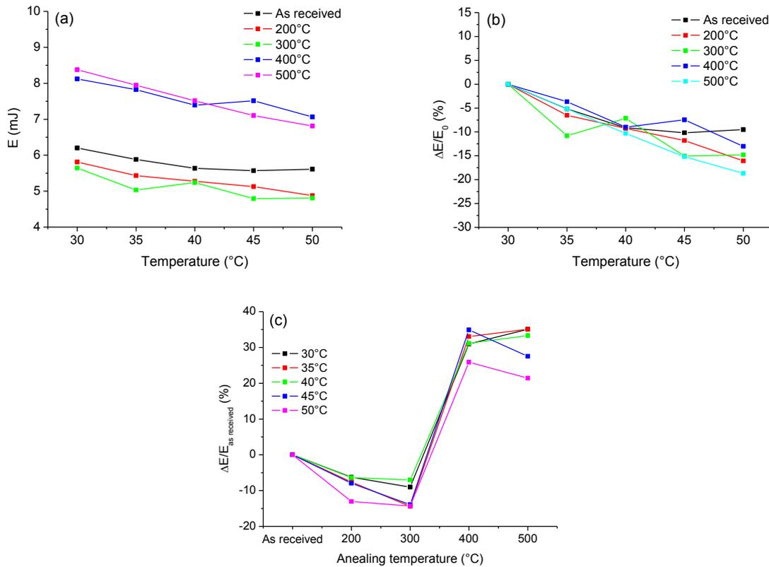
Figure 5. Energy dissipation capacity of M7 NiTi mini spring in function of test temperature and annealing temperature. (a) Absolute values. (b) Percentage variation related to the first value (at 30°C). (c) Percentage variation related to the E value of the *as received* sample.
