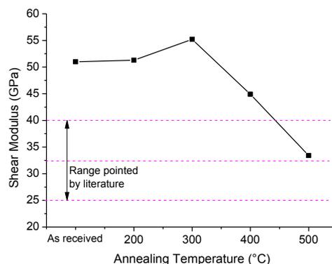
Figure 6. Shear modulus values (at 30°C) in function of annealing temperature.
