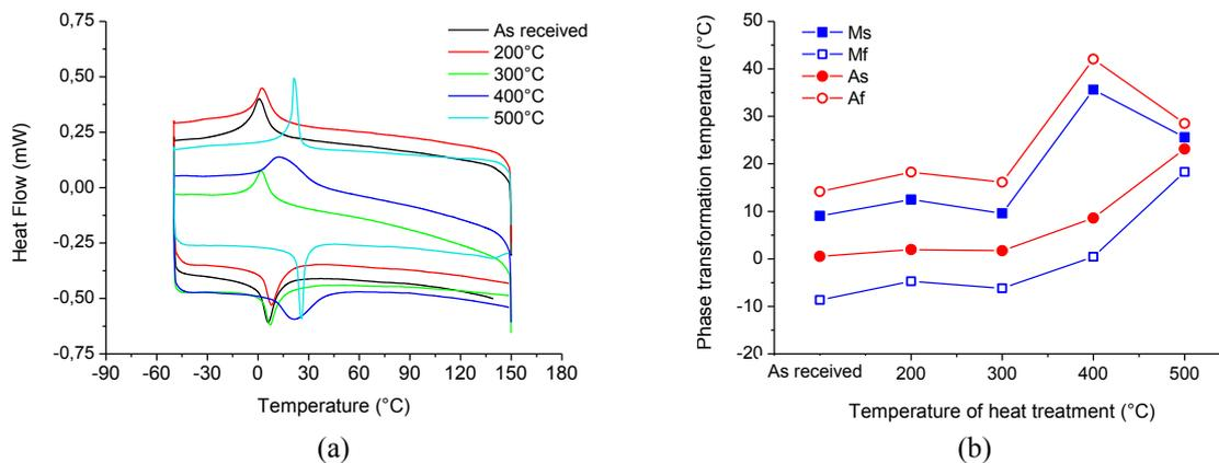
Figure 7. Thermal behavior of the NiTi SMA mini springs. (a) DSC curves for the spring sample treated at different annealing temperatures. (b) Phase transformation temperature ( $M_s$ ,  $M_f$ ,  $A_s$  and  $A_f$ ) obtained from DSC curves.
