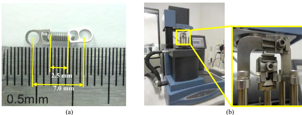
Figure 1. NiTi mini coil spring. (a) M7 mini coil spring with 2.5 mm of deformable length. (b) M7 mounted on uniaxial tensile clamp of DMA Q800, from TA Instruments.
