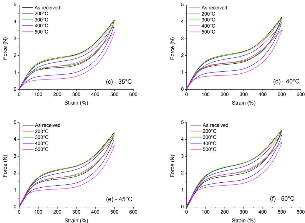
Figure 3. Superelastic behavior of the M7 NiTi mini spring in function of temperature and annealing temperature.
