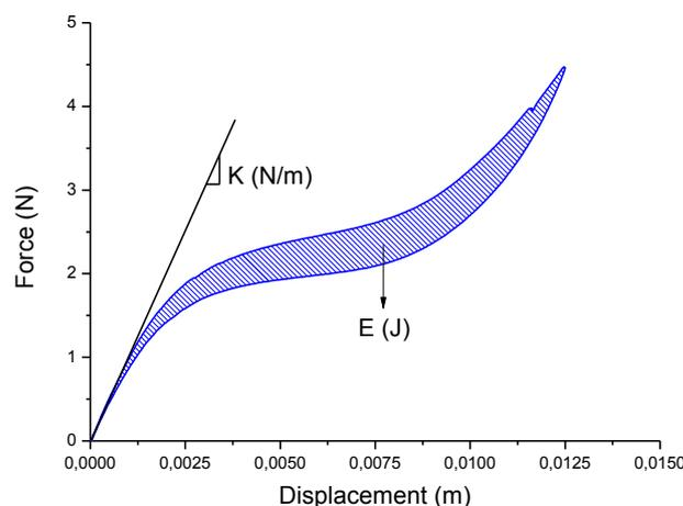
Figure 2. Scheme of a superelastic curve of the NiTi SMA mini spring showing the methodology to calculate stiffness of austenitic phase ( $K$ ) and energy dissipation capacity ( $E$ ).
