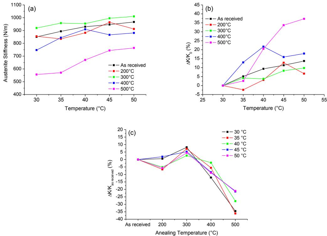
Figure 4. Stiffness behavior of M7 NiTi mini spring in function of test temperature and annealing temperature. (a) Absolute values. (b) Percentage variation related to the first value (at 30°C). (c) Percentage variation related to the stiffness value of the *as received* sample.
