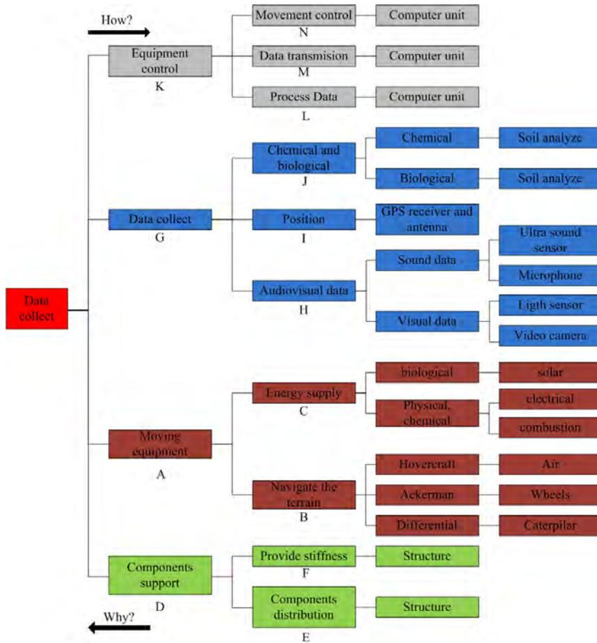
Figure 8. FAST to "data collection" function.
