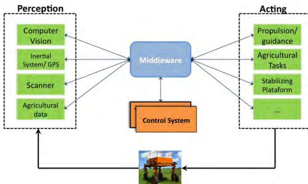
Figure 2. Integration of robotic architecture systems using middleware.
