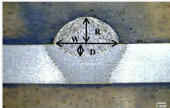
Figure 12 - Cross section of a weld bead simple deposition on the plate using AC MIG / MAG process, the Approach A; ( $EN = 50\%$ ;  $I_p = 250A$ ;  $I_b = 40A$ ;  $I_n = 126A$ ;  $t_p = 5,9$  ms;  $t_{b1} = 2,7$  ms;  $t_{b2} = 1$  ms;  $t_n = 2,73$  ms;  $T = 19,26$  ms;  $W = 6,8$  mm;  $D = 1,3$  mm;  $R = 3,4$  mm.)
