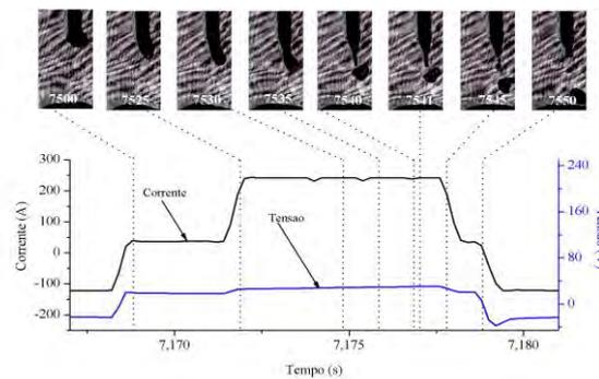
Figure 6 – Graphic of metal transfer AC MIG/MAG process, showing a parameter regulation that produces "ODPP the end of the pulse"; (50%EN:  $I_m^+ = 165A$ ;  $I_p = 250A$ ;  $I_{b1}=I_{b2}=40 A$ ;  $t_p=5,2ms$ ;  $t_{b1}=2,73ms$ ;  $t_{b2}=1ms$ ;  $F_s=5,0m/min$ ;  $I_n=126A$ ;  $t_n=9,6ms$ ;  $I_{(mg)}=147A$ ;  $T=22,8ms$ ;  $CTWD=25mm$
