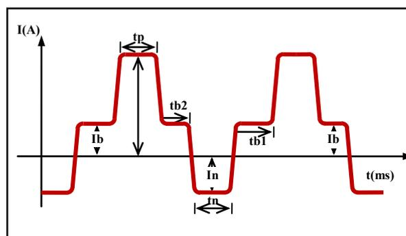
Figure 1 - Waveform (base-pulse-base)  $I_p$ = Peak current;  $I_{b1}$ = Background current before of detachment;  $t_{b1}$ = Background time before the peak detachment;  $I_{b2}$ = Background current after peak of detachment;  $t_{b2}$ = Background time after the peak detachment;  $I_n$ = Negative current in the;  $t_n$ = Negative Time.
