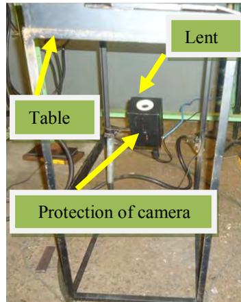
Figure 10 - Infrared Camera FLIR A325 series in its enclosure positioned to shoot infrared
