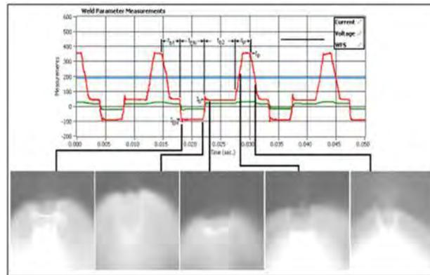
Figure 1 - Typical Waveform CA MIG / MAG and its correlation with the stages of growth and detachment of the drop (Harwig adapted from 2006)
