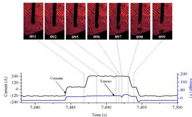
Figure 7 – Graphic of metal transfer AC MIG/MAG process, showing a parameter regulation that produces "ODPP the end of the pulse". Approach A com 50%EN:  $I_m^+ = 165A$ ;  $I_p = 250A$ ;  $I_{b1}=I_{b2}=40A$ ;  $t_p=5,9ms$ ;  $t_{b1}=4,5ms$ ;  $t_{b2}=1ms$ ;  $F_s = 4,7m/min$ ;  $I_n=126A$ ;  $t_n=7,6ms$ ;  $I_{(mg)}=147A$ ;  $T=19ms$ ;  $CTWD = 25mm$
