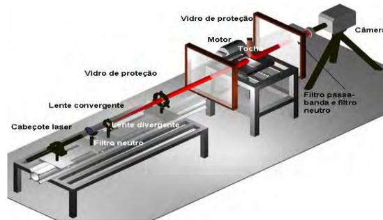
Figure 5 - Arrangement drawing of the equipment for filming, especially the high-speed camera(Balsamo et al 2000) and table displacement of the specimen
