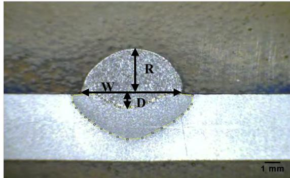
Figure 13 - Cross section of a weld bead simple deposition on the plate using AC MIG / MAG process, the Approach B; ( $EN = 50\%$ ;  $I_p = 250A$ ;  $I_b = 40A$ ;  $I_n = 126A$ ;  $t_p = 5,9$  ms;  $t_{b1} = 2.60$  ms;  $t_{b2} = 1$  ms;  $t_{EN} = 9.50$  ms;  $T=19$  ms;  $W=6.56$  mm;  $D=0.94$  mm;  $R=3.30$  mm)
