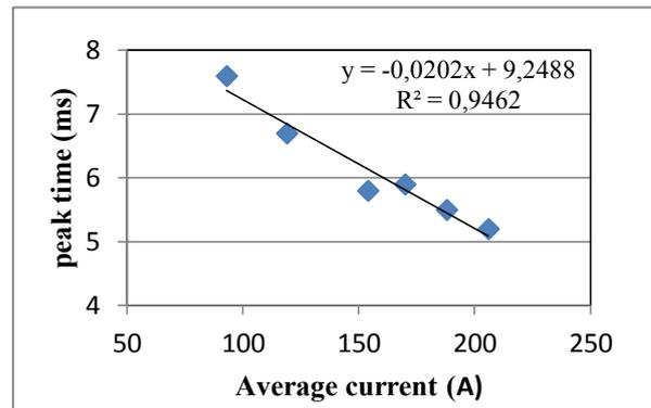
Figure 3 - Relationship between average current and peak time raised for  $I_p = 250$  A, wire AWS ER70S-6 and protection with using a mixture of Ar + 2% O<sub>2</sub>
