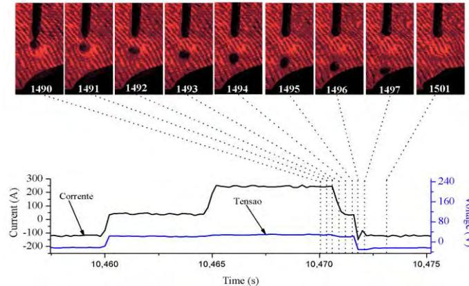
Figure 8 – Graphic of metal transfer AC MIG/MAG process, showing a parameter regulation that produces "ODPP the end of the pulse. Approach B com 50%EN:  $I_m^+ = 165A$ ;  $I_p = 250A$ ;  $I_{b1} = I_{b2} = 40A$ ;  $t_p = 5,9ms$ ;  $t_{b1} = 6,4ms$ ;  $t_{b2} = 1ms$ ;  $F_s = 4,7m/min$ ;  $I_n = 126A$ ;  $t_n = 7,6ms$ ;  $I_{(mg)} = 147A$ ;  $T = 19ms$ ;  $CTWD = 25mm$
