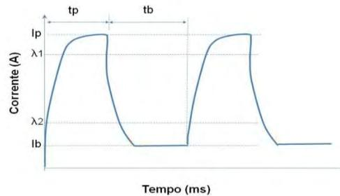
Figure 2 - Waveform for pulsed current of type Exponential, typical equipment capable of pulsed current
