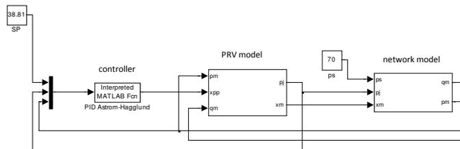
Figure 7: Simulation diagram of the system with Astrom-Hagglund tuning method.
