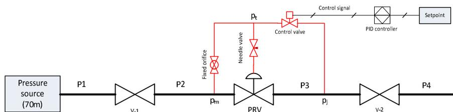
Figure 3: Test network with PID controller layout.
