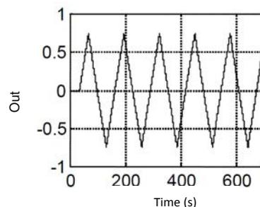
Figure 6: Example of critical period obtained to first order process.
