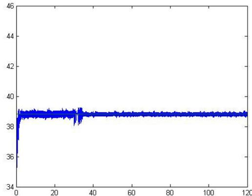
Figure 12: PRV downstream pressure profile obtained with the PID controller with gain scheduling method.
