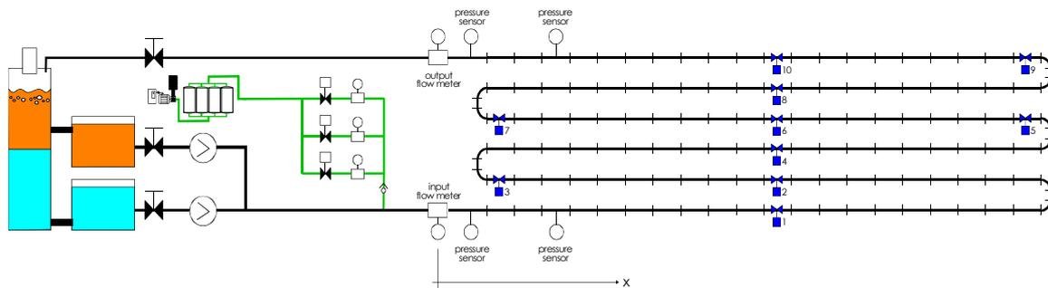
Figure 1. Schematic representation of the pilot pipeline at the Industrial Multiphase Flow laboratory.
