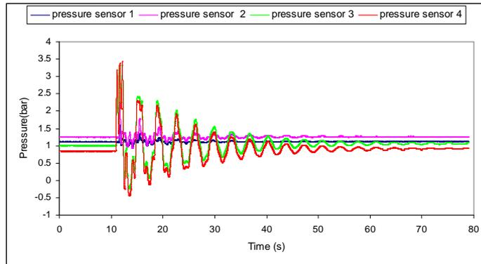
Figure 2. Experimental results in a pipeline without leak.
