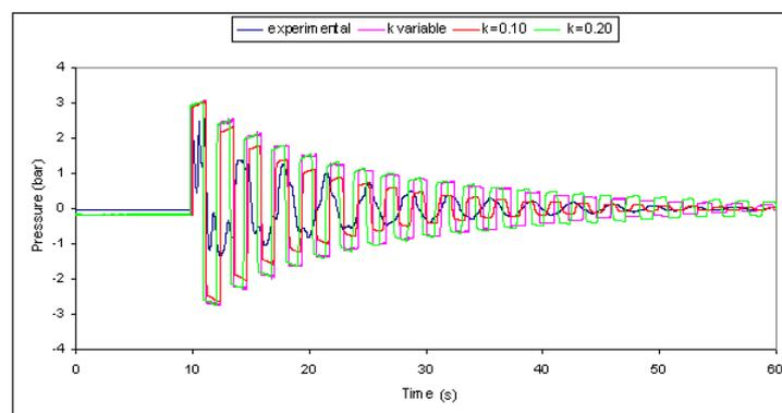
Figure 6. Comparison between numerical and experimental results in the pipeline without leak.
