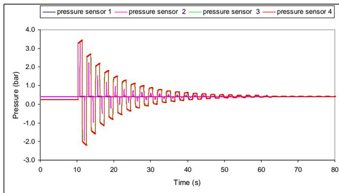
Figure 3. Numerical results in a pipeline without leak.
