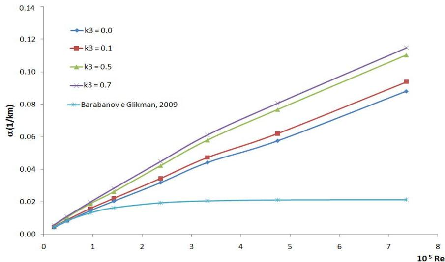
Figure 9. Comparison of numerical and experimental results, dependence of the attenuation coefficient on the Reynolds number
