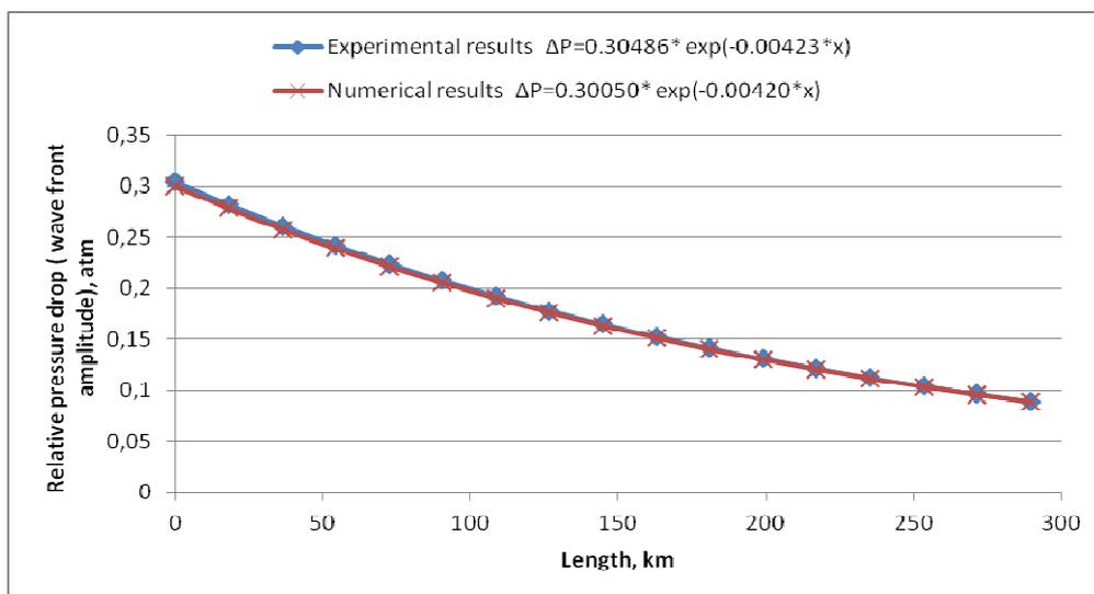
Figure 8. Variation of the perturbation amplitude along pipeline: experimental results and numerical results.
