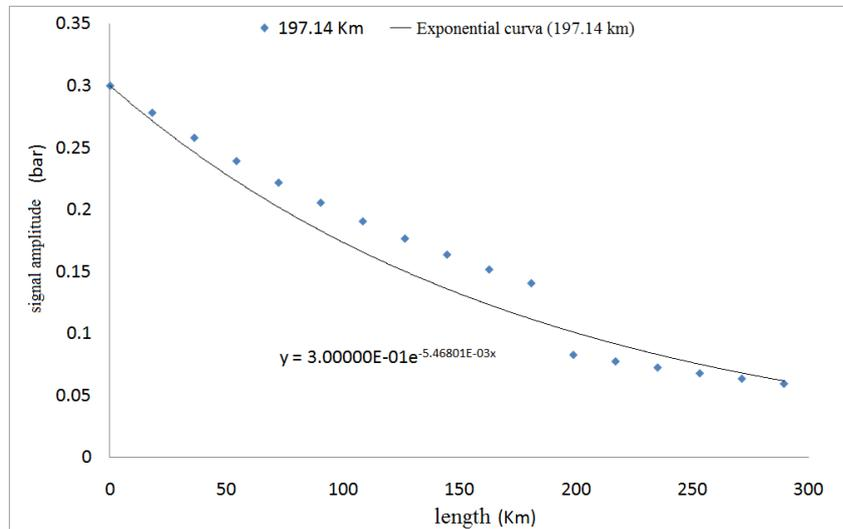
Figure 10. Obtaining the apparent attenuation coefficient.
