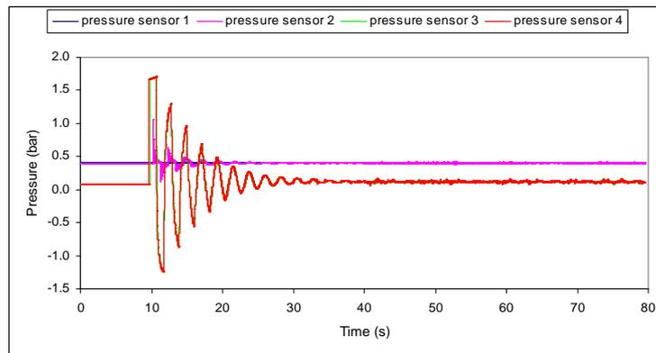
Figure 5. Numerical results in a pipeline with a leak in solenoid valve 1.
