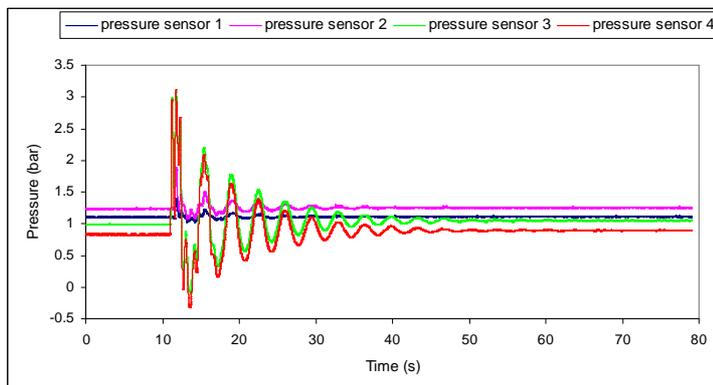
Figure 4. Experimental results in a pipeline with a leak in solenoid valve 1.
