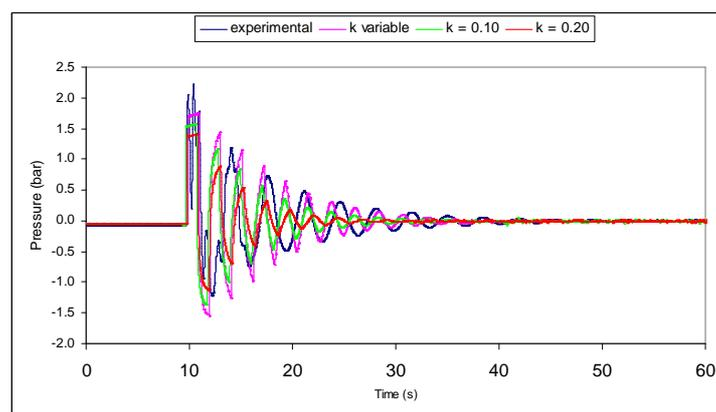
Figure 7. Comparison of numerical and experimental results in the pipeline with a leak in solenoid valve 1.
