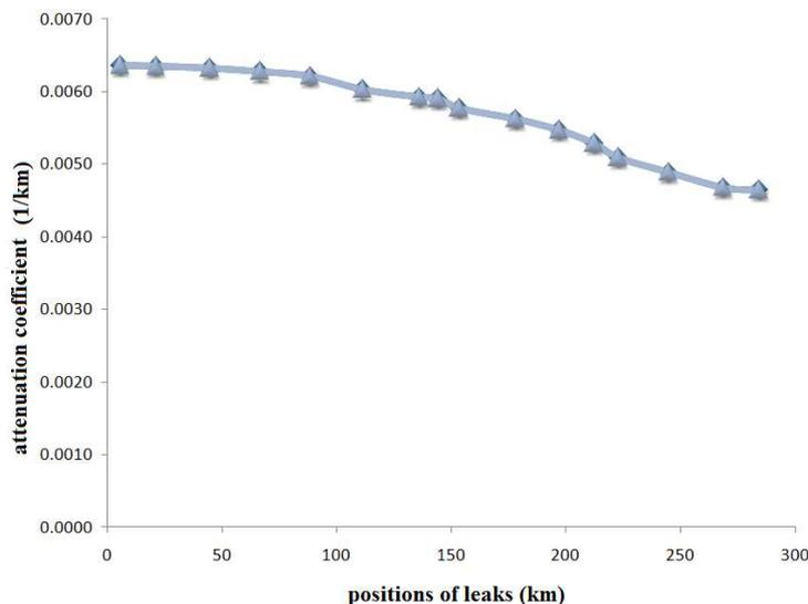
Figure 11. Behavior apparent attenuation coefficient depending on the position of the leak.
