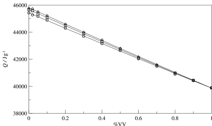
Figure 4. Heating values,  $Q$ , as a function volume fraction of biodiesel, for biodiesel-diesel blends: ◇, S10; □, S500; ○, S1800. (—) Eq. (4).
