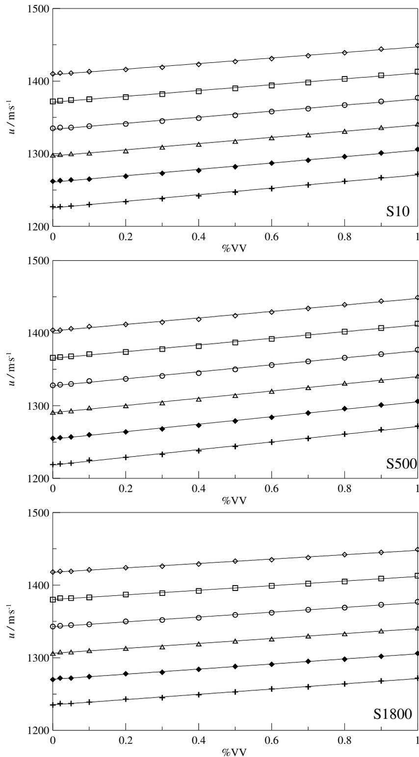
Figure 2. Speed of sound values,  $u$ , as a function volume fraction of biodiesel, for biodiesel-diesel blends as different temperatures:  $\diamond$ , 10 °C;  $\square$ , 20 °C;  $\circ$ , 30 °C;  $\triangle$ , 40 °C;  $\blacklozenge$ , 50 °C;  $\+$ , 60 °C. (—) Eq. (2).
