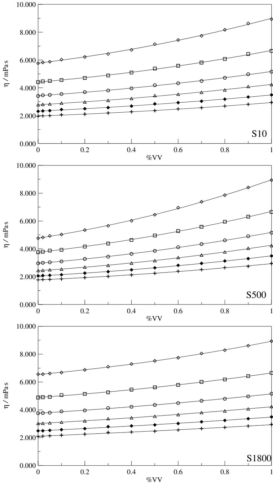
Figure 3. Viscosity values,  $\eta$ , as a function volume fraction of biodiesel, for biodiesel-diesel blends as different temperatures:  $\diamond$ , 10 °C;  $\square$ , 20 °C;  $\circ$ , 30 °C;  $\triangle$ , 40 °C;  $\blacklozenge$ , 50 °C;  $+$ , 60 °C. (—) Eq. (3).
