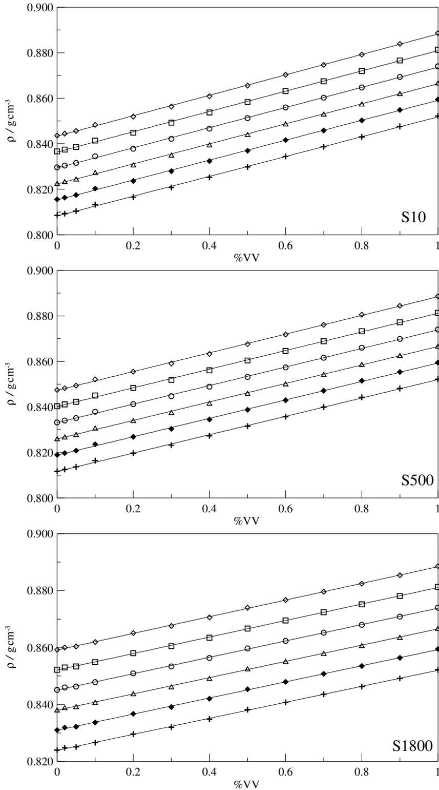
Figure 1. Density values,  $\rho$ , as a function volume fraction of biodiesel, for biodiesel/diesel blends as different temperatures:  $\diamond$ , 10 °C;  $\square$ , 20 °C;  $\circ$ , 30 °C;  $\triangle$ , 40 °C;  $\blacklozenge$ , 50 °C;  $+$ , 60 °C. (—) Eq. (1).
