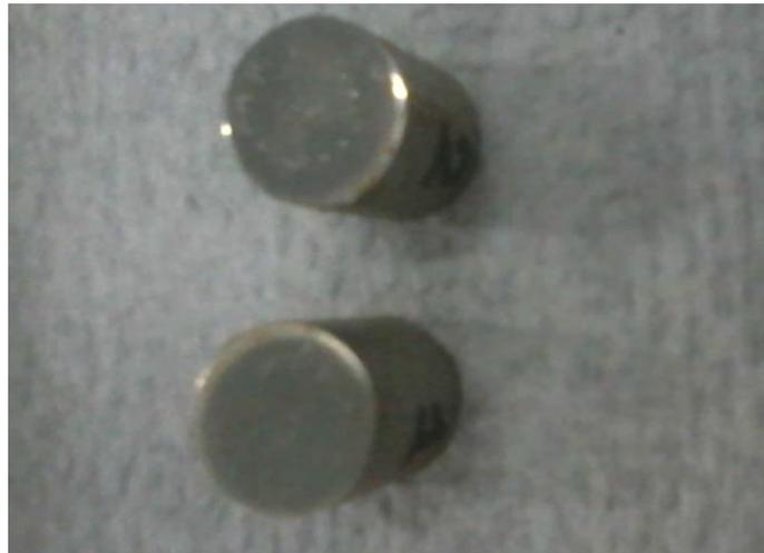
Figure 7. Interface AISI 316 - AISI 316 polished.
