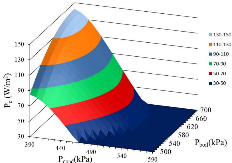
Figure 4. Behavior of specific power for the working fluid R152a.
