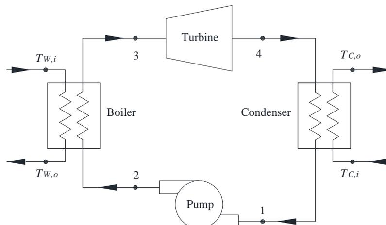
Figure 1. Scheme of a closed cycle of an OTEC plant.
