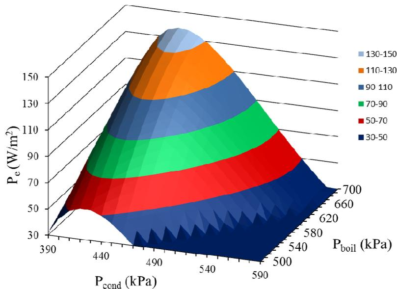
Figure 2. Behavior of specific power for the working fluid R-12.
