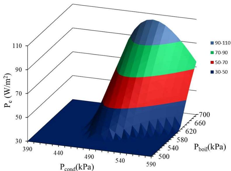
Figure 5. Behavior of specific power for the working fluid R500.
