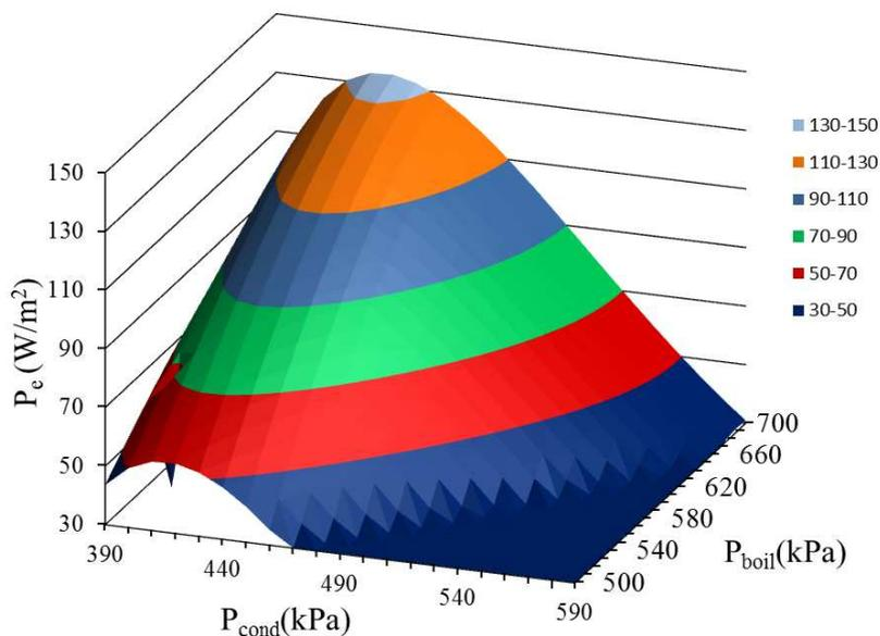
Figure 3. Behavior of specific power for the working fluid R134a.
