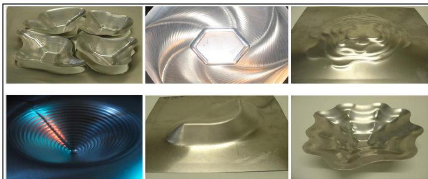
Figure 1. Several parts obtained by Incremental Sheet Forming
