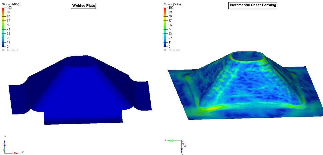
Figure 9. Stress contours before the impact
