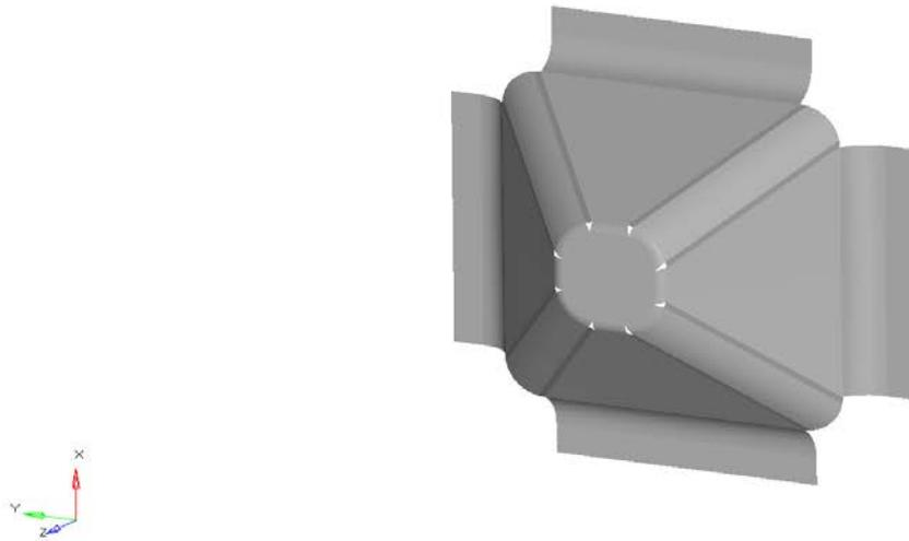
Figure 4. Impact Attenuator Model
