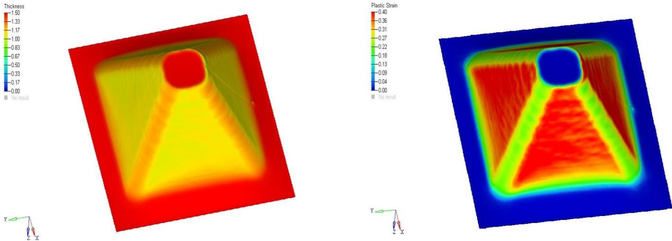
Figure 8. Thickness distribution (left). Plastic Strain contours (right)
