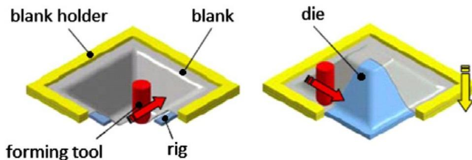
Figure 2. Comparison of SPIF(a) and TPIF(b) processes
