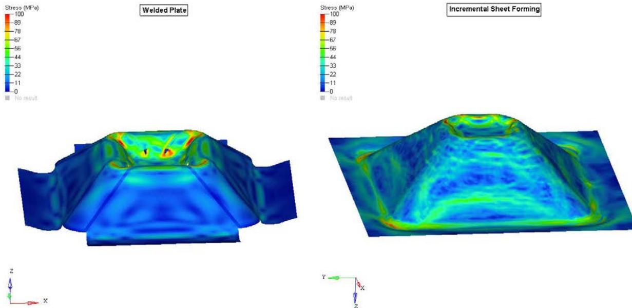
Figure 10. Stress contours after the impact
