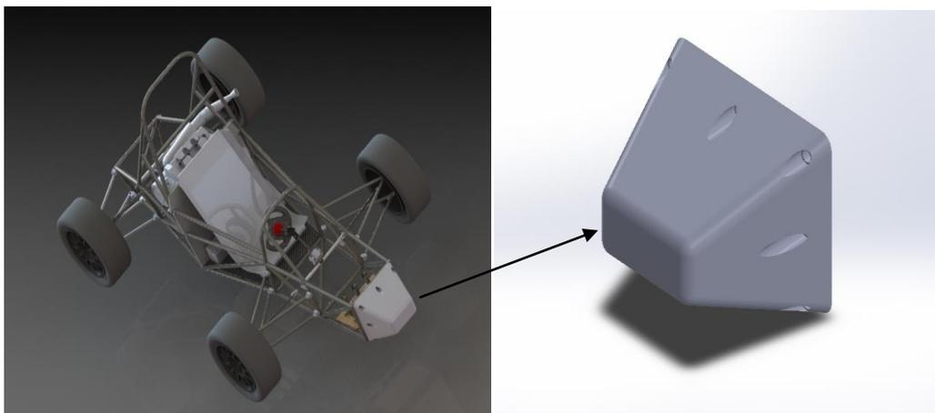
Figure 3. a) Formula SAE semi-finished prototype CAD of FSAE UFSJ. b) Impact attenuator template
