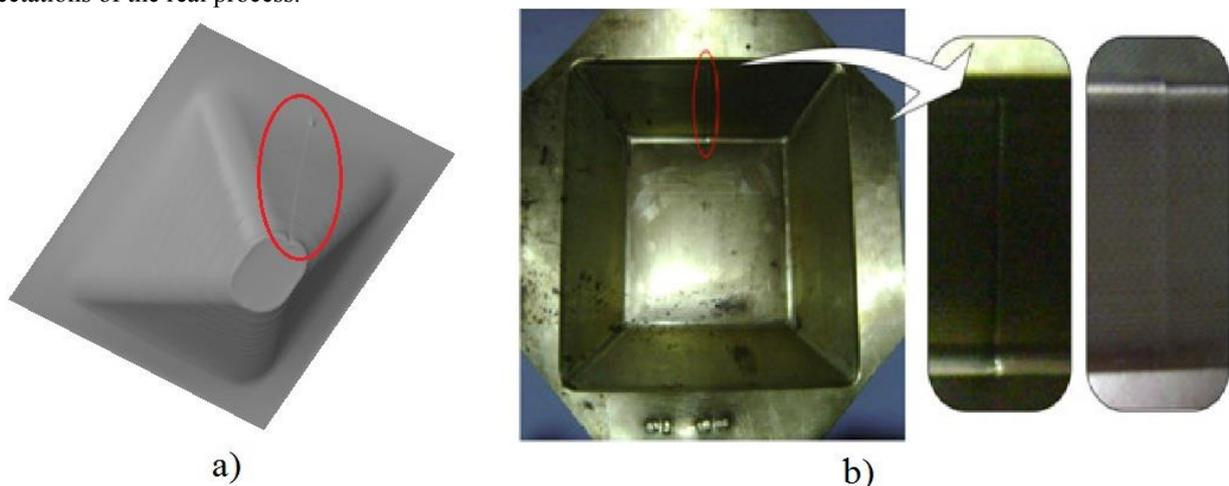
Figure 7. a) mark of the point of increment of ISF simulation; b) mark of the point of increment of the experimental ISF process (source: FRITZEN, p. 10)
