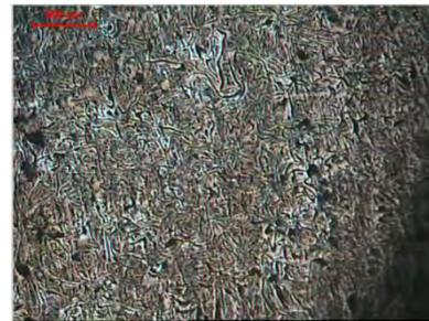
Figure 18. Microstructure of rupture extremity on plate with 100x increase.
