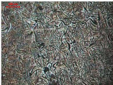
Figure 17. Microstructure of rupture center on plate with 100x increase.
