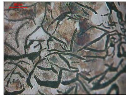
Figure 16. Microstructure of rupture extremity on plate with 50x increase.
