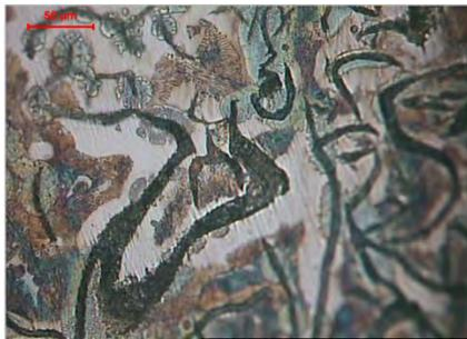
Figure 15. Microstructure of rupture center on plate with 50x increase.
