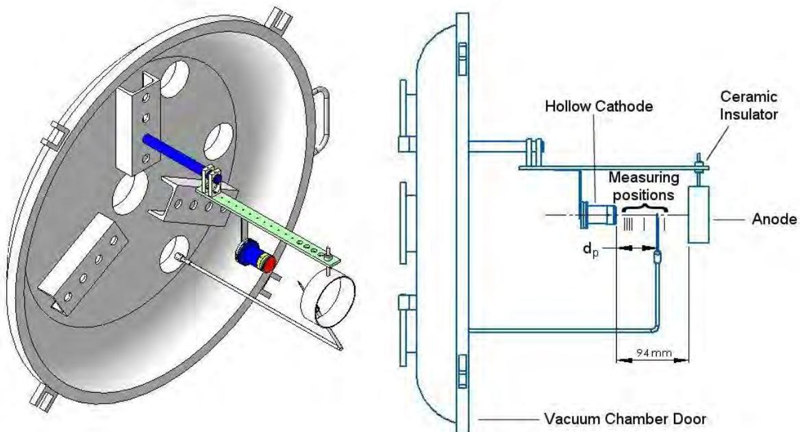
Figure 3. Hollow cathode assembled on the vacuum chamber door.  $d_p$ : distance from cylindrical probe to keeper.
