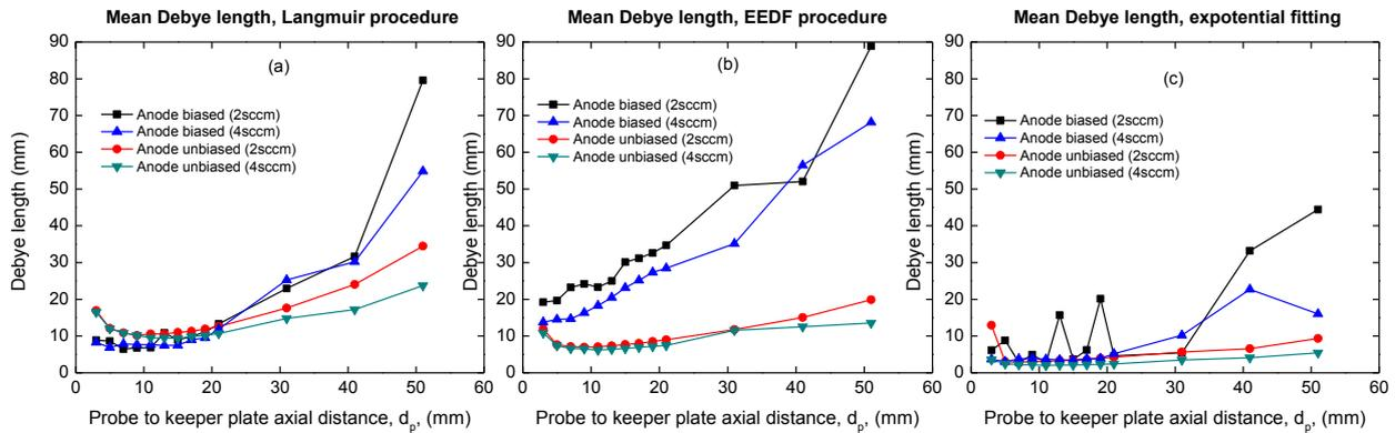
Figure 11. Mean Debye length obtained by Langmuir (a), EEDF (b) and exponential fitting (c) procedures.
