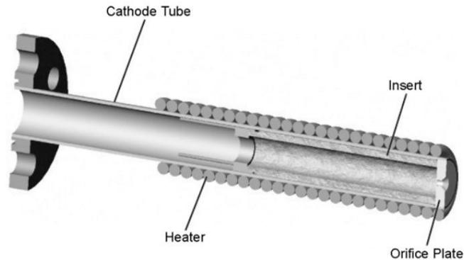
Figure 1. Typical hollow cathode geometry of a refractory metal tube with an emissive insert inside and a heater wrapped on the outside (Goebel & Katz, 2008).
