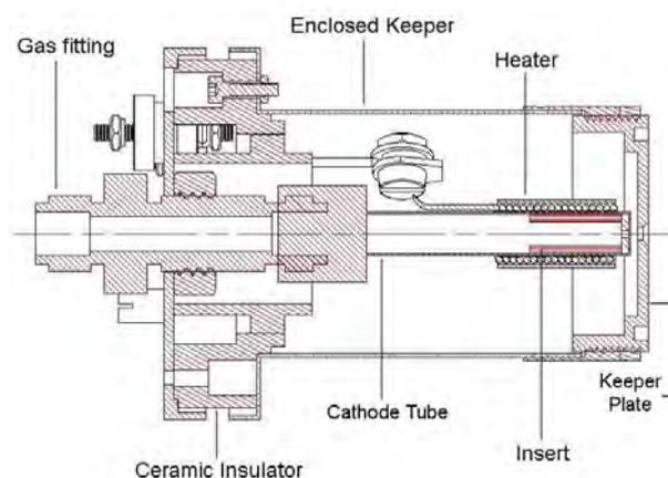
Figure 2. LAP hollow cathode schematics
