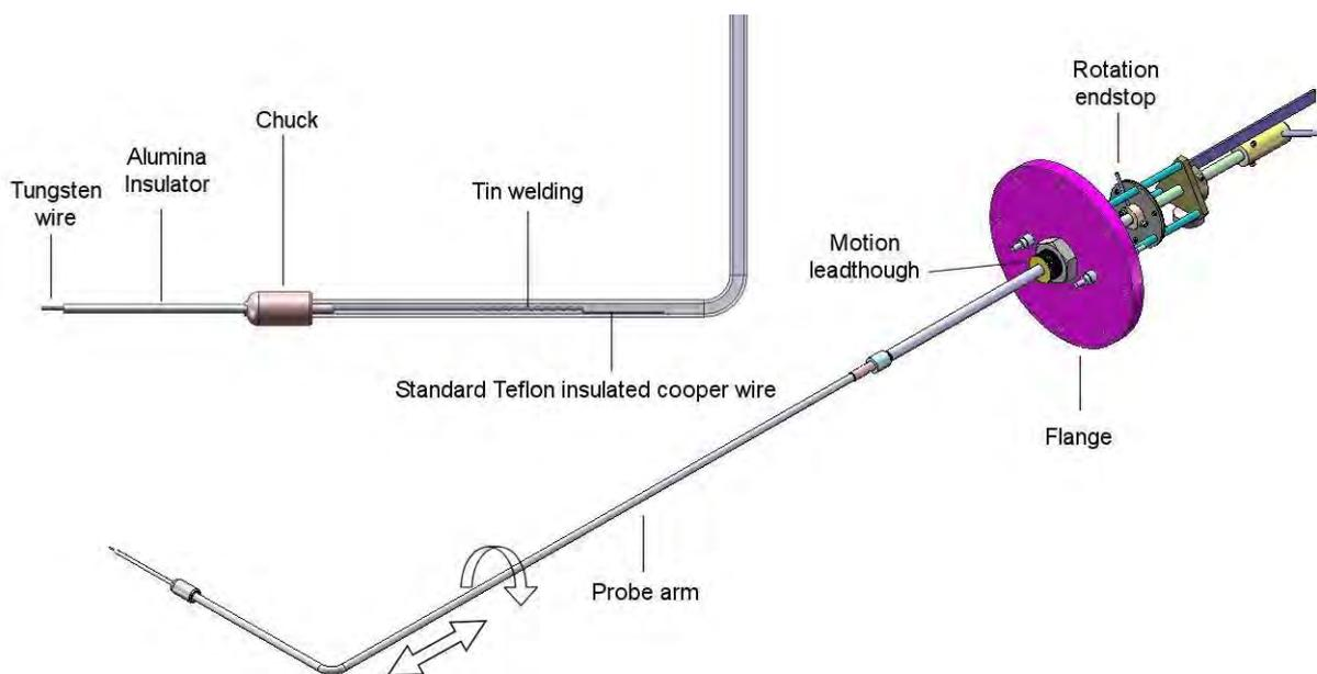
Figure 5. Cylindrical electrostatic probe schematics.
