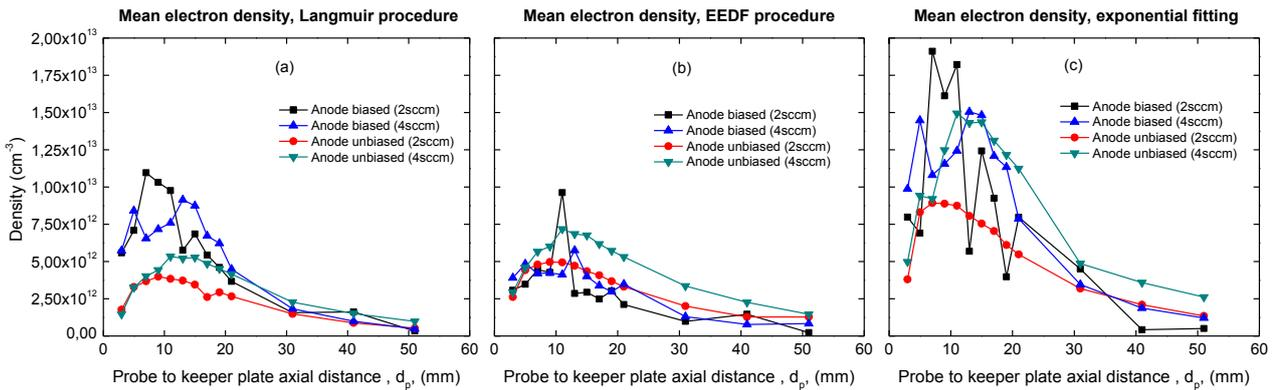
Figure 9. Mean electron density obtained by Langmuir (a), EEDF (b) and exponential fitting (c) procedures.
