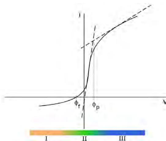
Figure 4. Typical I-V probe curves for different probe geometries. **I** is the ion saturation region; **II** is the transition region; and, **III** is the electron saturation region.  $\phi_f$ : floating potential,  $\phi_p$ : plasma potential.
