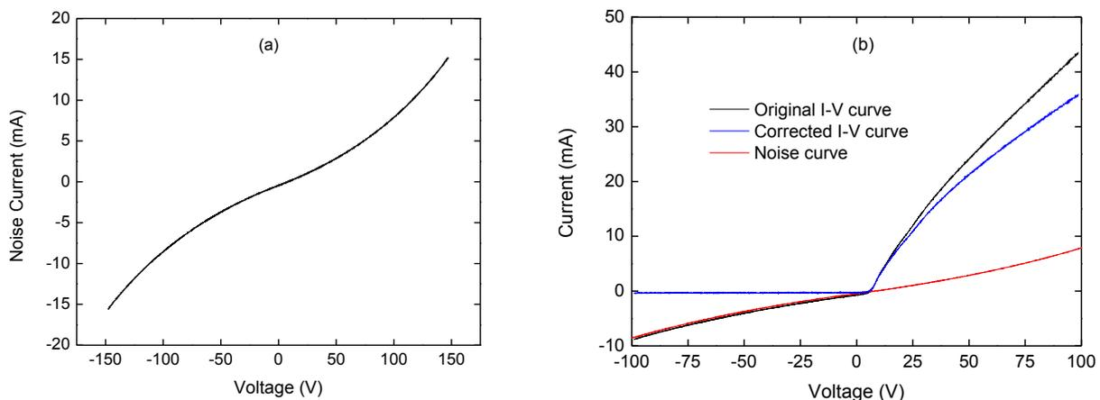
Figure 6. Power supply noise current (a) and example of I-V curve correction by noise subtraction (b).
