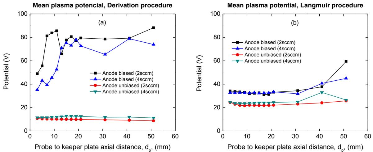
Figure 7. Plasma potential obtained using I-V curve derivation procedure (a) and Langmuir procedure (b)
