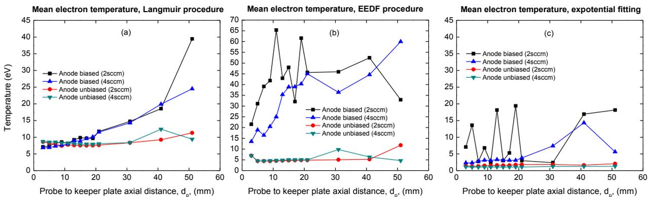
Figure 10. Mean electron temperature obtained by Langmuir (a), EEDF (b) and exponential fitting (c) procedures.
