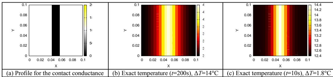
Figure 4. Profile for the contact conductance and exact temperatures for test case 2.
