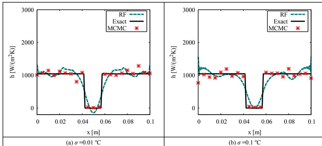
Figure 7. Recovered profile for the contact conductance for test case 2.
