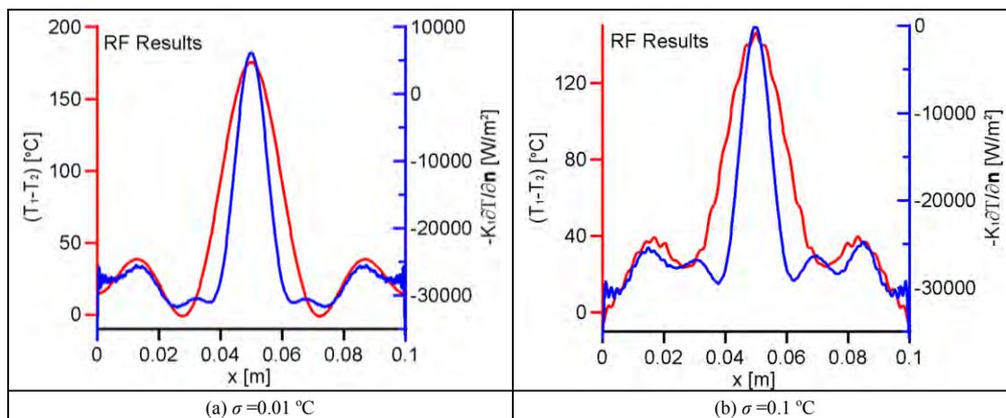
Figure 6. Recovered profile for the temperature difference and heat flux at the interface, for test case 1.
