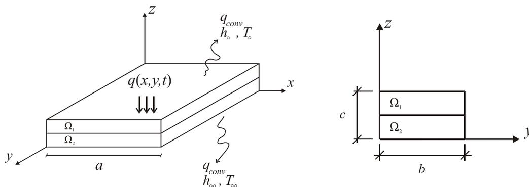
Figure 2. Geometry for a three-dimensional case
