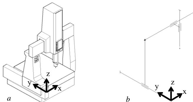
Figure 1. Movable bridge-type CMM (a) and diagram of the CMM (b)
