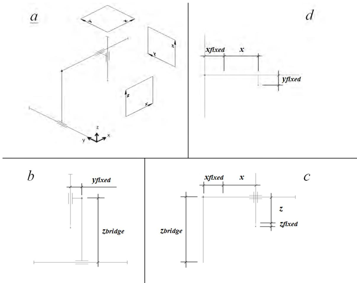
Figure 2. Definition of planes of CMM (a), side view (right) of the diagram proposed, yz plane (b); Front view of the diagram, xz plane (c), top view of the diagram, xy plane (d).
