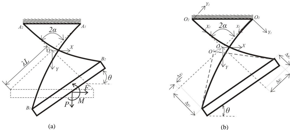
Figure 2. Shift of the rotary axis of the cross leaf-spring.
