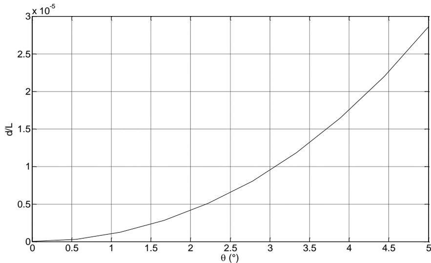
Figure 11. Center shift of cross leaf spring bearing,  $\alpha=30^\circ$  and  $\lambda =0.13$
