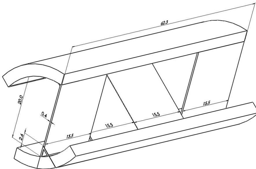
Figure 12. Cross leaf-spring bearing,  $\alpha=30^\circ$  and  $\lambda =0.13$
