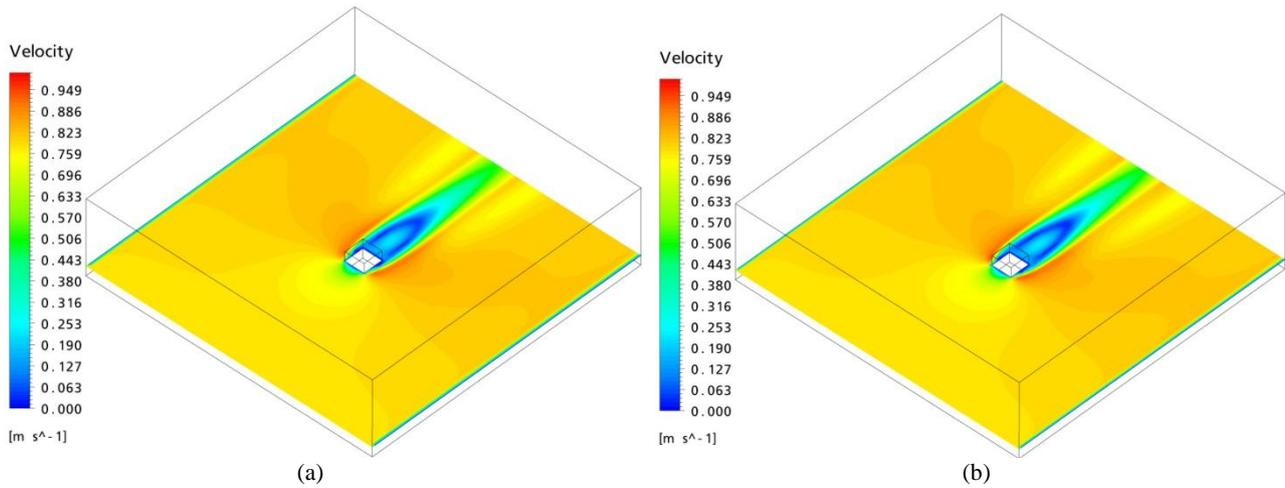
Figure 4 – Velocity contours for external domain mesh spacing (a) 0.80 m and (b) 0.60 m.
