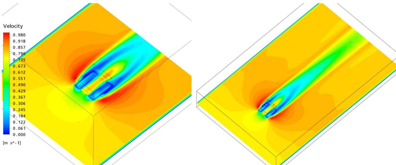
Figure 3 – Airflow around building (geometry 1): (a) Asfour and Gadi (2007) external box dimensions; (b) fully developed airflow external box dimensions.
