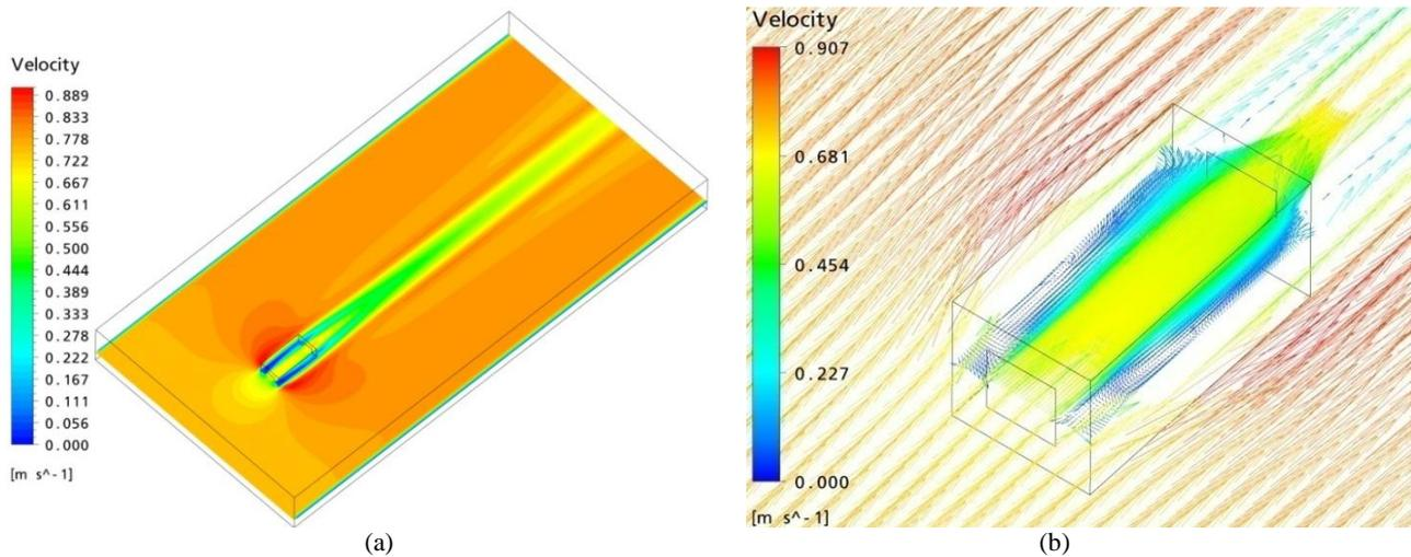
Figure 12 - Geometry 2 simulation results: (a) velocity contours; (b) velocity vectors.
