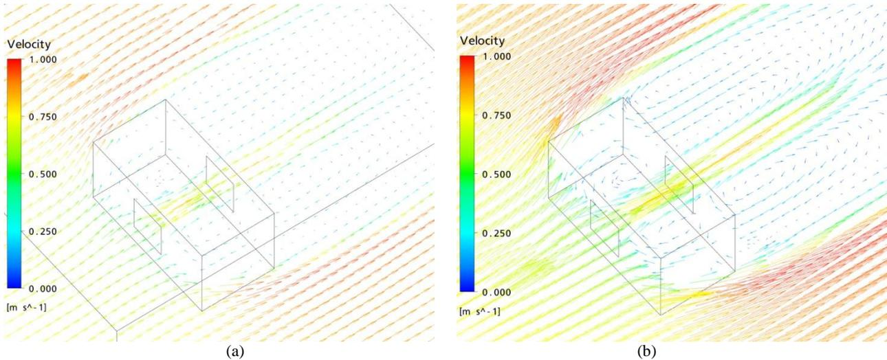
Figure 7 – Geometry 3 external airflow pattern for (a) 30 m x 30 m x 20 m external domain and for (b) building-proportional external domain (32 m x 76 m x 8 m).
