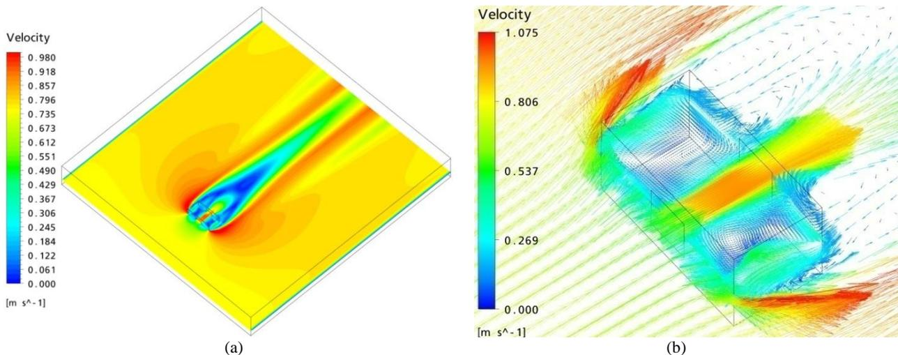
Figure 13 - Geometry 3 simulation results: (a) velocity contours; (b) velocity vectors.
