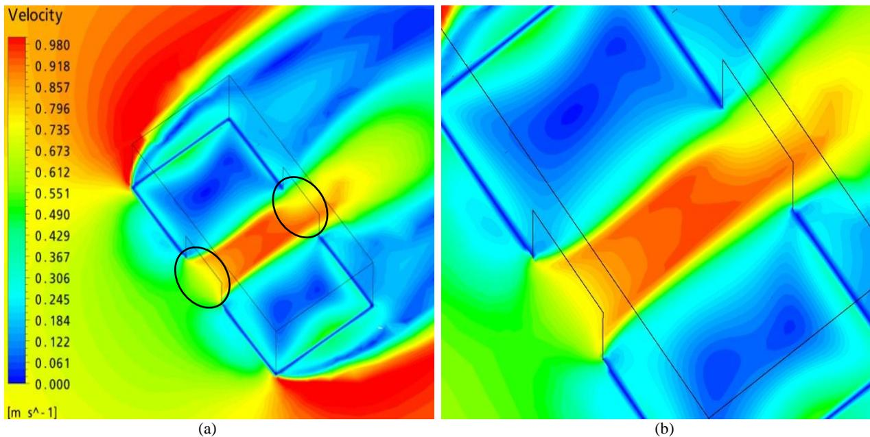
Figure 10 - Geometry 3 velocity contour for simulation with special interface between external and internal domains: (a) asymmetry was observed at exit opening; (b) openings magnification.
