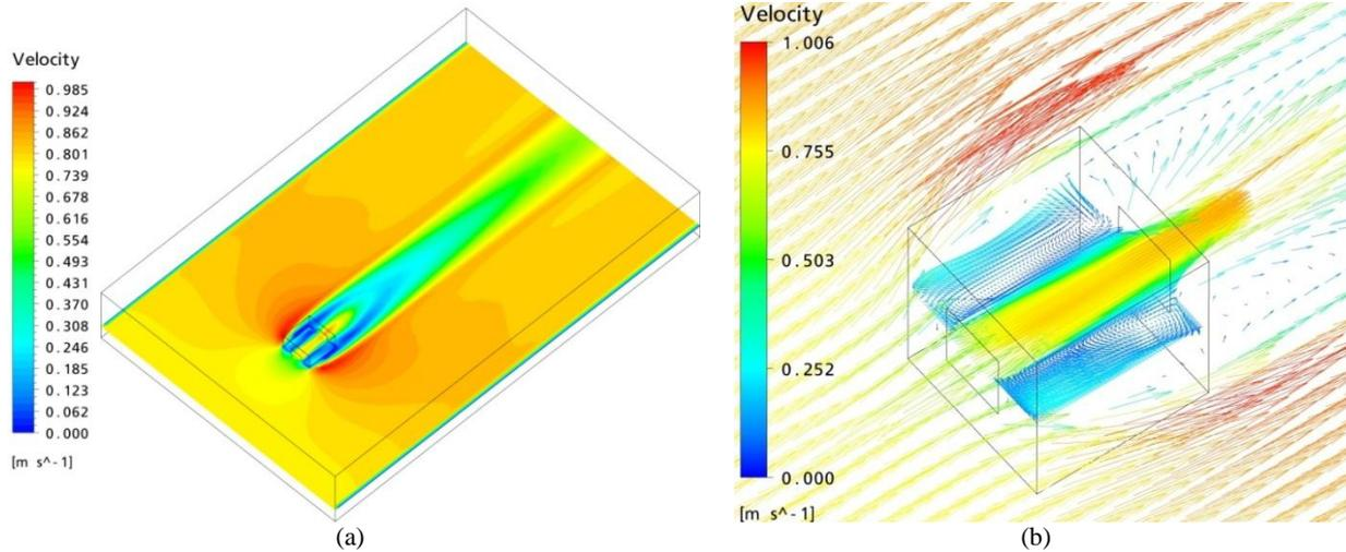
Figure 11 – Geometry 1 simulation results: (a) velocity contours; (b) velocity vectors.
