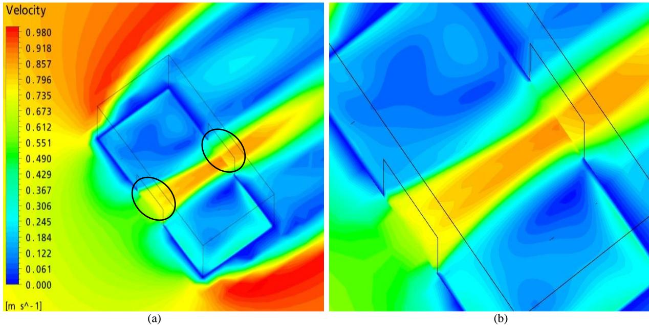
Figure 9 – Geometry 3 velocity contour for simulation without special interface between external and internal domains: (a) discontinuities were observed at openings; (b) openings magnification.
