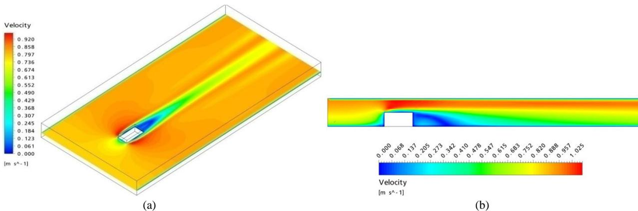
Figure 8 – Geometry 2 velocity contours for fully developed external airflow: (a) horizontal plane and (b) longitudinal plane.
