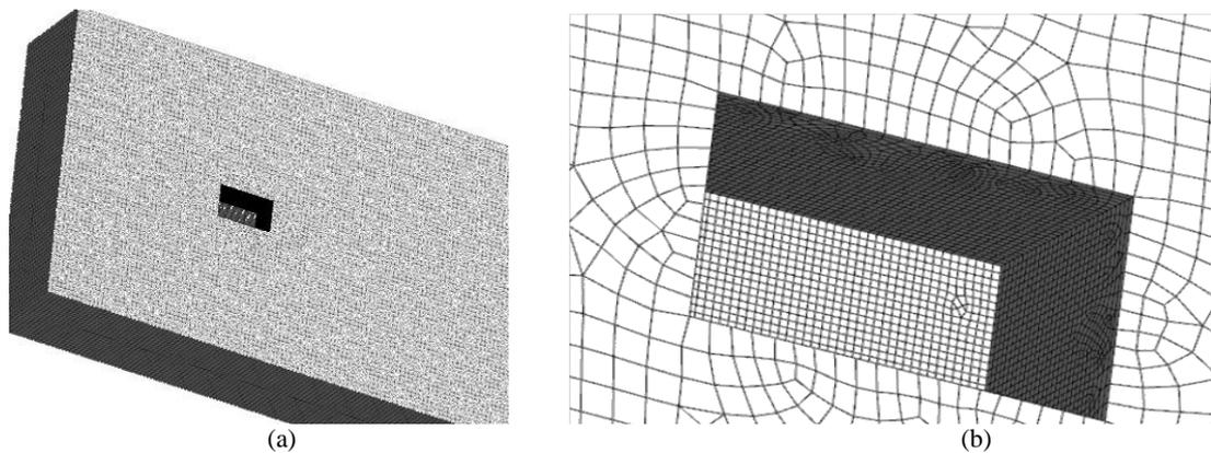
Figure 6 – External domain (a) overview and (b) interface refinement.
