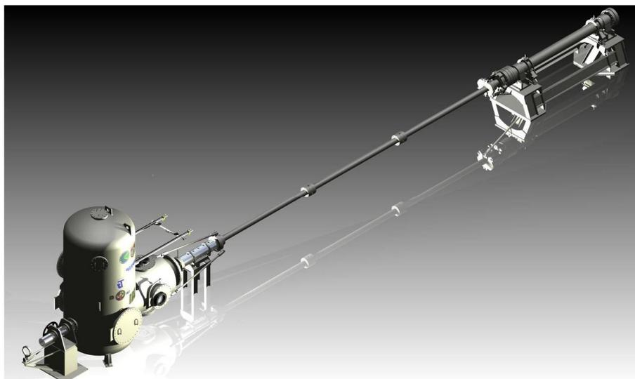
Figure 1. T3 0.60-m. nozzle exit diameter Hypersonic Shock Tunnel.
