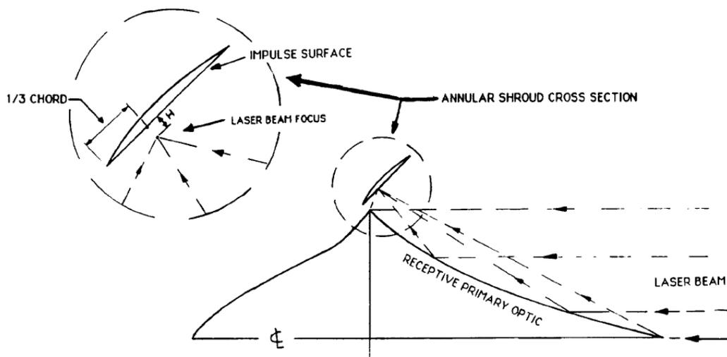
Figure 3. Side view of the lightcraft vehicle showing its principle of operation (Adapted from Myrabo, 1988).
