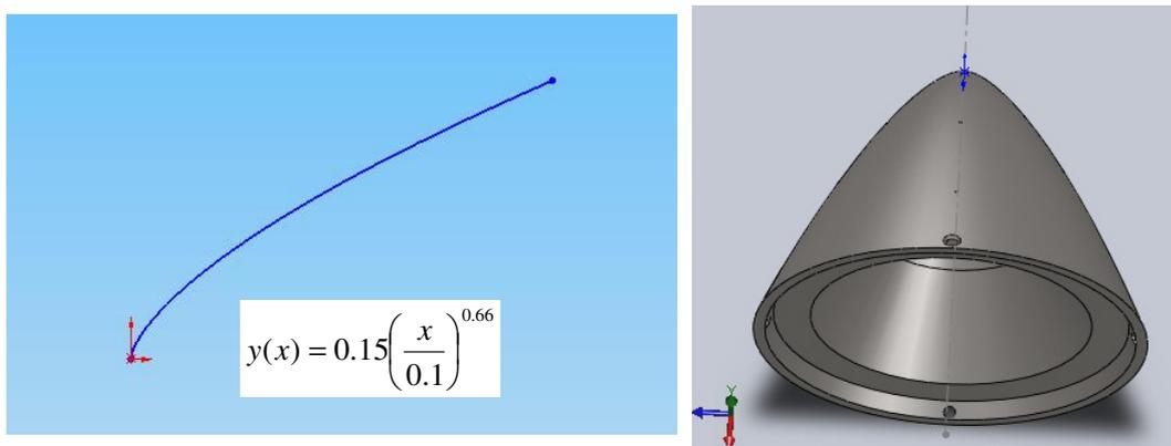
Figure 4. Lightcraft nose contour (left) and 3D CAD configuration (right).
