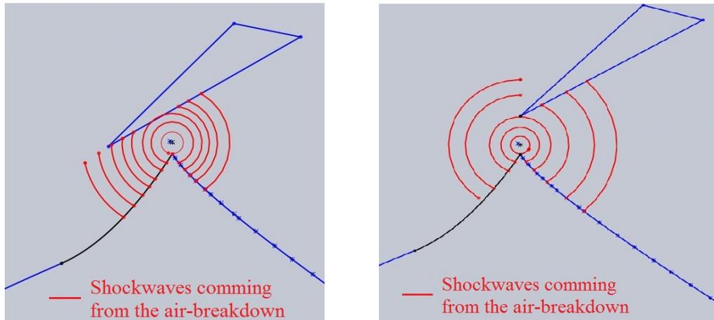
Figure 7. Shroud tip in position forward (left) and rearward (right) of the focal point.
