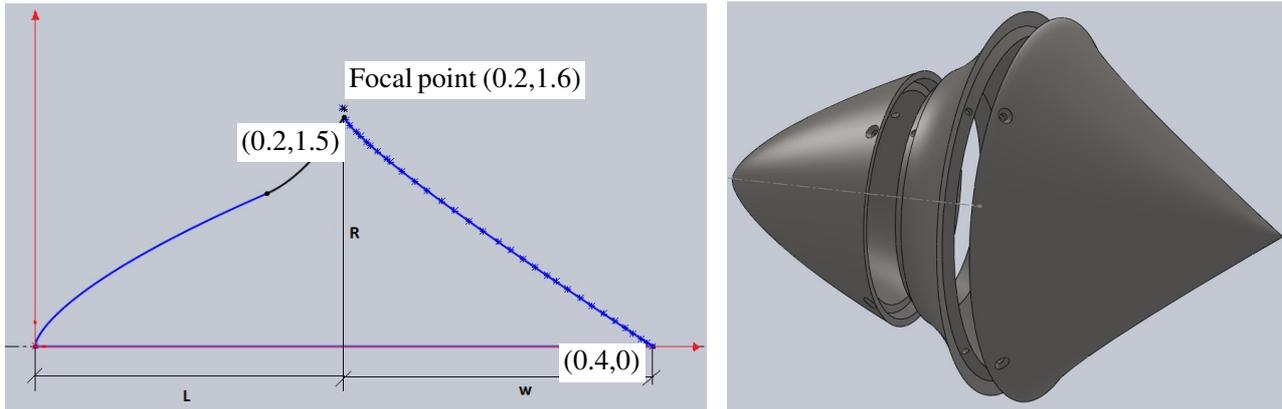
Figure 5. Contours of both forebody and afterbody (left) and 3D CAD forebody plus plug nozzle (right).
