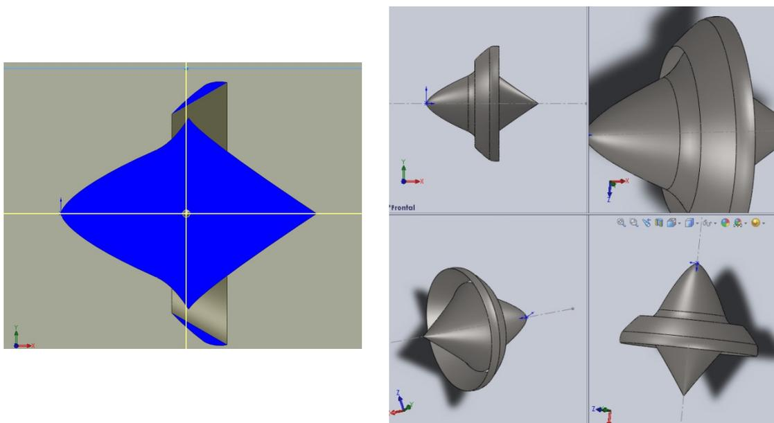
Figure 9. 2D view of the lightcraft (left) and 3D CAD lightcraft (right).
