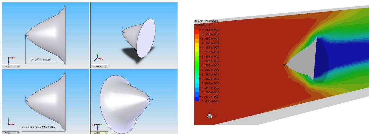
Figure 6. Lightcraft forebody configuration (left) and CFX velocity contours at Mach 6 (right).
