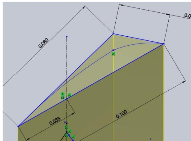
Figure 6. Comparison between the triangular and smoothed shroud contours (in meter).
