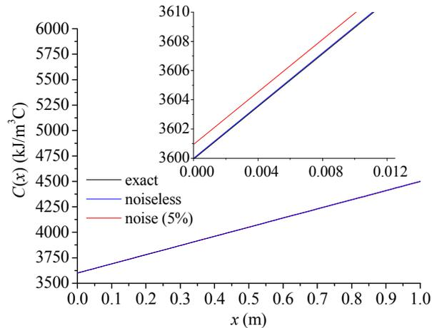
Figure 4: Estimated heat capacity  $C(x)$  for a plate of metal-like material by using the DE algorithm.
