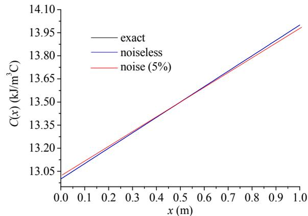
Figure 6: Estimated heat capacity  $C(x)$  for a plate of insulating material (fiberglass) by using the DE algorithm.
