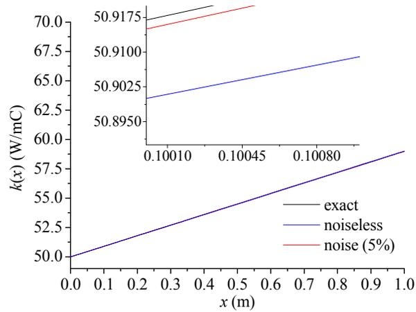
Figure 3: Estimated thermal conductivity  $k(x)$  for a plate of metal-like iron by using the DE algorithm.
