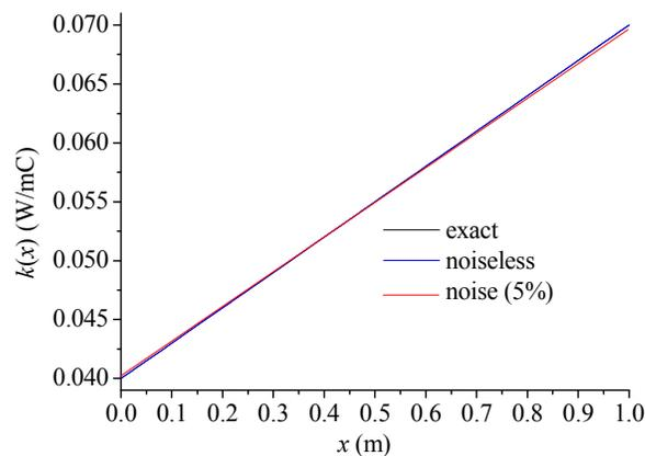
Figure 5: Estimated thermal conductivity  $k(x)$  for a plate of insulating material (fiberglass) by using the DE algorithm.
