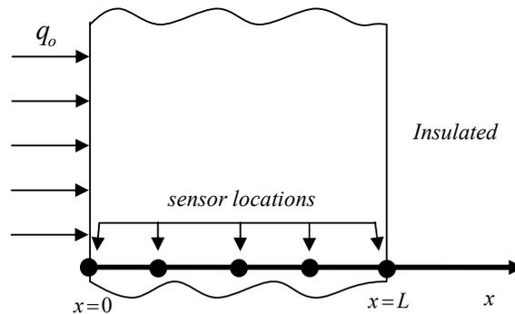
Figure 1: Geometry and coordinates of the heat conduction problem.
