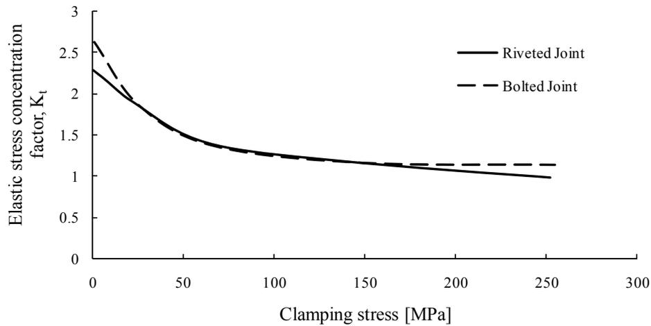
Figure 4. Evolution of the elastic stress concentration factor for riveted and bolted joints ( $\mu=0.35$ ).
