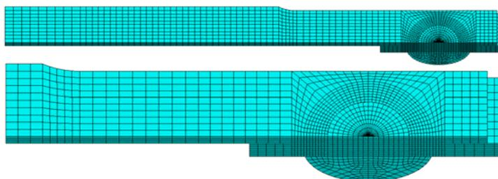
Figure 3. Finite element mesh of the riveted/bolted connection.
