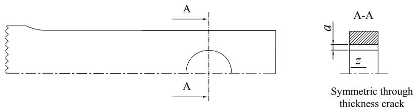
Figure 5. Through thickness constant depth crack configuration: crack depth  $a$ .
