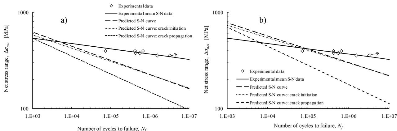
Figure 10. Fatigue life prediction for the bolted joint: a) clamping stress equal to 58 MPa; b) clamping stress equal to 254.72 MPa.
