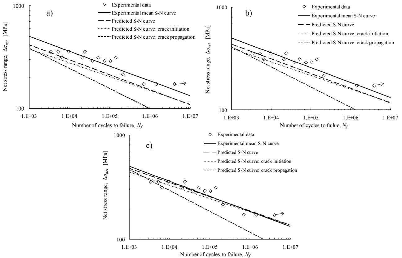
Figure 8. Fatigue life prediction for the riveted joint: a) clamping stress equal to 0.63 MPa; b) clamping stress equal to 8.94 MPa; c) clamping stress equal to 22.78 MPa.
