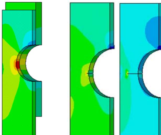
Figure 6. Illustration of the stress fields in the cracked and uncracked riveted joint (null clamping).
