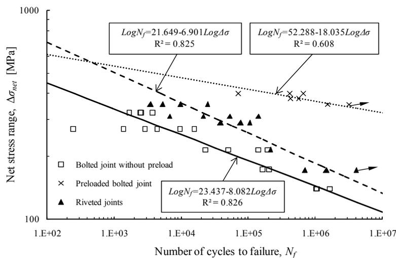
Figure 2. Comparison of constant amplitude S-N data between riveted and bolted joints.
