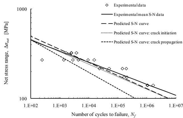
Figure 9. Fatigue life prediction for the bolted joint without preload on bolts.
