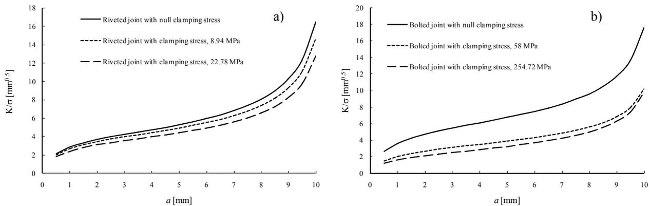
Figure 7. Stress intensity functions for constant depth cracks under distinct clamping stresses: a) riveted joint; b) bolted joint.
