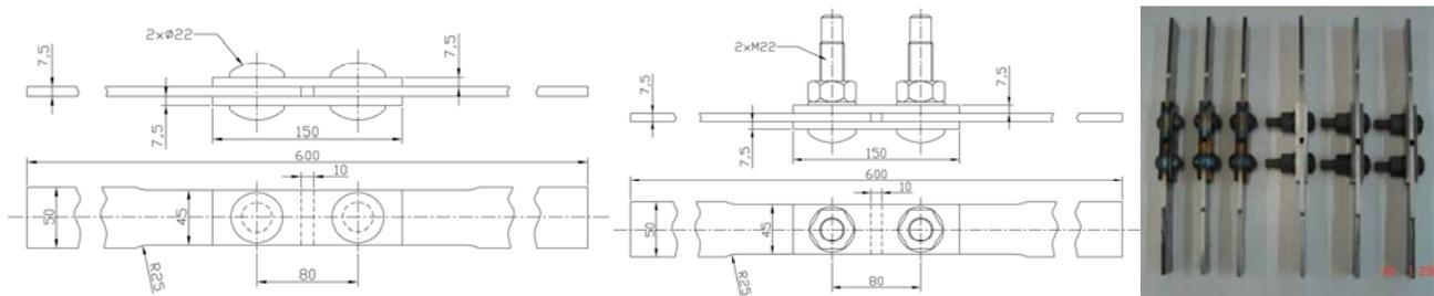
Figure 1. Riveted/bolted joints made of puddle iron from the Fão bridge.
