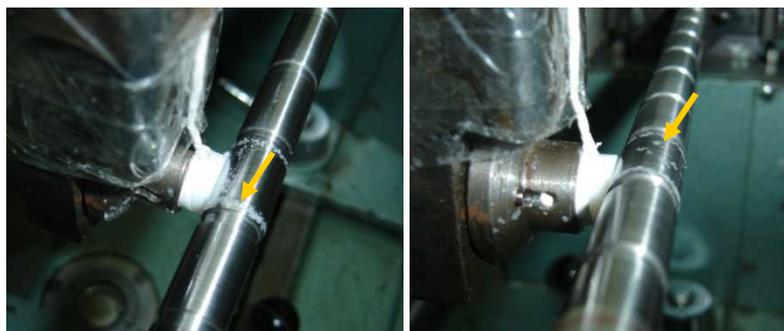
Figure 9. Image of the test PTFE – AISI 4140, arrow show the PTFE on the counterbody
