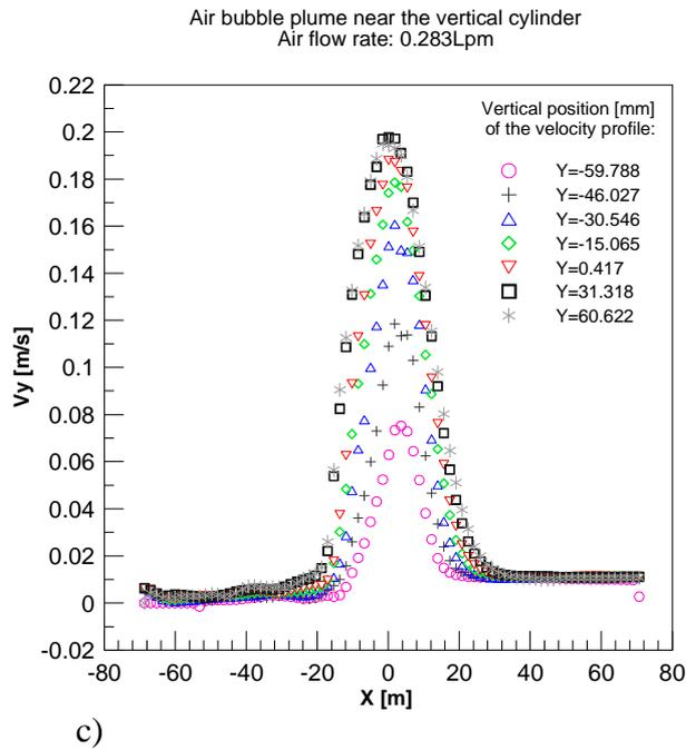
Figure 5- Velocity profile  $V_y$  of the liquid along the plane of the laser sheet, in several height  $Y$ . Air flow rate: 0.283Lpm. a) Axisymmetric bubble plume; b) Flat plate near the nozzle; c) Cylinder near the nozzle;
