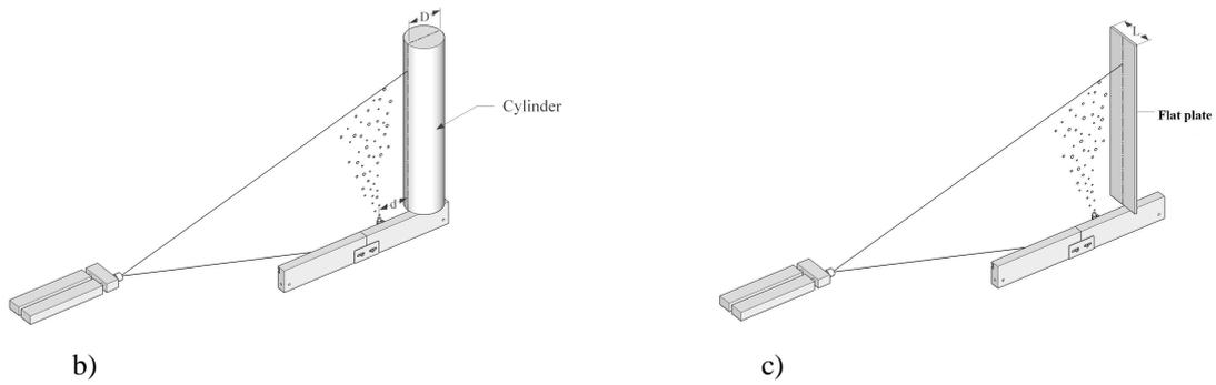
Figure 1- Schematic of experimental set up: a) tank; b and c) laser sheet on the solid surfaces
