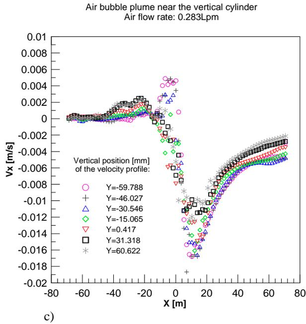
Figure 6 - Velocity profile  $V_x$  of the liquid along the plane of the laser sheet, in several height  $Y$ . Air flow rate 0.283Lpm . a) Axisymmetric bubble plume; b). Flat plate near the nozzle; c) Cylinder near the nozzle.
