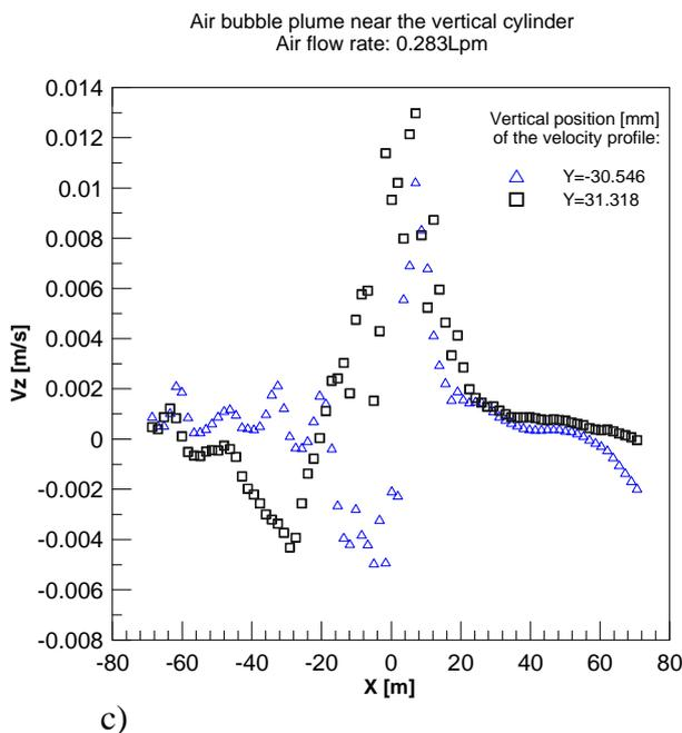
Figure 7- Velocity profile  $V_z$  of the liquid along the plane of the laser sheet, in two different height  $Y$ . Air flow rate 0.283Lpm . a) Axisymmetric bubble plume; b). Flat plate near the nozzle; c) Cylinder near the nozzle.
