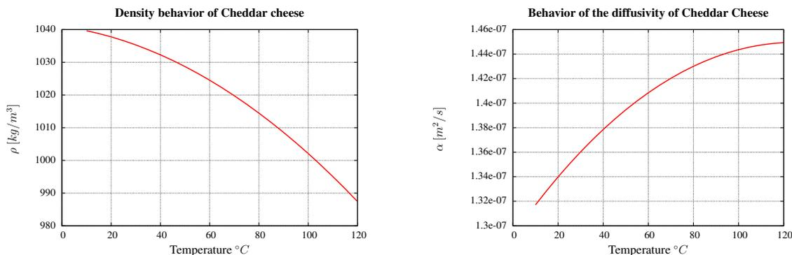
Figure 2. Behavior of density and diffusivity of cheddar cheese as a function of temperature.
