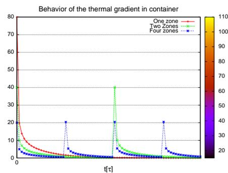
Figure 10. Behavior of the temperature gradient in the package as a function of the number of areas.
