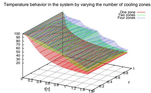
Figure 12. Temperature behavior of the food to be cooled with one, two or four cooling zones.
