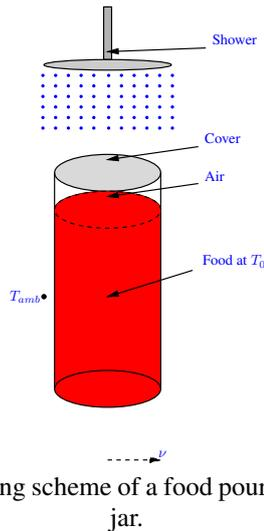
Figure 3. Cooling scheme of a food poured into a glass jar.
