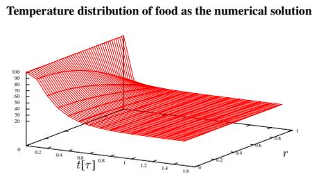
Figure 5. Temperature behavior in the food as a function of characteristic time and position.
