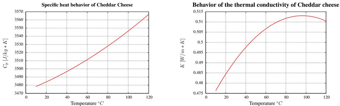
Figure 1. Behavior of specific heat and thermal conductivity of Cheddar cheese as a function of temperature.
