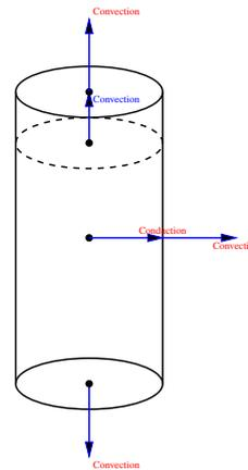
Figure 4. Forms of heat transfer in the food packaging during cooling.
