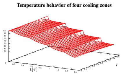
Figure 11. Temperature behavior of the food to be cooled with four cooling zones.
