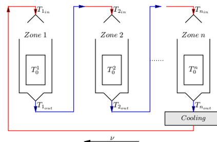
Figure 8. Cooling System Diagram interdependent without heating.
