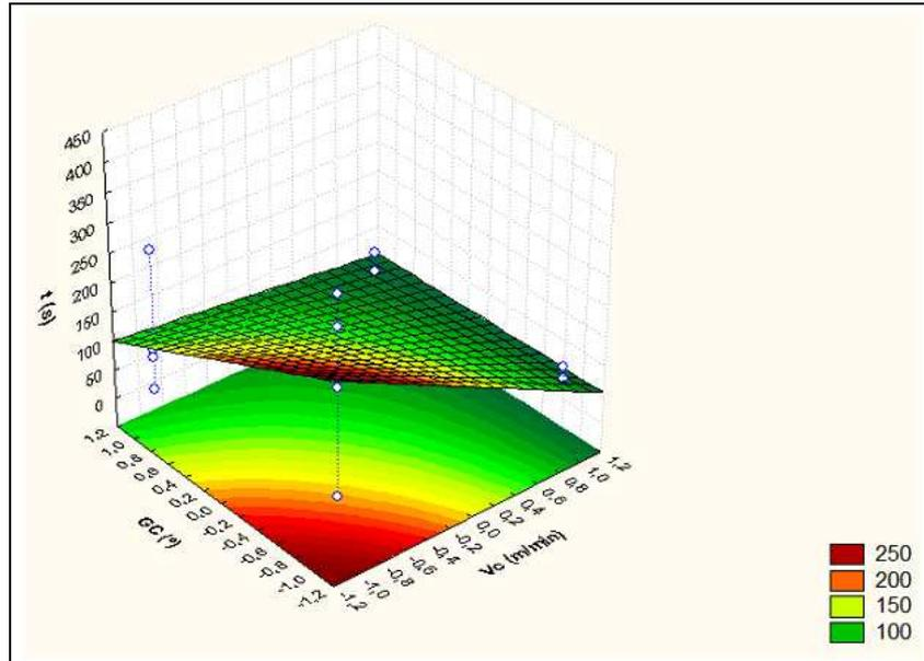
Figure 6. Influence of inputs parameters on the tool life . SiAlON ceramic inserts ( $\text{Si}_3\text{N}_4 + \text{Al}_2\text{O}_3$ ) x Mixed ceramic ( $\text{Al}_2\text{O}_3 + \text{TiC}$ )
