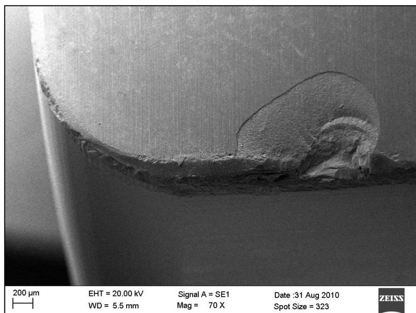
Figure 3. Average flank wear ( $VB_B$ ) on SiAlON ( $Si_3N_4 + Al_2O_3$ ) ceramic, after 60s. A large chipped area is also seen on the rake face
