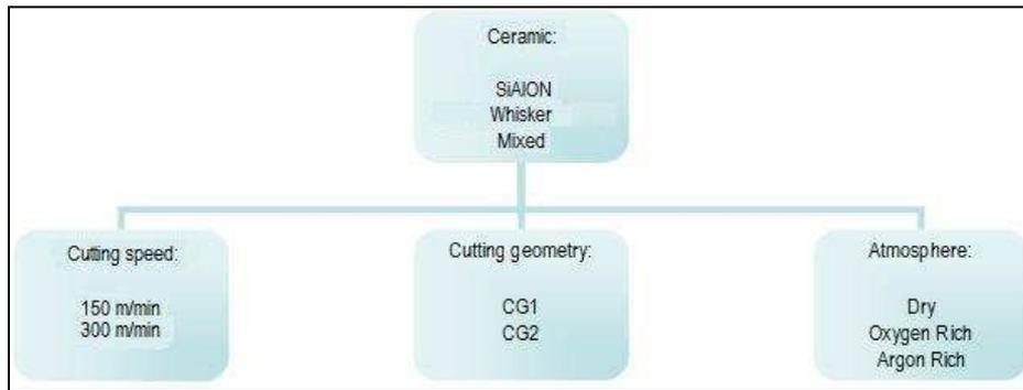
Figure 2. Scheme of tests with the ceramic inserts
