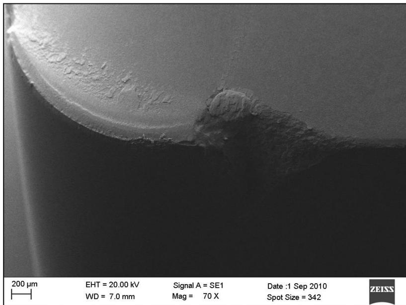
Figure 5. Notch wear ( $VB_N$ ) on Whisker ( $Al_2O_3 + SiC$ ) ceramic, after 20s
