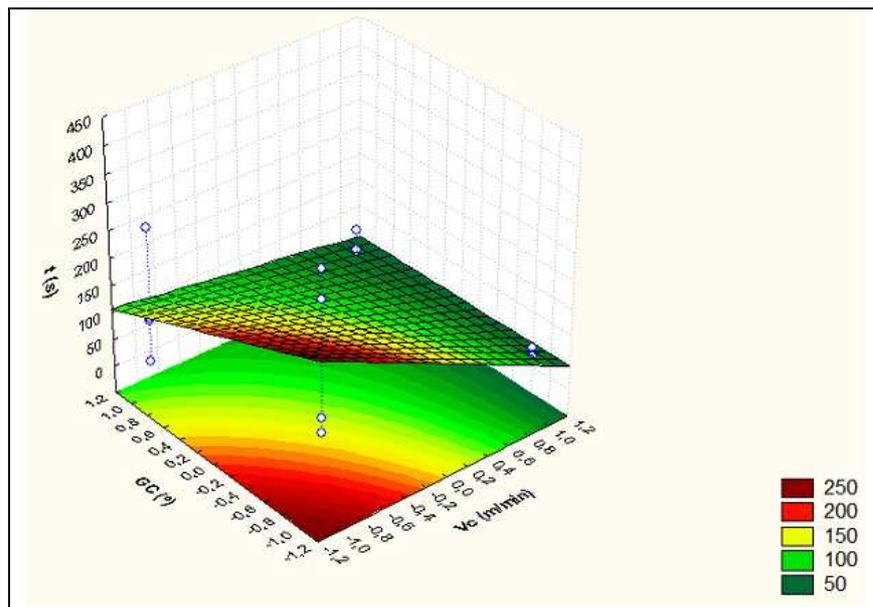
Figure 7. Influence of inputs parameters on the tool life . SiAlON ceramic inserts ( $\text{Si}_3\text{N}_4 + \text{Al}_2\text{O}_3$ ) x Whisker ceramic ( $\text{Al}_2\text{O}_3 + \text{SiC}$ )
