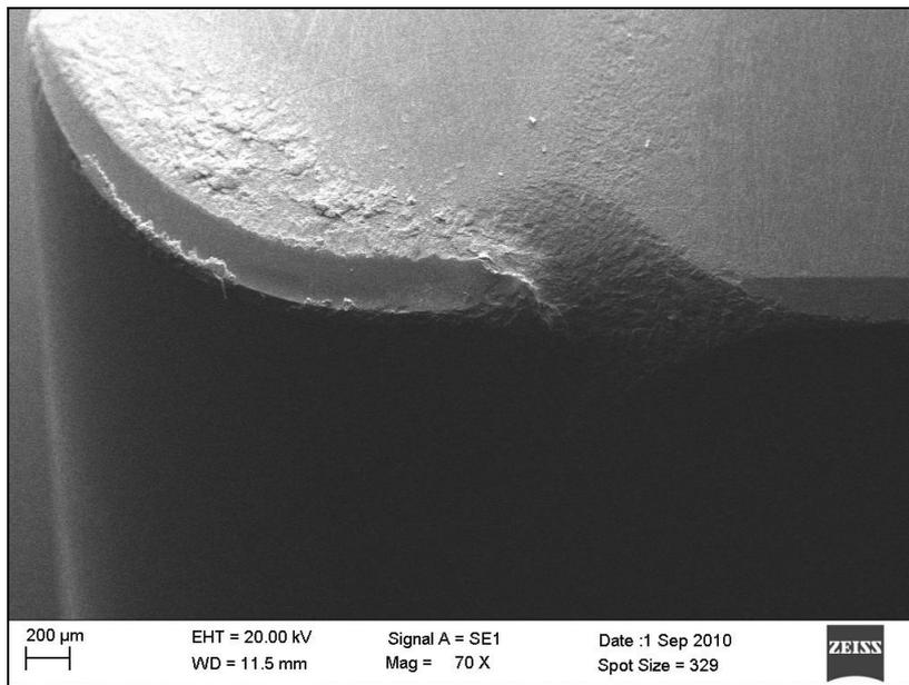
Figure 4. Notch wear ( $VB_N$ ) and nose wear ( $VB_C$ ) on Mixed ( $Al_2O_3 + TiC$ ) ceramic, after 60s
