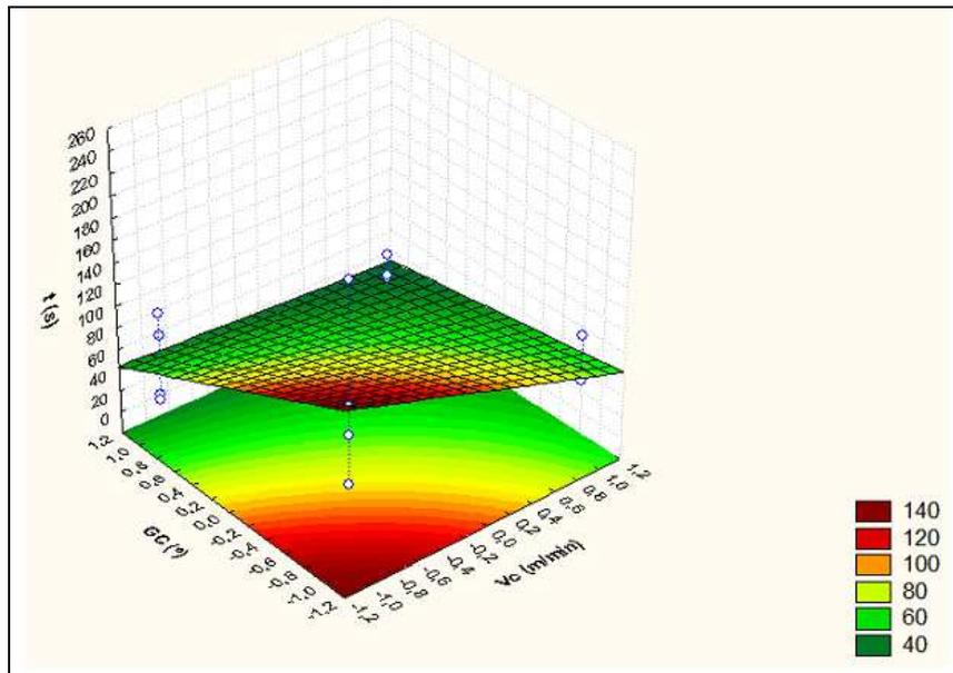
Figure 8. Influence of inputs parameters on the tool life . Mixed ceramic inserts ( $\text{Al}_2\text{O}_3 + \text{TiC}$ ) x Whisker ceramic ( $\text{Al}_2\text{O}_3 + \text{SiC}$ )
