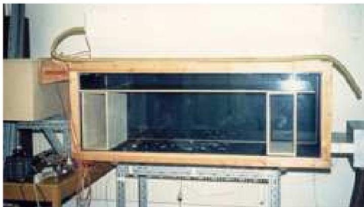
Figure 1. Experimental apparatus (Nielsen, 1976), source: <http://www.cfd-benchmarks.com>.
