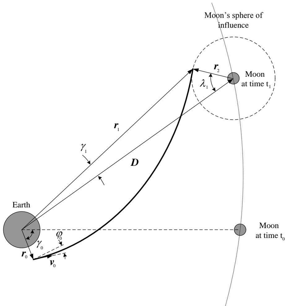
**Figure 1 – Geometry of the geocentric phase**
