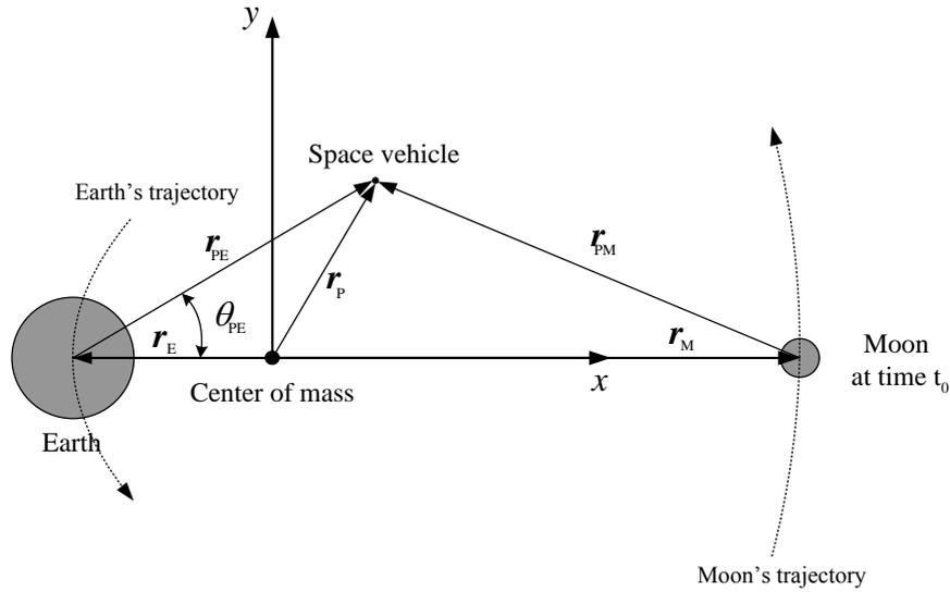
Figure 4 – Inertial reference frame Gxy
