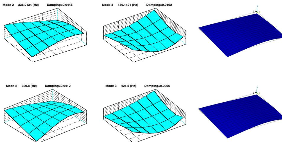
Figure 3. On upper line the Shapes modes for 5%, 10% nanoclay plate on the bottom line. On the left column the experimental spurious modes (336.0 Hz) for 5% nanocomposite and below (329.8 Hz) for 10% nanocomposite. At center column the experimental best fit for the 2<sup>th</sup> mode 430.1 Hz for 5% and 425.5 Hz for 10% nanocomposite, both out of phase by 180°. At right the final optimized FE shape mode.
