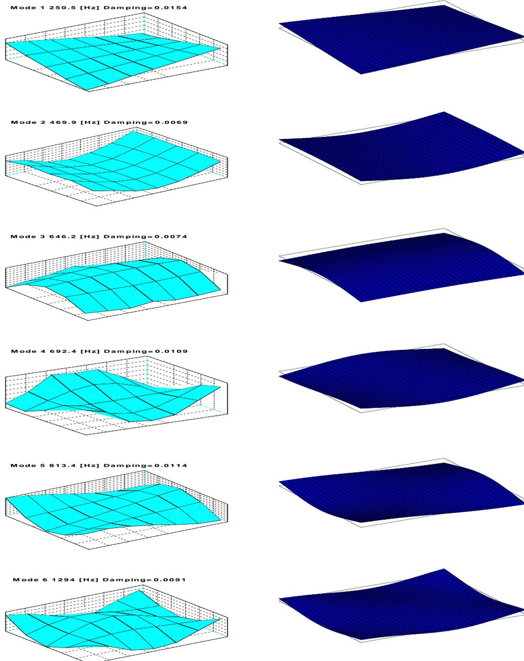
Figure 4. Shape modes for 1% nanocomposite plate, hammer method. At the left column the experimental shape modes at right the FE mode at the end of optimization process.
