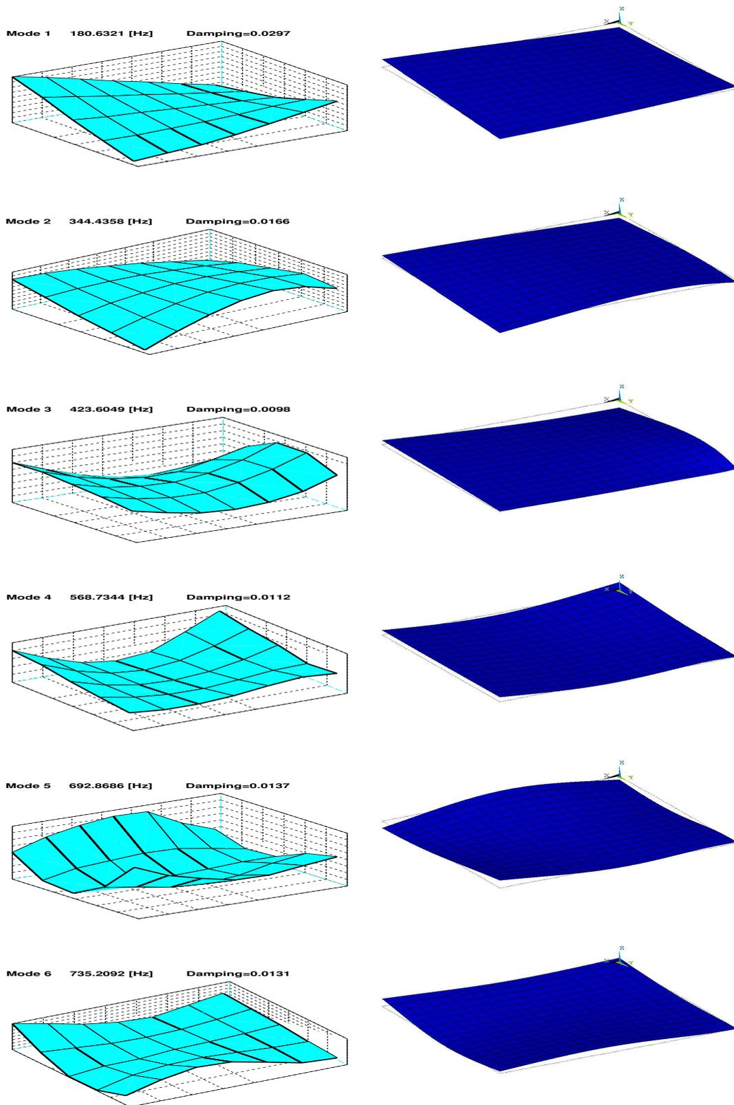
Figure 1. Mode shapes for Resin plate. At the left side the experimental shape modes at right the same modes at the end of the inverse approximation method.
