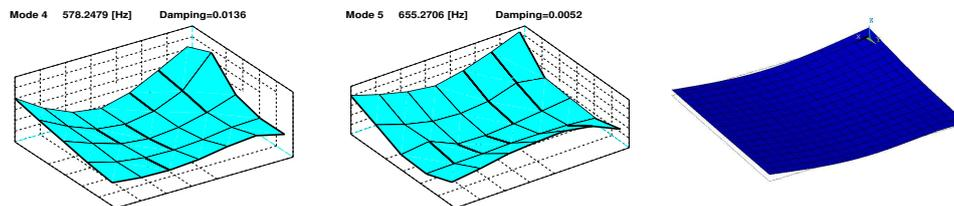
Figure 2. Shapes modes for 2% nanocomposite plate. At the left side the experimental 4<sup>th</sup> mode (578.0 Hz), at center the experimental spurious 5<sup>th</sup> mode (655.3 Hz) and at right the final optimized FE shape mode.
