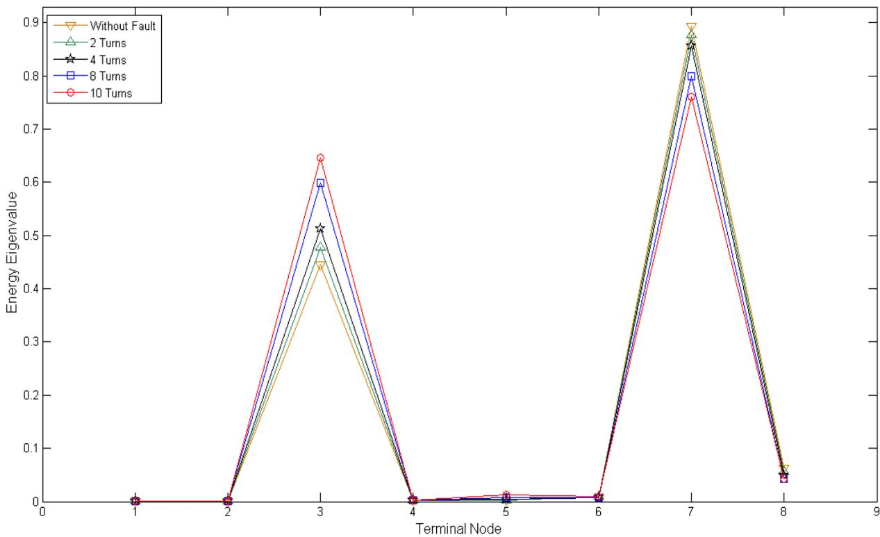
Figure 6. Graph for energy eigenvalues in each node for different conditions
