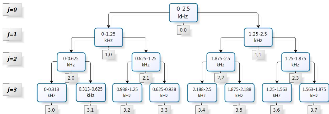
Figure 5. Diagram of an example of a 3 levels Wavelet Packet Transform decomposition
