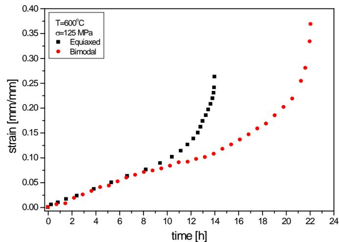
Figure 1: Creep curve at 600°C and 125 MPa.
