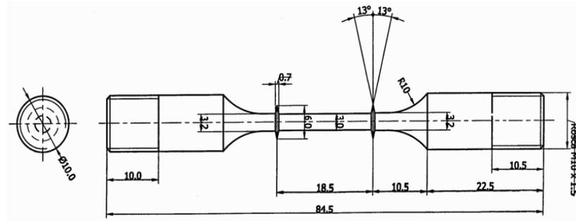
Fig. 1 Sample utilized for creep tests
