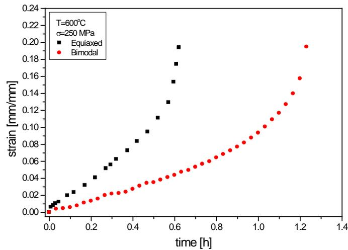
Figure 2: Creep curve at 600°C and 250 MPa.
