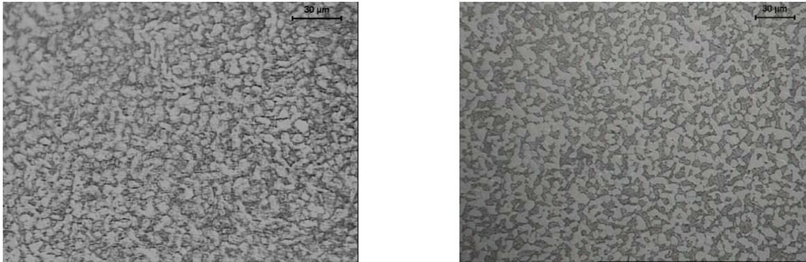
Fig. 2a – Micrograph of Ti-6Al-4V alloy as received
