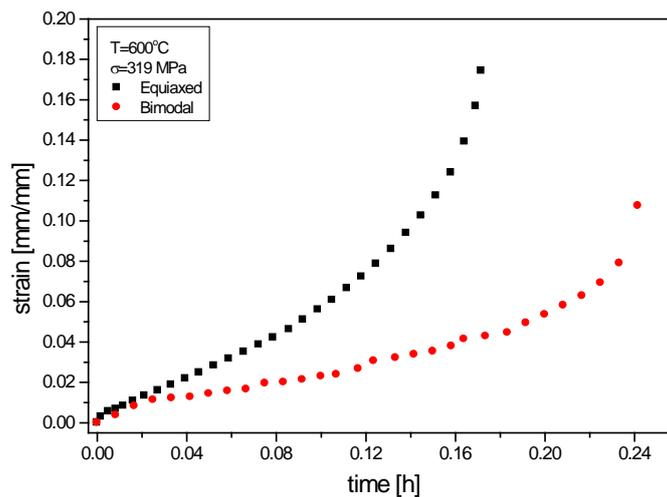
Figure 3: Creep curve at 600°C and 319 MPa.
