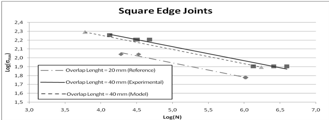
Figure 2: Fatigue tests Comparison between experiments and model prediction.
