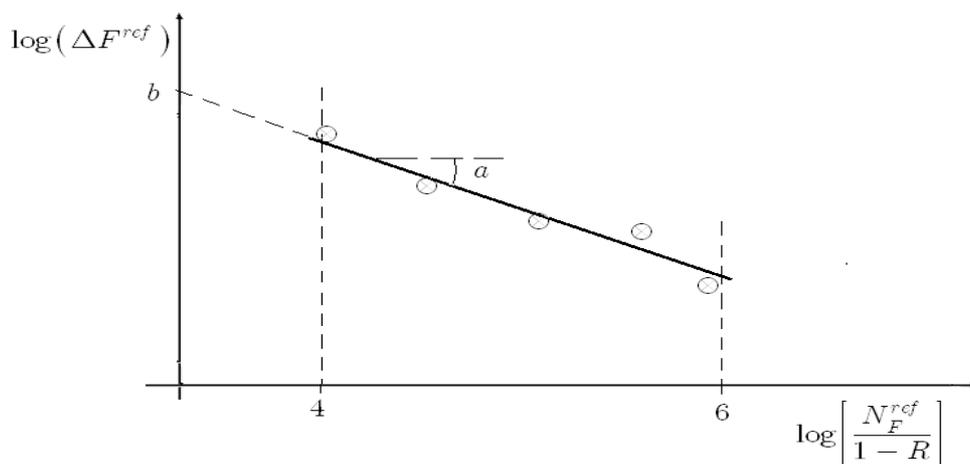
Figure 2: Experimental identification of parameters  $a, b$  using a reference joint with glued area  $A_{ref}=L_{ref}W_{ref}$
