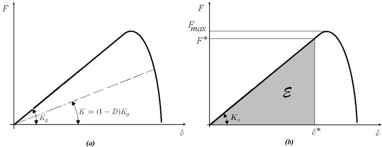
Figure 1: (a) Definition of the variable  $D$  during a tensile test. (b) Definition of the energy  $\mathcal{E}$  in a tensile test.
