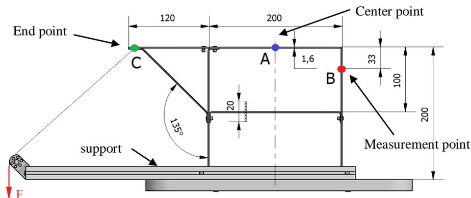
Figure 1 – Geometry of the portico structure, in mm.
