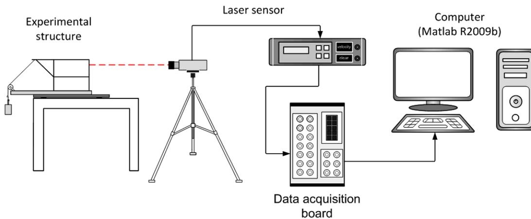
Figure 3 - Measurement system for experiment 1.
