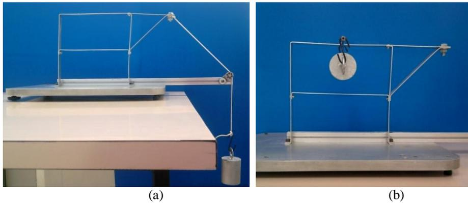
Figure 2 – Layout of experimental tests of the structure, for load at (a) point C and (b) point A.
