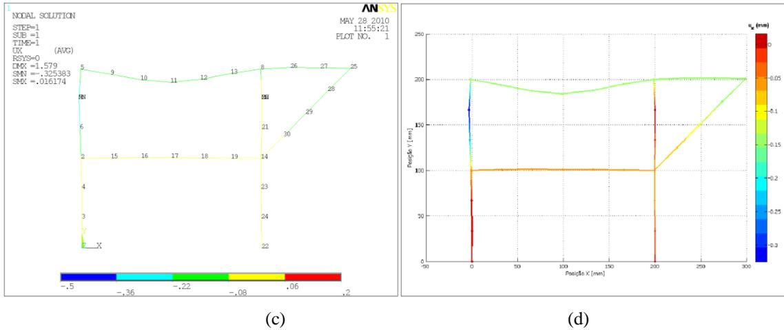
Figure 4 – Displacements, in mm, of the frame for load applied at (a),( b) point C and (c), (d) point A. Figs. (a), (c) and (b), (d) show Ansys and in-house code results, respectively.
