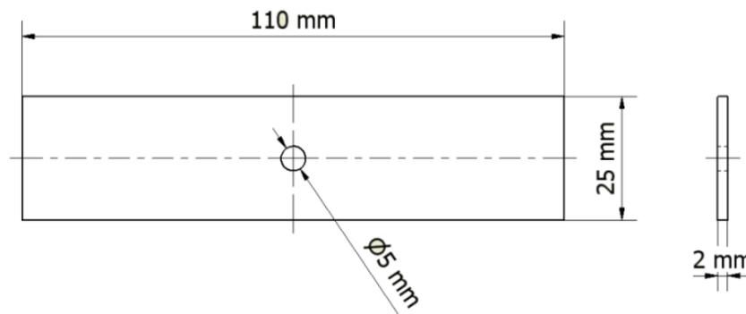
Figure 11 – Plate geometry.
