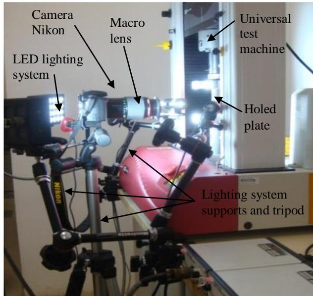
Figure 12 – Photo instrumentation and lighting system for the test.
