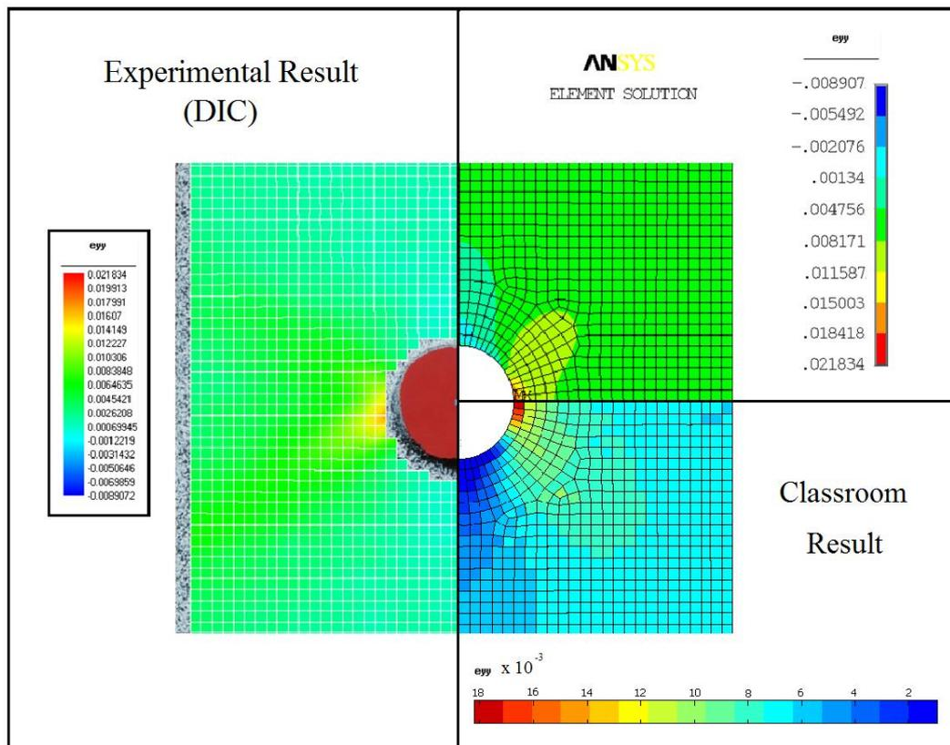
Figure 14 – Results for the strain in the y direction.
