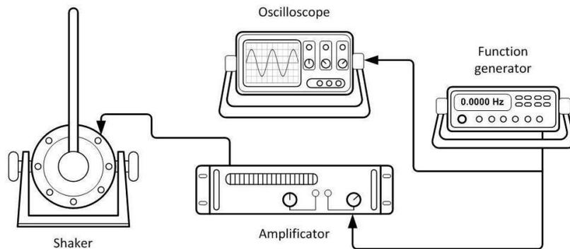
Figure 6. Measurement system for the modal analysis experiment.
