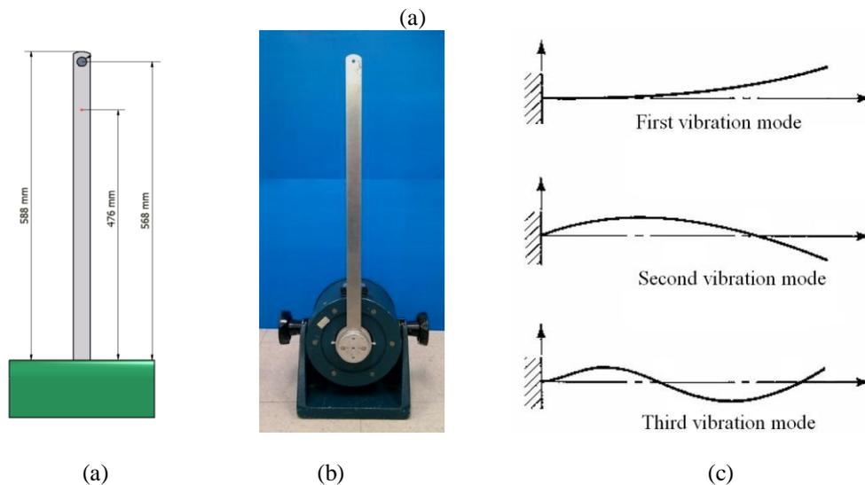
Figure 5 – Cantilever beam: (a) geometry; (b) setting of the beam on the shaker and (c) first three theoretical vibration modes.
