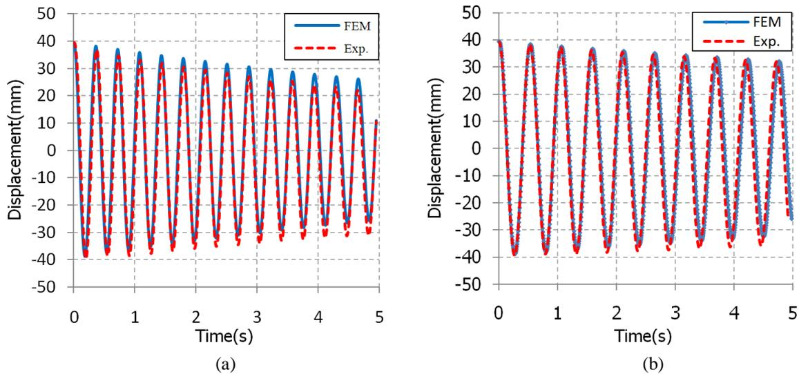
Figure 10 – Experimental and in-house FE tip displacement for the beam during free vibration, (a) without and (b) with added mass.
