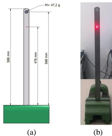
Figure 8 – Layout for the free vibration experiment.
