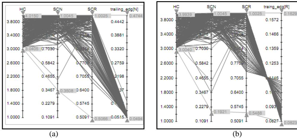
Figure 5: Variation of trailing edge loss for each blade row: (a) nozzle; (b) rotor.
