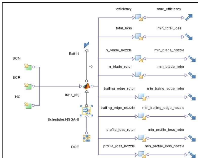
Figure 1: Schematic of the optimization process in the environment modeFRONTIER.
