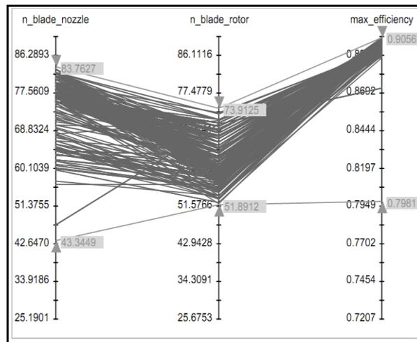
Figure 3: Influence of the choice of the number of blades in turbine efficiency.
