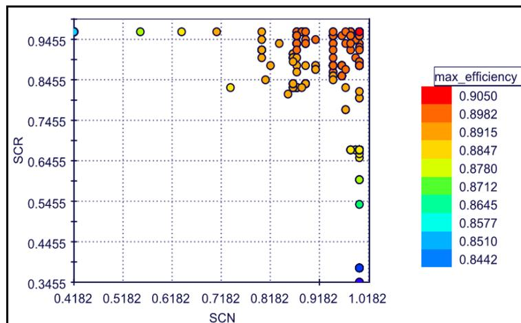
Figure 7: Front Pareto showing the various possible and viable projects based on the ratio s/c in the nozzle and rotor.
