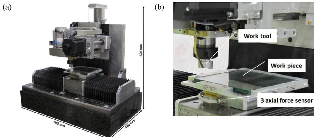
Figure 1. (a) Tribometer overview developed at TU-KL; (b) Work tool, sample holder and 3 axial sensor in detail.
