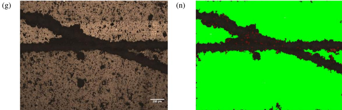
Figure 6: Optical microscopy for crossing angle (a) 22.5°; (b) 45.0°; (c) 67.5°; (d) 90.0°, (e) 112.5°; (f) 135.0°; (g) 157.5°. Image analysis recognition from (h) until (n).
