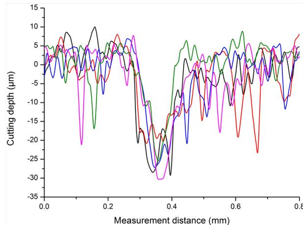
Figure 8: Optical profilometry for cutting depth.
