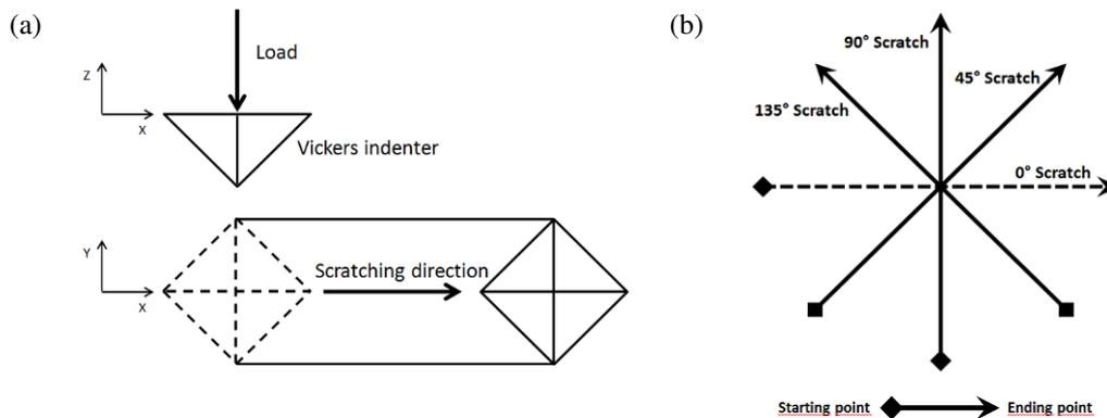
Figure 3. (a) Edge positioning for the scratch test; (b) Schematic configuration showing the scratching sequence;
