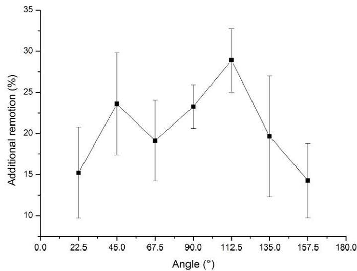
Figure 7: Additional material removal vs. scratching crossing angle.
