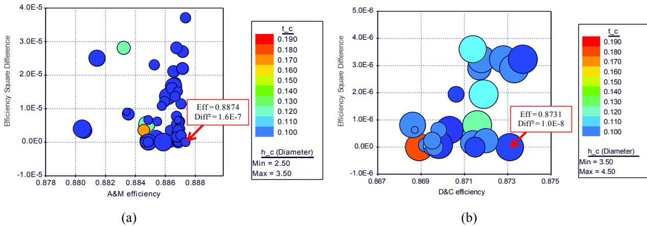
Figure 8. Optimization result highlighting optimum designs: (a) considering the efficiency of Ainley and Mathieson model and (b) Dunham and Came model.
