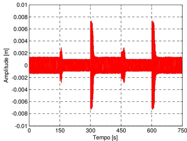
Figure 10 - Response mass displacement with system excited at frequencies 14 Hz and 17 Hz
