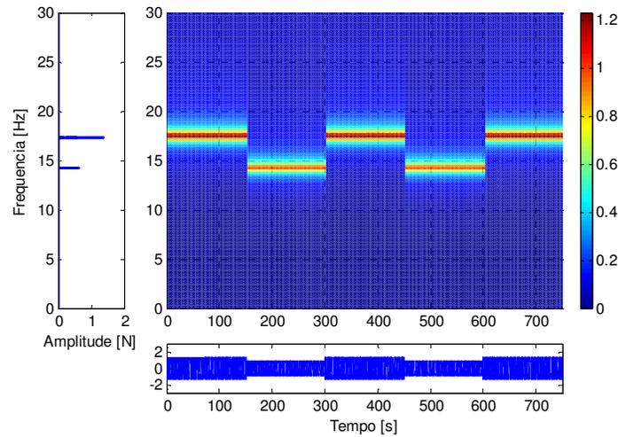
Figure 9 - Signal excitation at frequencies 14 Hz and 17 Hz.
