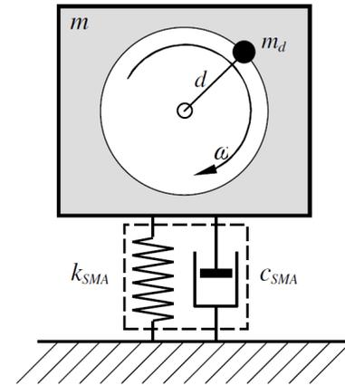
Figure 1 – Mass-spring-damper system
