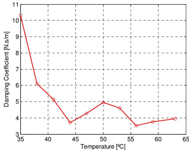
Figure 6 - Damping coefficient in function of temperature
