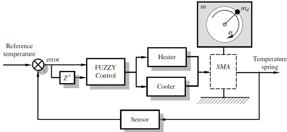
Figure 7 – Block diagram of spring temperature control
