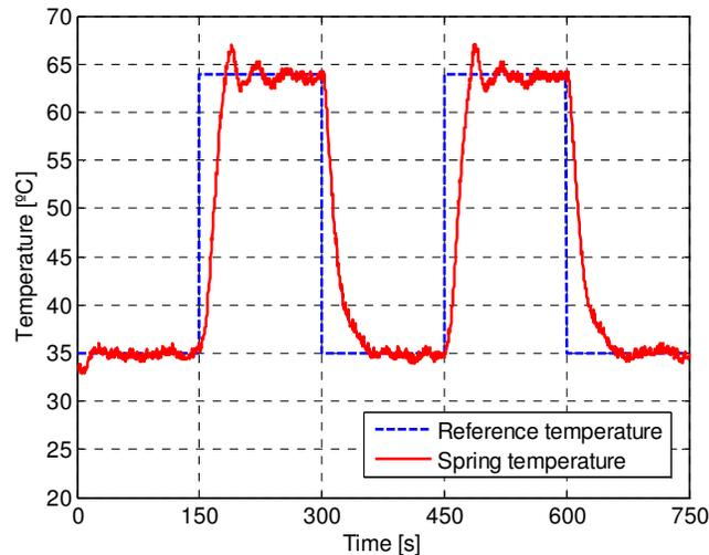
Figure 11 – Spring temperature variation with 14 Hz e 17Hz excitation
