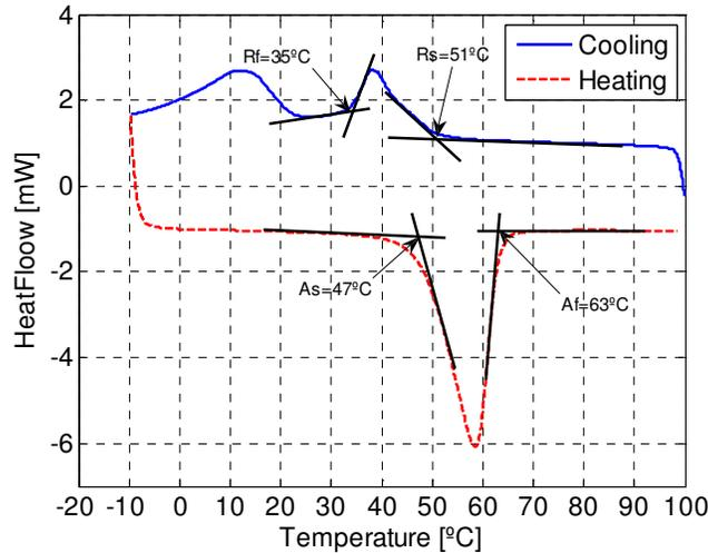
Figure 3 - Transformation temperatures obtained by DSC
