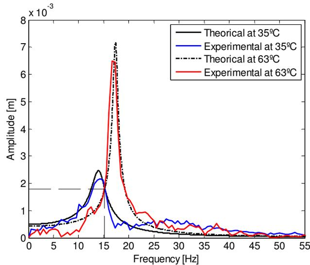
Figure 8 - Frequency Response theoretical and experimental
