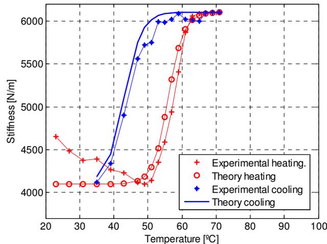
Figure 4 – Stiffness SMA spring
