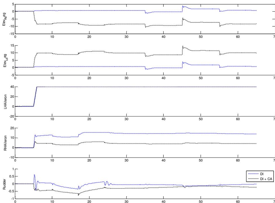
Figure 2. Surfaces position for aileron failure.
