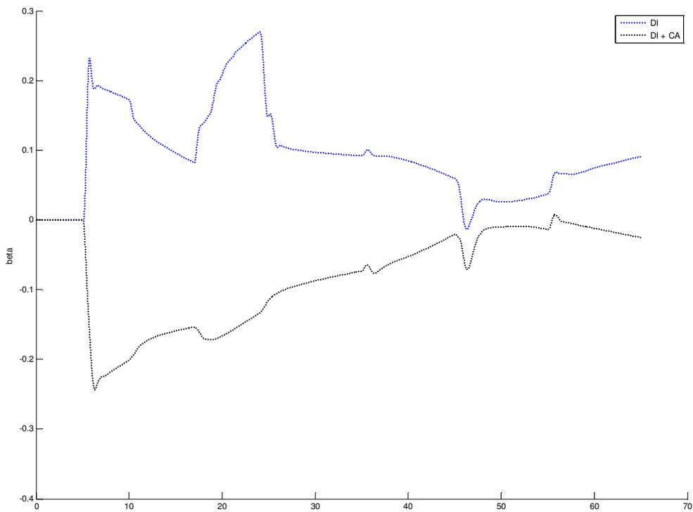
Figure 5. Drift angle for aileron failure.
