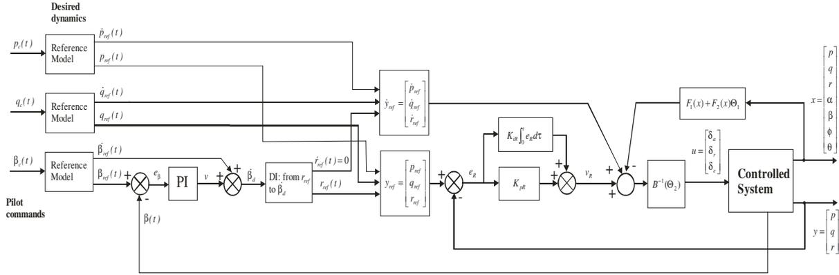
Figure 1. Baseline aircraft control system based on dynamic inversion.
