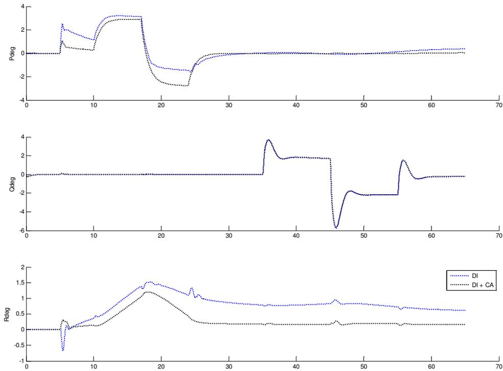
Figure 4. Angular rates for aileron failure.
