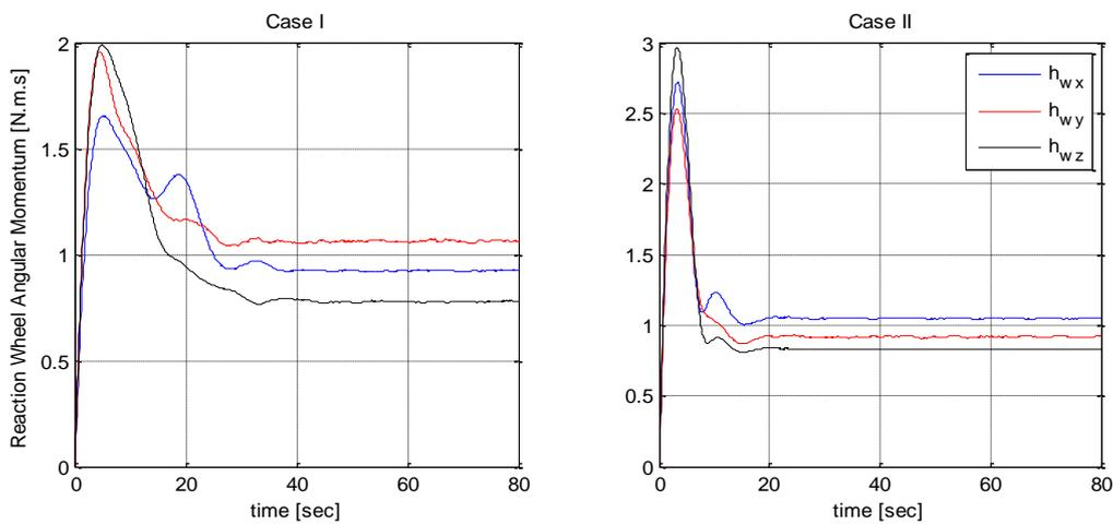
Figure 5. Angular momentum accumulated in reaction wheels (worst condition).
