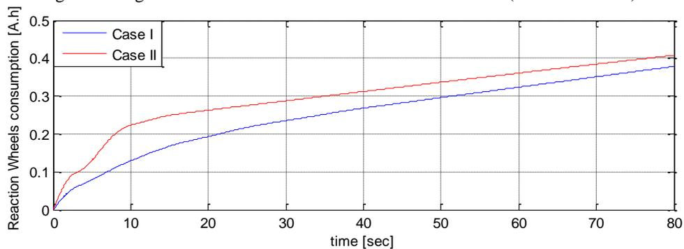
Figure 6. Reaction wheels battery charge consumption (worst condition).
