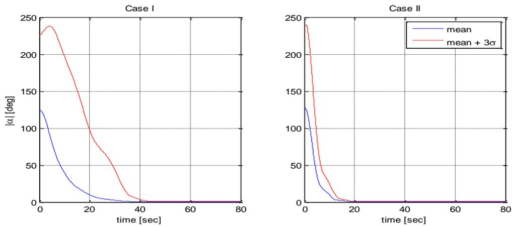
Figure 3. Euler angle evolution for combined control laws with attitude estimators.
