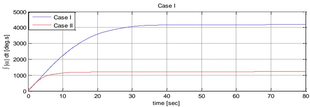
Figure 4. Integral of error angle  $|\alpha|$  about the Euler axis of rotation (worst condition).
