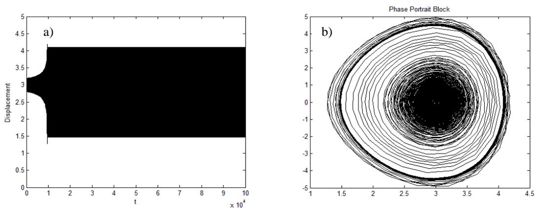
Figure 6: initial position  $[4.5, 0, 0, 0]$  in jump a) displacement  $\mu_1 = 3.2$  b) phase portrait  $\mu_1 = 3.2$
