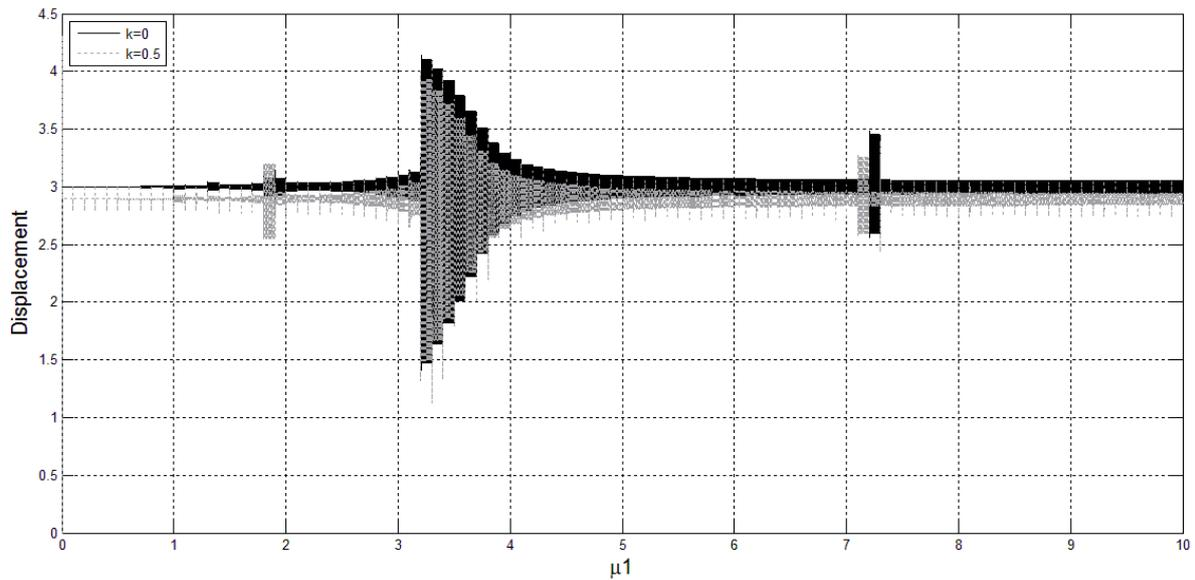
Figure 9: the comparative system with the spring (gray) and without spring (black)
