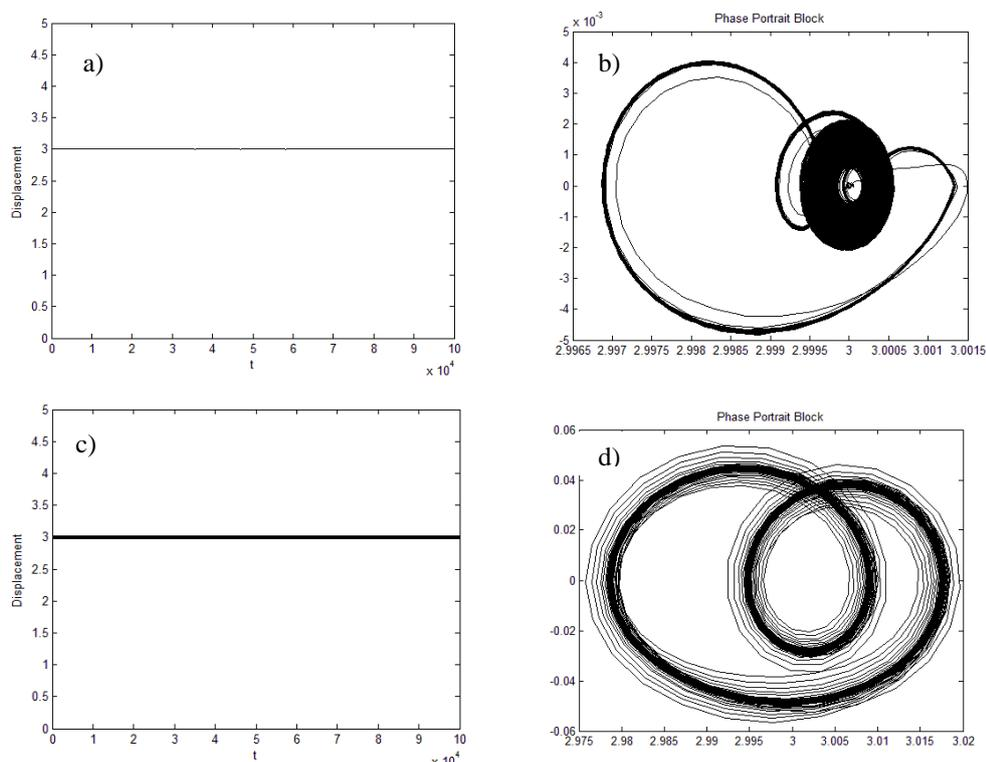
Figure 4: initial position  $[4.5, 0, 0, 0]$  before jump a) displacement  $\mu_1 = 0.5$  b) phase portrait  $\mu_1 = 0.5$  c) displacement  $\mu_1 = 1.6$  d) phase portrait  $\mu_1 = 1.6$
