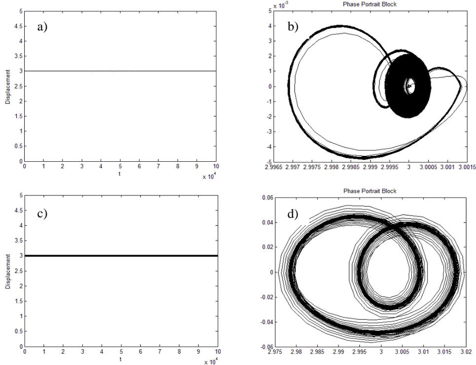
Figure 3: Initial position  $[0, 0, 0, 0]$  before jump a) displacement  $\mu_1 = 0.5$  b) phase portrait  $\mu_1 = 0.5$  c) displacement  $\mu_1 = 1.6$  d) phase portrait  $\mu_1 = 1.6$ .
