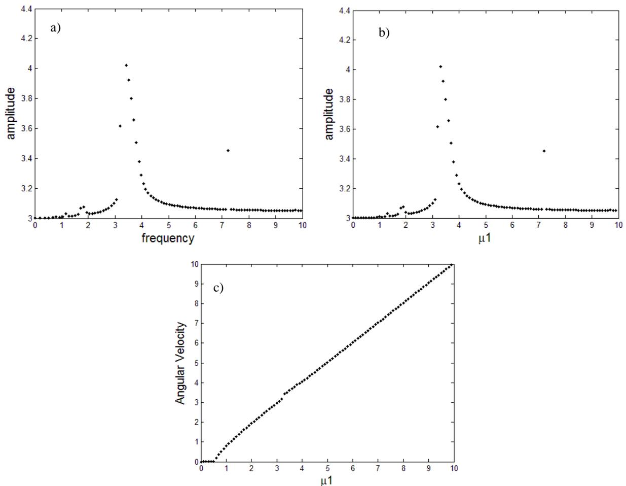
Figure 2 – Sommerfeld Effect a) amplitude vs. frequency means b) amplitude vs. tension ( $\mu_1$ ) c) angular velocity vs tension ( $\mu_1$ )
