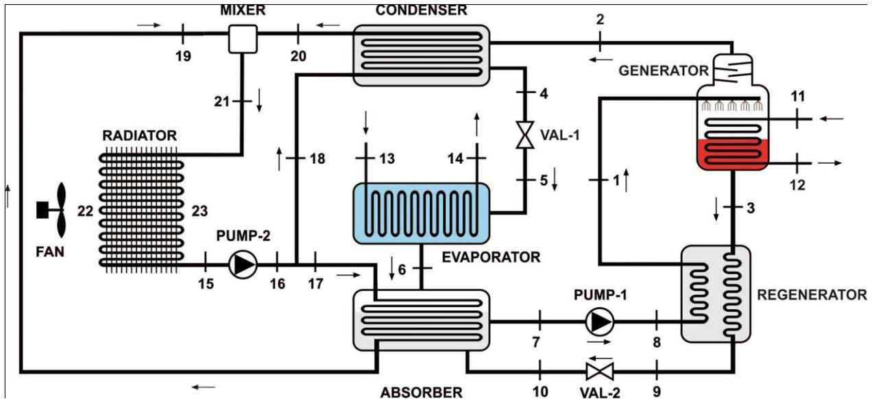
Figure 2. AAR basic schematic with regenerator coupled to external circuit (radiator, pump-2 and mixer).
