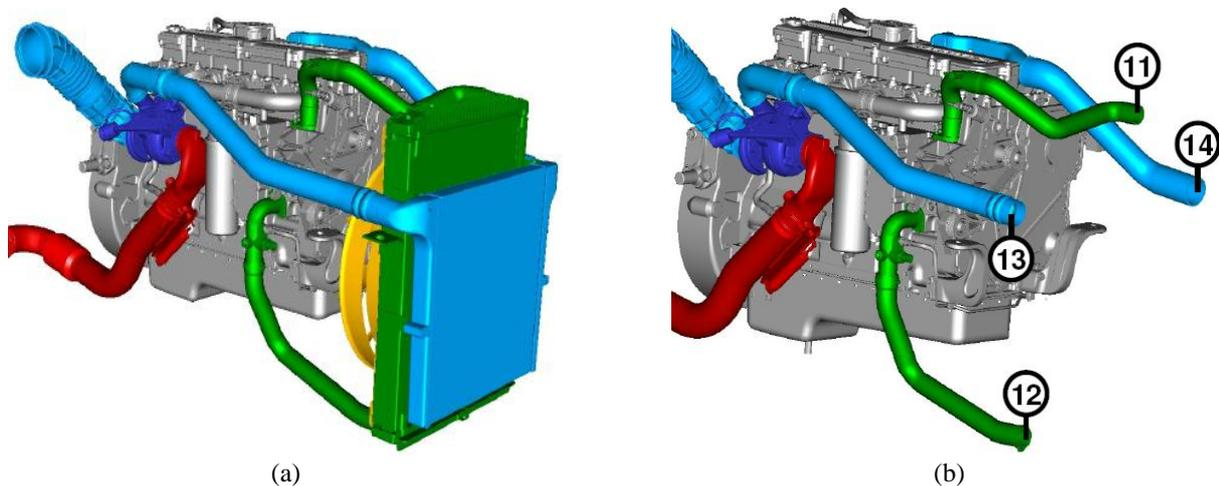
Figure 1. Schematic (a) turbo engine coupled to standard cooling package (b) turbo engine uncoupled.
