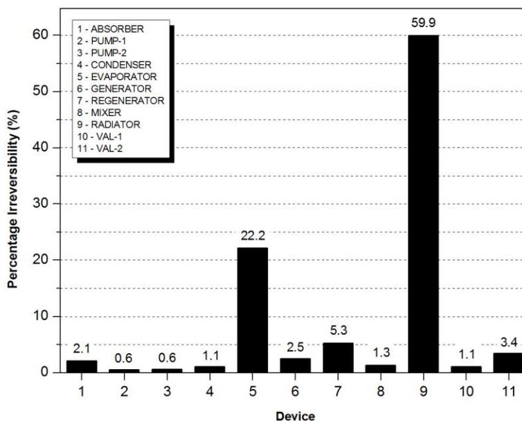
Figure 3. Percentage irreversibility of each device of the cycle according to results from table 5.
