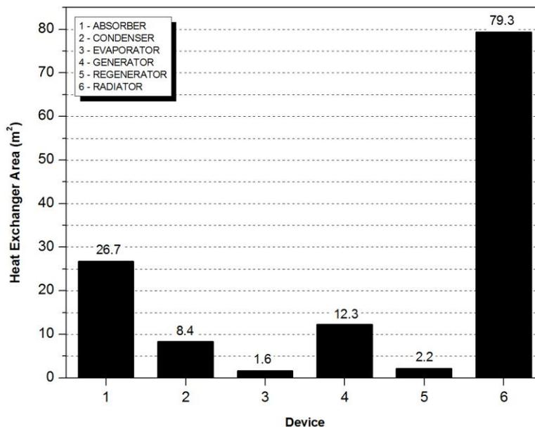
Figure 4. Heat exchanger area of devices according to equation 12 and table 2.
