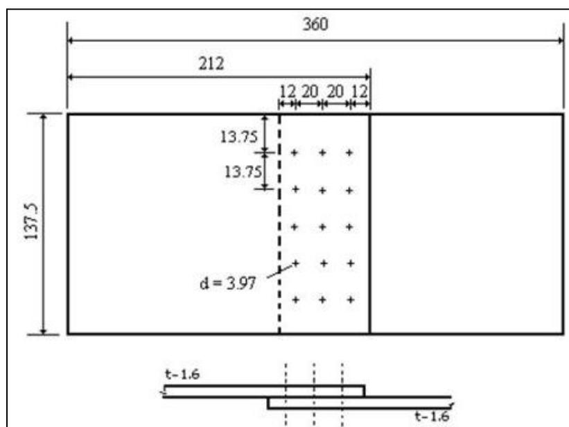
Figure 1. Specimen's dimensions [mm]
