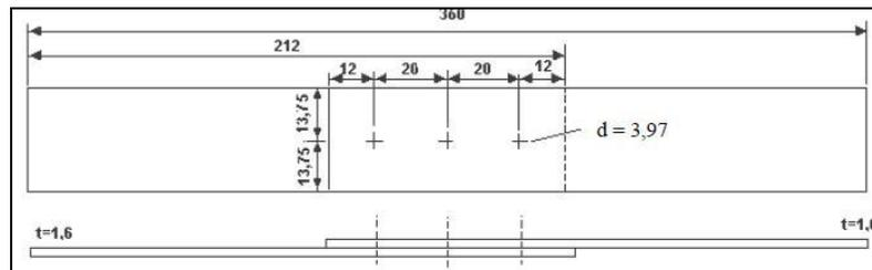
Figure 4. Dimensions of the solid riveted joint’s model [mm]
