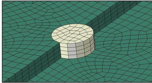
Figure 7. Compatible mesh between the part instances
