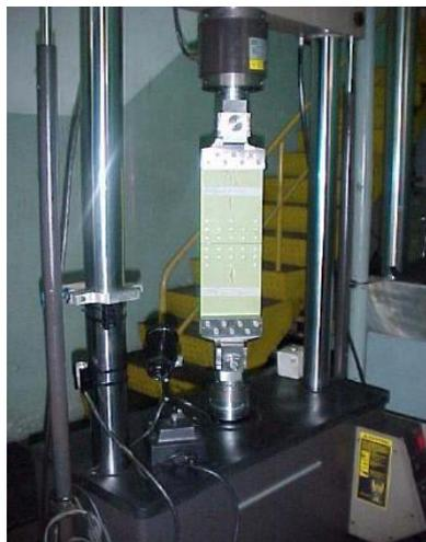
Figure 2. Universal machine MTS 25”
