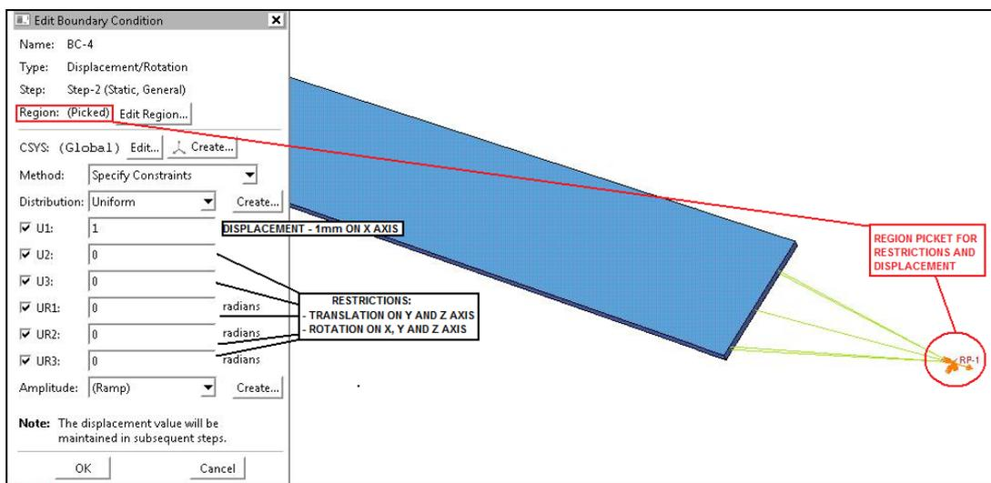
Figura 13. BC Step2: Ending displacement
