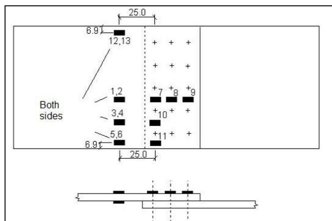
Figure 3. Strain-gauges distribution
