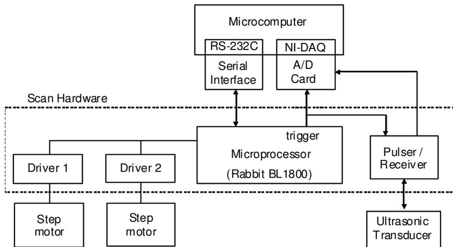
Figure 2. Block diagram of the automatic inspection equipment.
