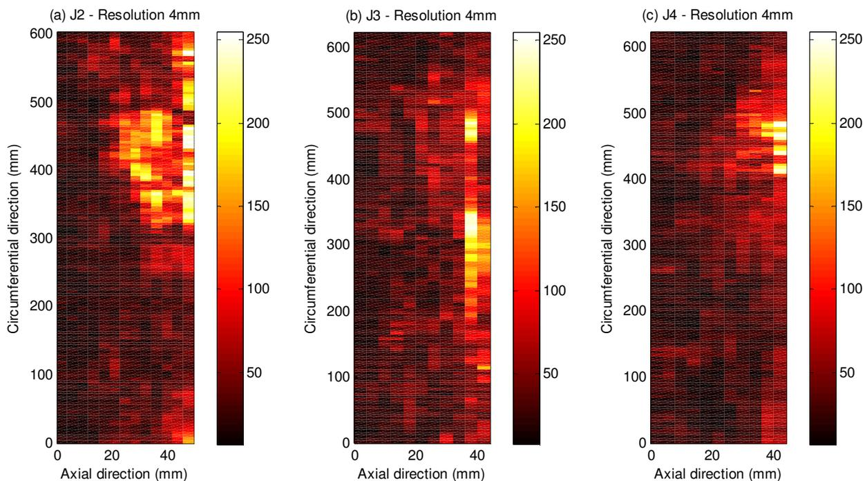
Figure 9. C-scan images obtained from joints (a) J2, (b) J3, and (c) J4 at 4-mm spatial resolution, using the 2-MHz transducer.
