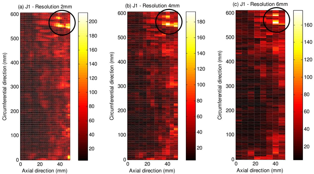
Figure 8. Comparison of the C-scan images from joint J1 obtained using the 2-MHz transducer for three different spatial resolutions: (a) 2 mm, (b) 4 mm, and (c) 6 mm.
