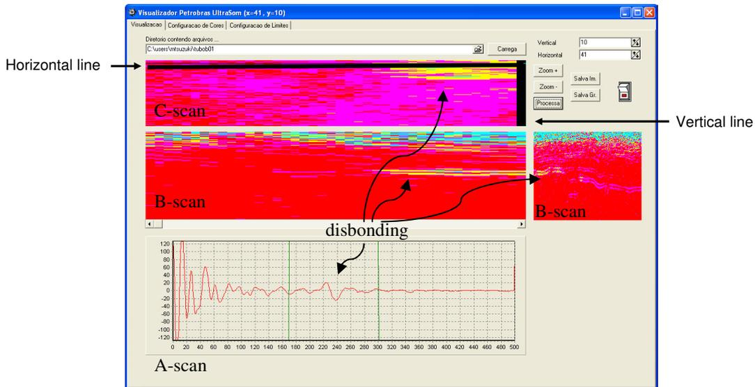
Figure 6. Scanning display software window.
