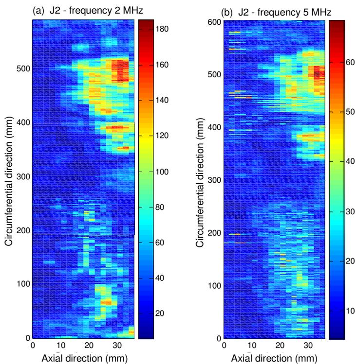
Figure 10. Comparison of the C-scan images from joint J2 at 2-mm spatial resolution obtained for two frequencies: (a) 2 MHz, and (b) 5 MHz.
