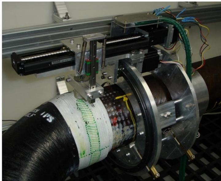
Figure 1. Mechanical parts of the automatic ultrasonic inspection system embracing the pipe.
