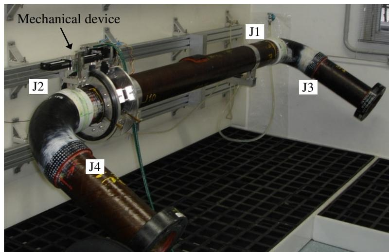
Figure 7. Experimental configuration (mechanical device attached to the composite tube with 4 joints)
