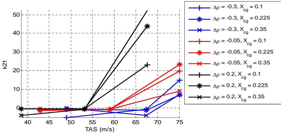
Figure 6. Proportional gain of PID2.
