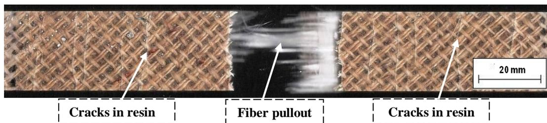
Figure 4: Final fracture region of a **CHN** test specimen.
