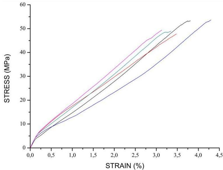
Figure 7: Stress x Strain diagram obtained for **CH7.5** test specimens.
