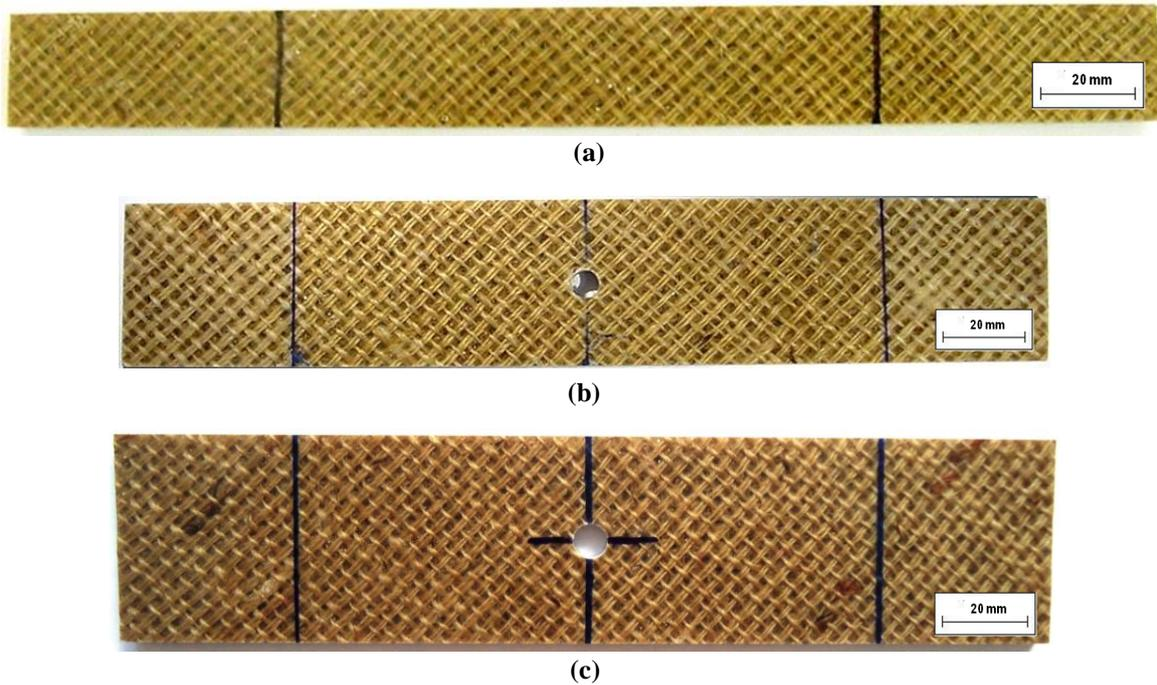
Figure 2: Test specimens used in the tests: (a) CHN; (b) CH6; (c) CH7.5.
