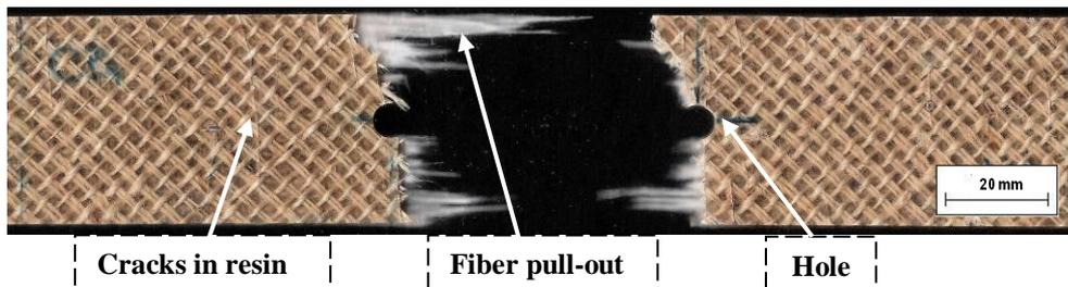
Figure 6: Final fracture region of a **CH6** test specimen.
