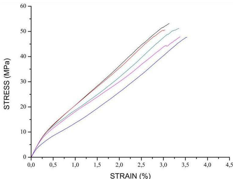
Figure 5: Stress x Strain diagram in uniaxial tensile testing - **CH6** test specimens.
