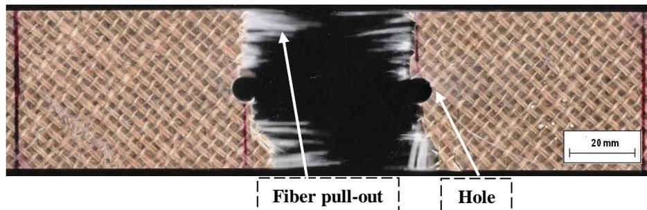
Figure 8: Final fracture region of a **CH7.5** test specimen.
