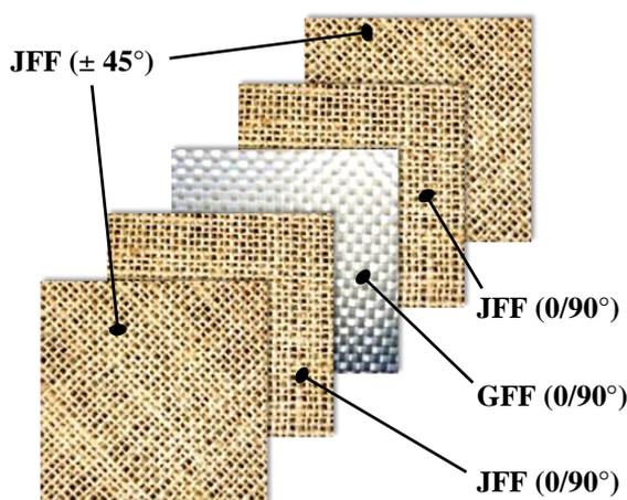
Figure 1: Configuration of Hybrid Composite Laminate - **CH**.
