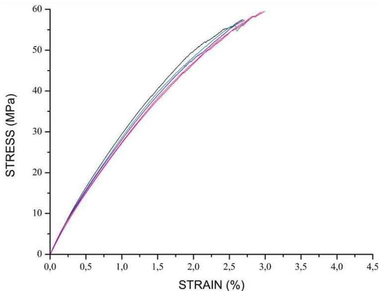
Figure 3: Stress x strain diagram in uniaxial tensile test – **CHN** test specimens.
